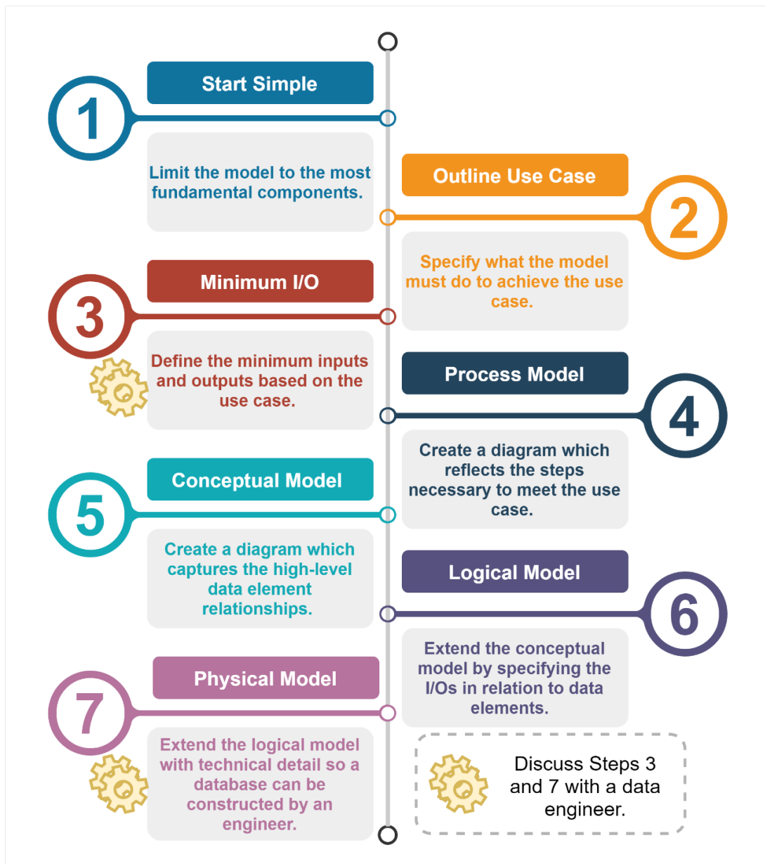
Figure 4 – Data Modelling Workflow. Suggested steps required to build and understand a data model, demonstrated through the worked example in Section 4.2. Documentation is necessary at all stages, and so is not explicitly connected to the other notes. Data Engineer Involvement is an optional node connected to steps three and seven. The figure layout is based off a DrawIO template which was customized for this document.
