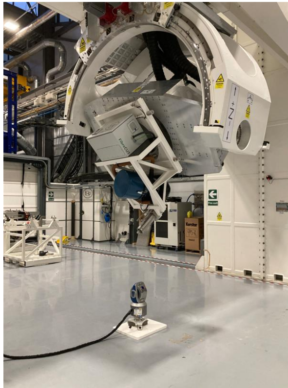
Figure 12 USK end-effector TCP was measured using a laser tracker
