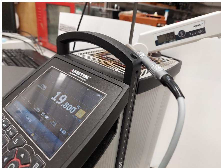
Figure 1 Calibration set-up for the EBRO sensor
