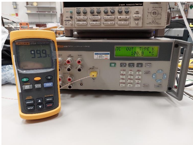
Figure 2 Calibration setup for the Fluke sensor
