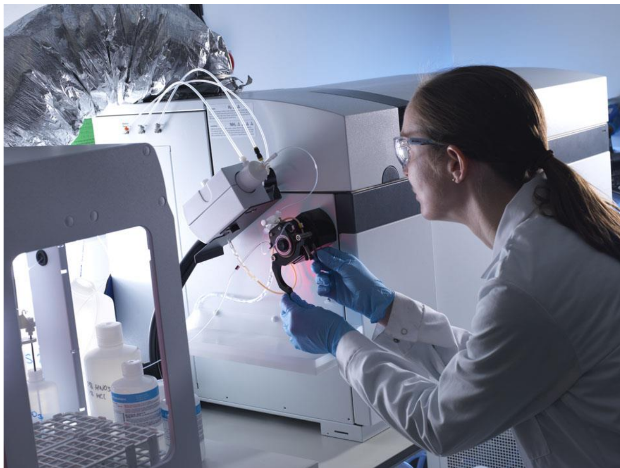
Image 3 Agilent 8800 ICP-QQQ-MS in the UK ambient metals analysis facility at NPL.
