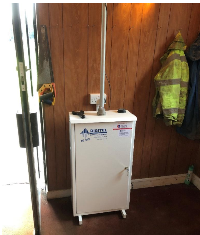
Image 1 The newly installed Digitel DPA14 sampler at the network monitoring site at Swansea Coedgwilym.
