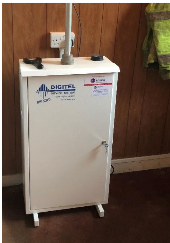
Image 1 The Digitel DPA14 sampler at the network monitoring site at Swansea Coedgwilym.
