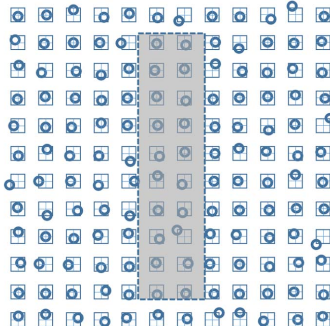
Figure 3. Simplified simulation of random offsets of the spot positions. The small squares are the nominal (planned) spot positions spaced 2.5 mm in both scan directions. The circles are the spot positions with a random offset distributed rectangulary in both directions with a half-width of 0.3 mm. The grey shaded area is the projected area perpendicular to the beam direction of a Farmer type ionization chamber with a diameter of 6 mm and a length of 24 mm. The circular lateral profile of a single spot was assumed to be Gaussian with a FWHM of 8 mm and the contribution to dose was integrated over the shaded area, both for the nominal spot positions and the randomized positions. In reality, the field simulated is much larger (200 mm \times 200 mm) in order to ensure lateral secondary proton equilibrium.
