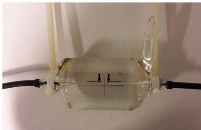
Figure 1. The glass detection vessel with the thermistor probes (indicated by arrows) aligned at the centre.
