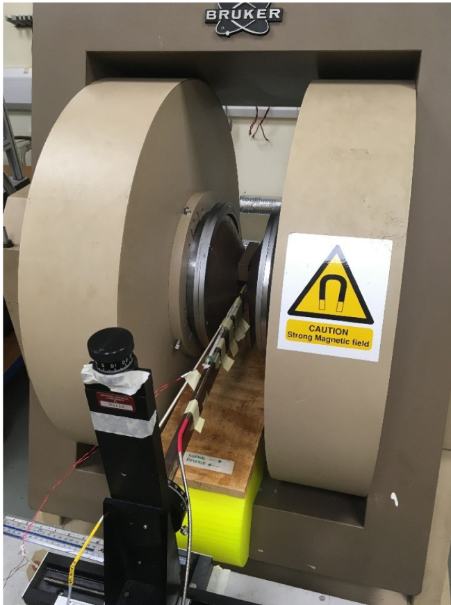
Figure 13. The three probes—NPL phosphor, thermocouple and resistance—mounted between the poles of the Bruker electromagnet.
