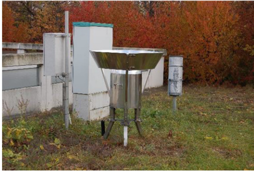
Figure 3. Weighing gauge installed in field.
