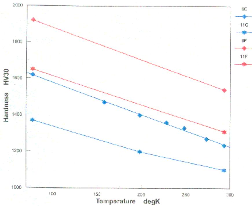
Figure 1: Variation of hardness with temperature for tests on 6F, 11F, 6C and 11C with Vickers indenter.
