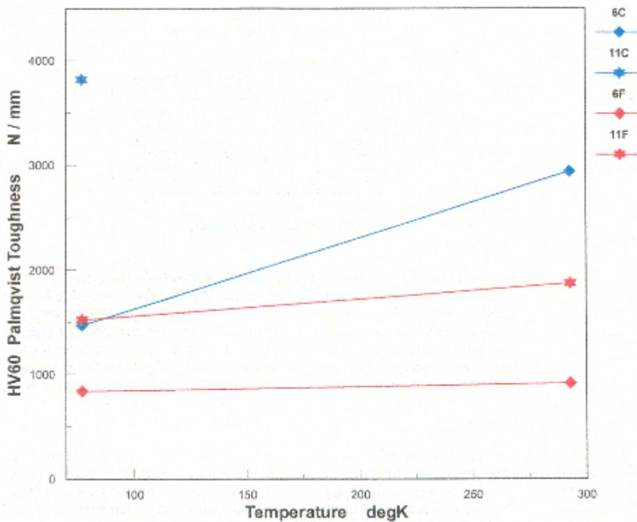
Figure 2: Variation of Palmqvist toughness with temperature.
