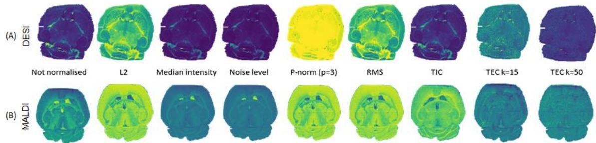
Figure 4. Published normalisation methods and TEC normalisation applied to (A, top) DESI and (B, bottom) MALDI MSI of sublimed Olanzapine on mouse brain. Normalisation methods (left-to-right): Not normalised, L2 normalisation, median intensity normalisation, noise level normalisation, P-norm normalisation ( $p=3$ ), root mean square (RMS) normalisation, total ion count (TIC) normalisation and TEC normalisation ( $k=15$  and  $k=50$ ).
