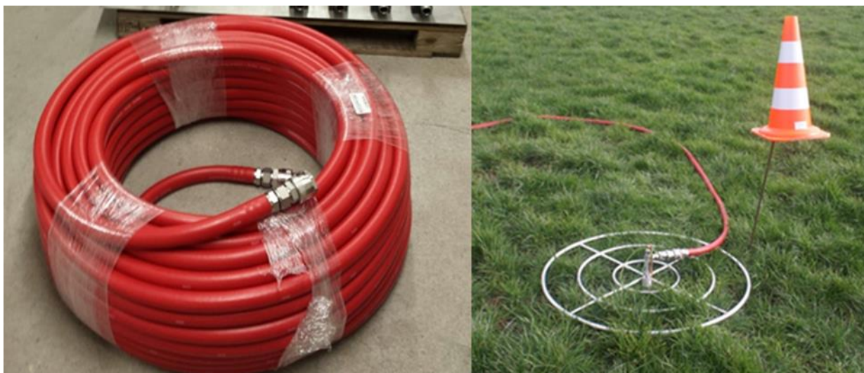
Figure A2.3 Pictures of the distribution hose (left) and emission node (right).
