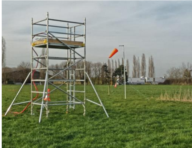
Figure A2.1 The ASF deployed in a tower release configuration.
