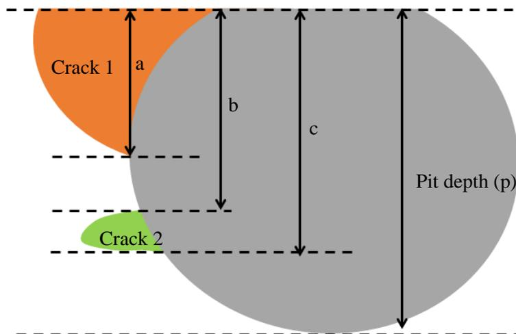
**Figure 3:** Schematic diagram illustrating the ratio of crack depth range to pit depth.
