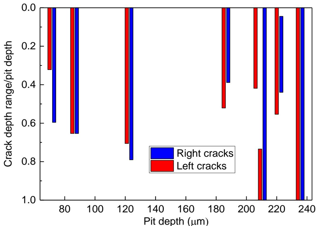
**Figure 4:** Ratio of crack depth range to pit depth versus pit depth (mean value from sectioning) for “dominant” cracks associated with pits with depths varying from 70  $\mu\text{m}$  to 240  $\mu\text{m}$ .
