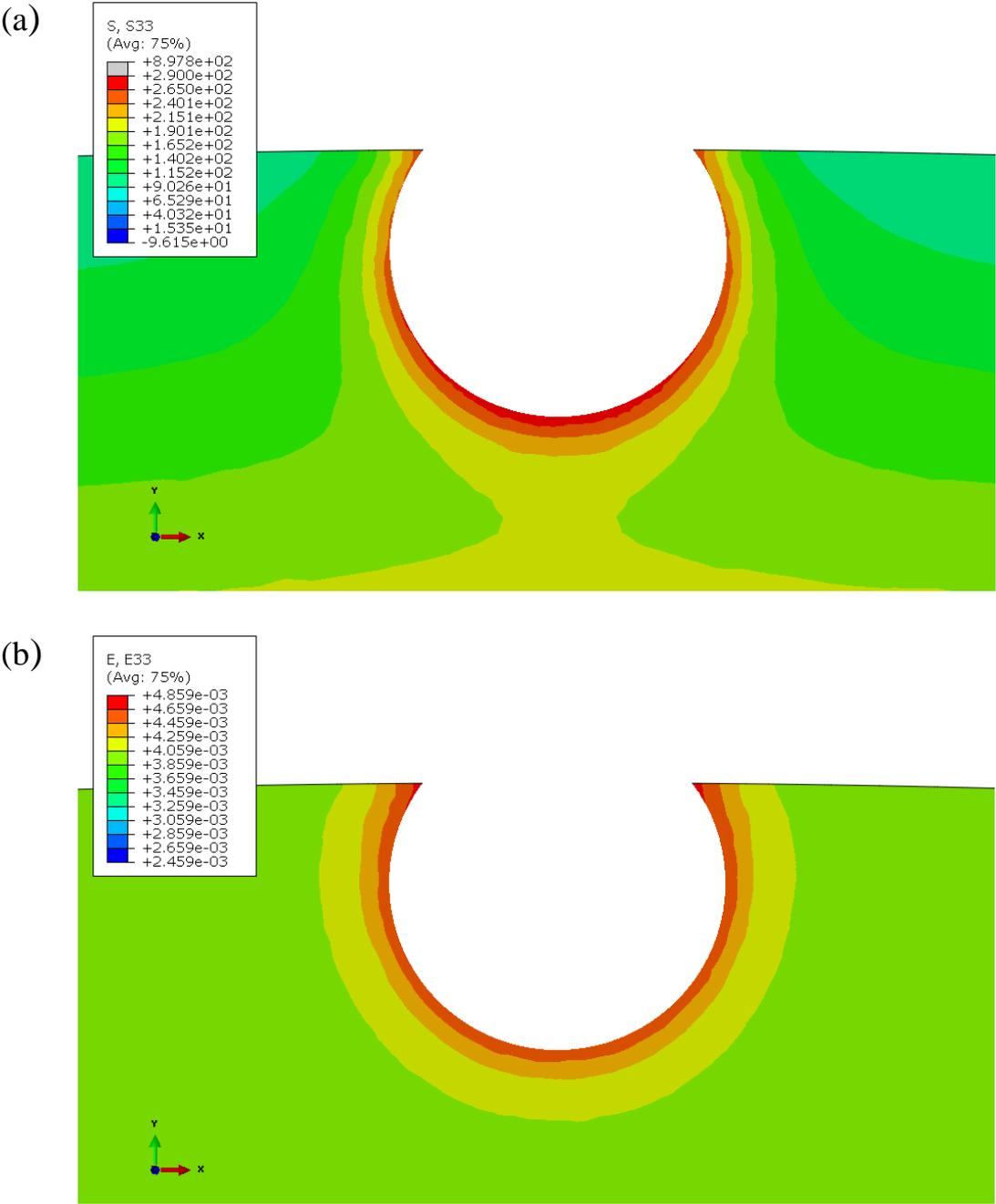
**Figure 8:** Cross-Section view of stress (a) and strain (b) around 50  $\mu\text{m}$  deep pit calculated with longitudinal (z-direction) residual compressive stress (profile shown in Figure 7) and 663 MPa applied tensile stress.
