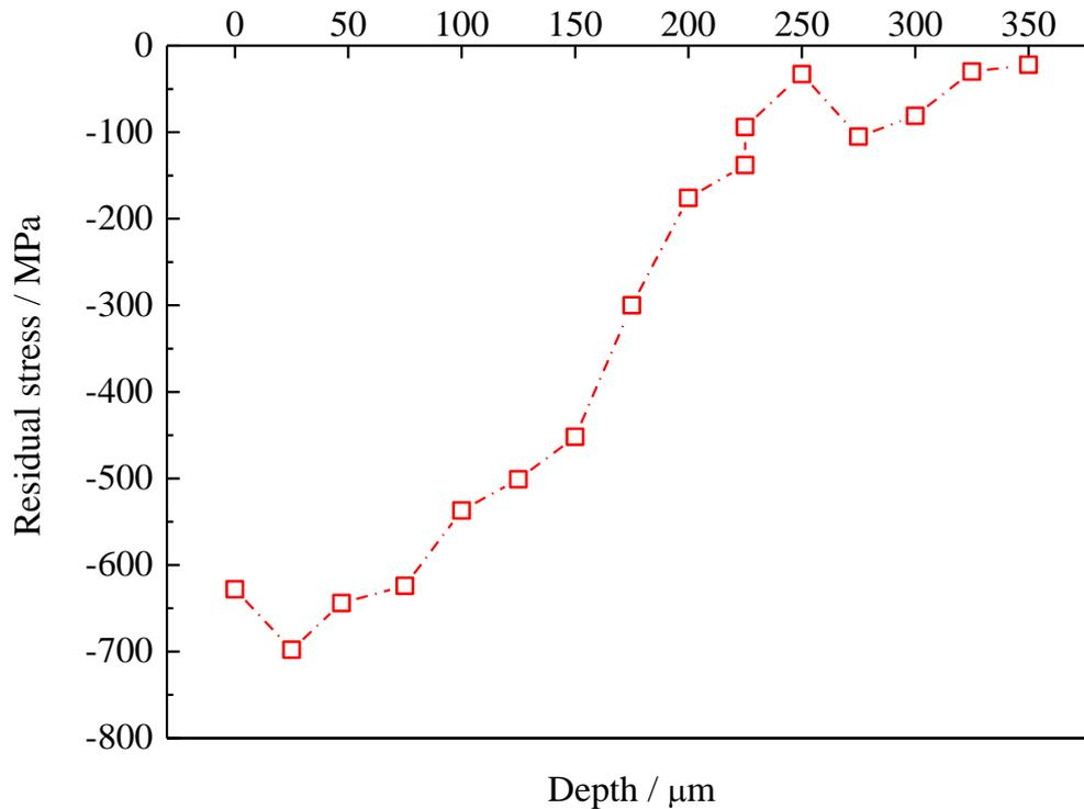
**Figure 7:** Longitudinal residual stress profile determined by X-ray diffraction.
