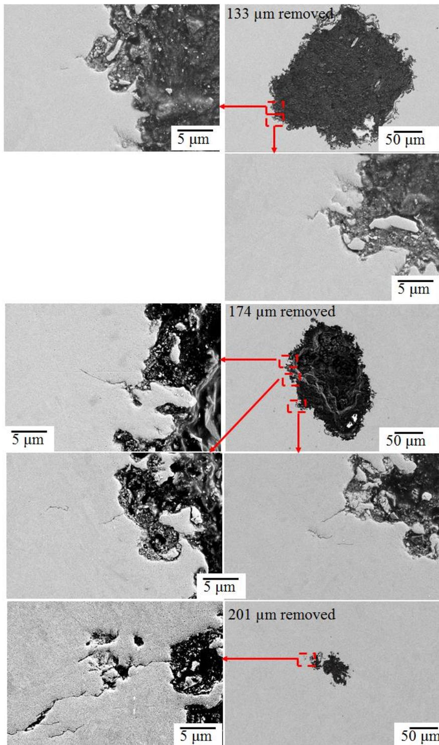
**Figure 6:** SEM images of a pit of 209  $\mu\text{m}$  depth and the corresponding cracks after serial sectioning.
