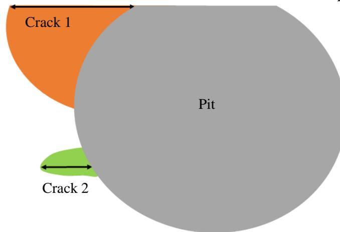
**Figure 2:** Schematic diagram illustrating the definition of the “dominant” crack with the arrows representing the maximum length of each crack.
