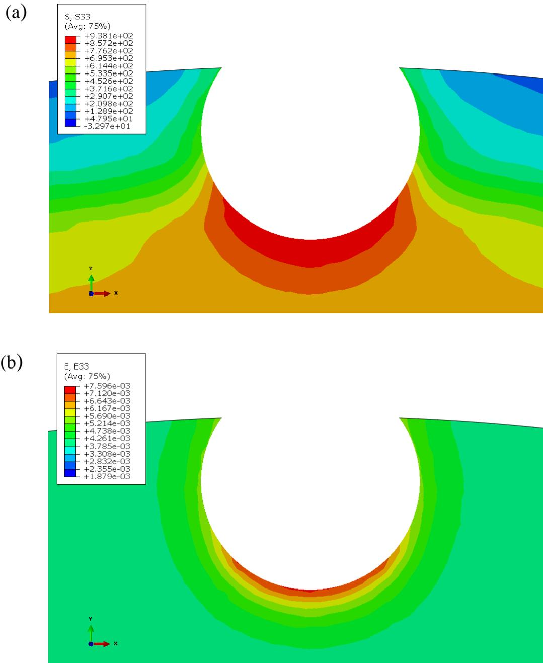
**Figure 10:** Cross-Section view of stress (a) and strain (b) around 250  $\mu\text{m}$  deep pit calculated with longitudinal (z-direction) residual compressive stress (profile shown in Figure 7) and 663 MPa applied tensile stress.
