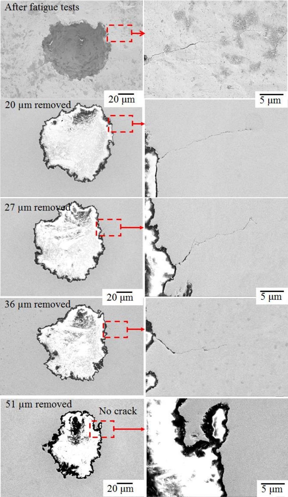
**Figure 5:** SEM images of a pit of 74 μm depth and a crack observed after fatigue tests and following serial sectioning steps.
