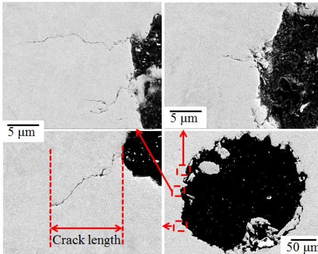
**Figure 1:** SEM images of a pit of 209  $\mu\text{m}$  depth and the corresponding cracks with a layer removal of 51  $\mu\text{m}$ .
