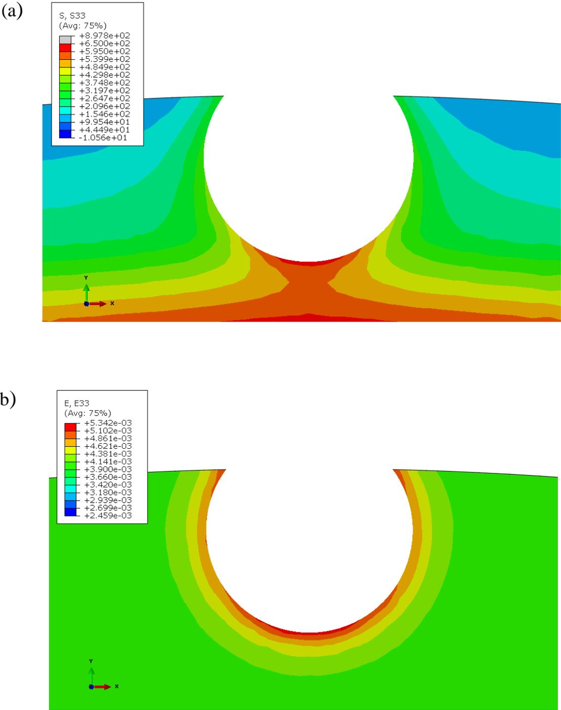
**Figure 9:** Cross-Section view of stress (a) and strain (b) around 150 µm deep pit calculated with longitudinal (z-direction) residual compressive stress (profile shown in Figure 7) and 663 MPa applied tensile stress.
