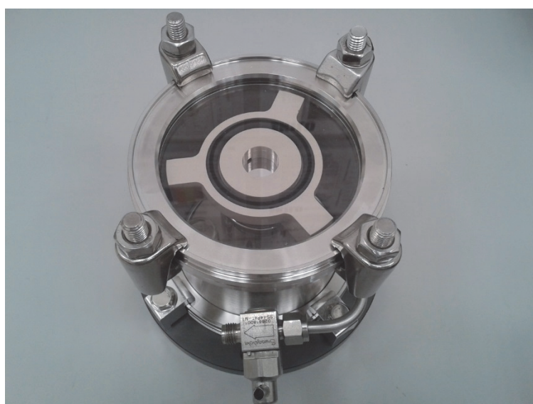
Figure 2. Stainless steel kilogram in an inert gas / vacuum compatible transfer vessel.
