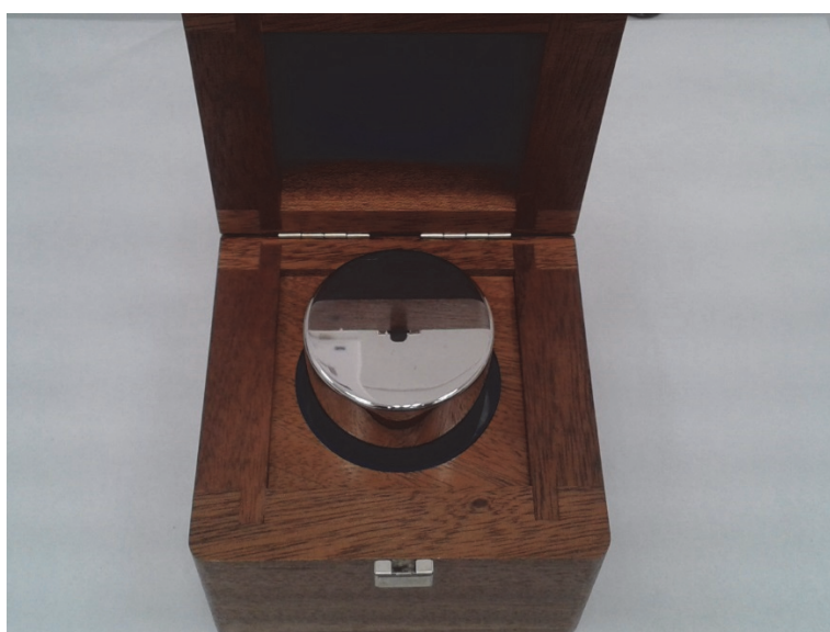
Figure 1. Stainless steel kilogram transfer standard in a conventional wooden transfer box.
