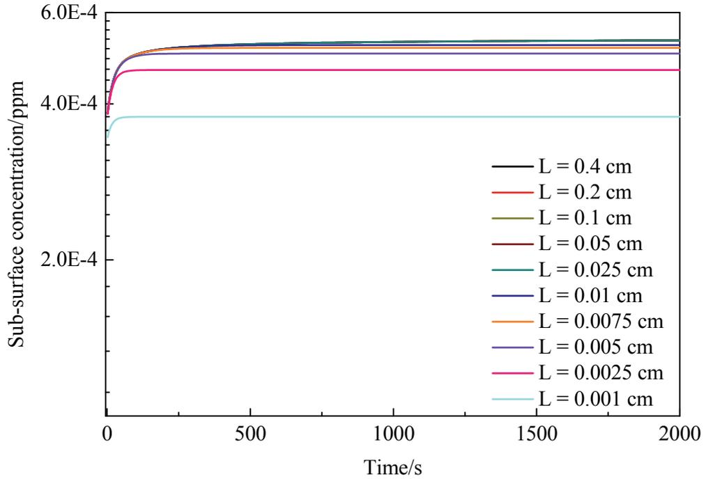
**Figure 2:** Calculated variation of the sub-surface concentration of hydrogen atoms as a function of time and specimen thickness; charging current density of  $48 \mu\text{A}/\text{cm}^2$ .
