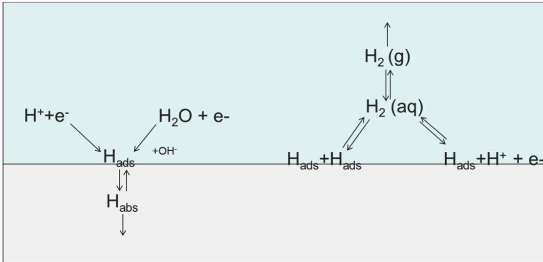
**Figure 1:** Schematic illustration of reaction processes at charging surface.
