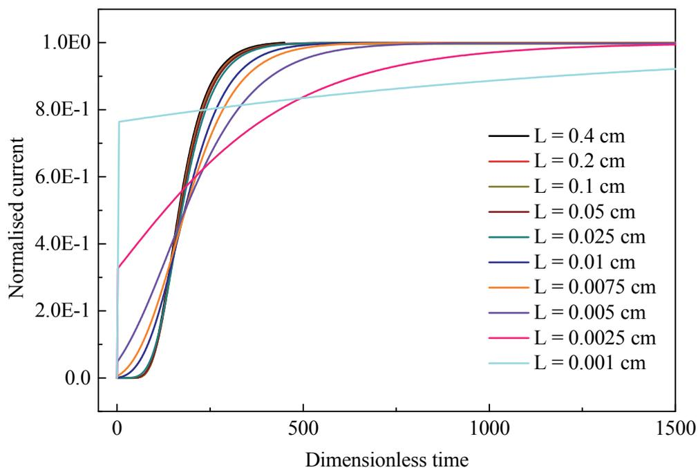
**Figure 4:** Normalised permeation current density at oxidation surface as a function of dimensionless time and thickness for charging current density of  $48 \mu\text{A}/\text{cm}^2$ .
