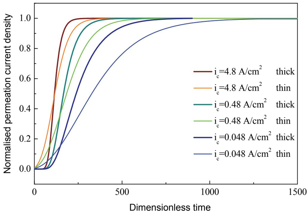
**Figure 5:** Effect of charging current density on normalised permeation flux vs dimensionless time for a thick specimen (0.4 cm) and for a relatively thin specimen (0.0075 cm).
