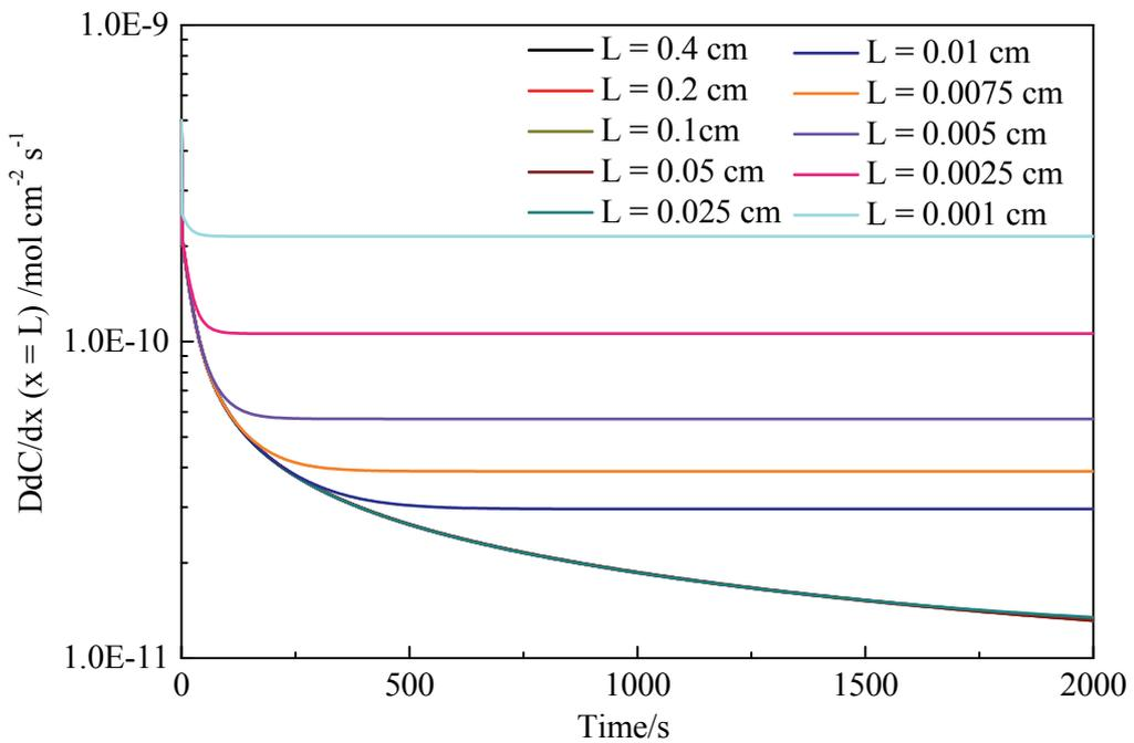
**Figure 3:** Calculated flux at charging surface as a function of thickness and time for charging current density of  $48 \mu\text{A}/\text{cm}^2$ .
