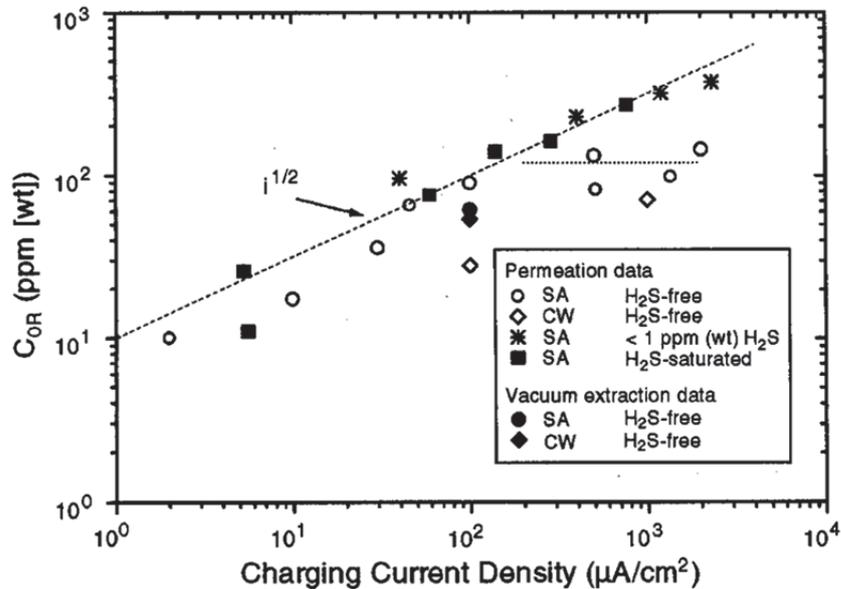
**Figure 6:** Experimental determined values of the total sub-surface concentration of lattice and reversibly trapped hydrogen atoms at steady state for duplex stainless steel in simulated oilfield environments at 80 °C [16].
