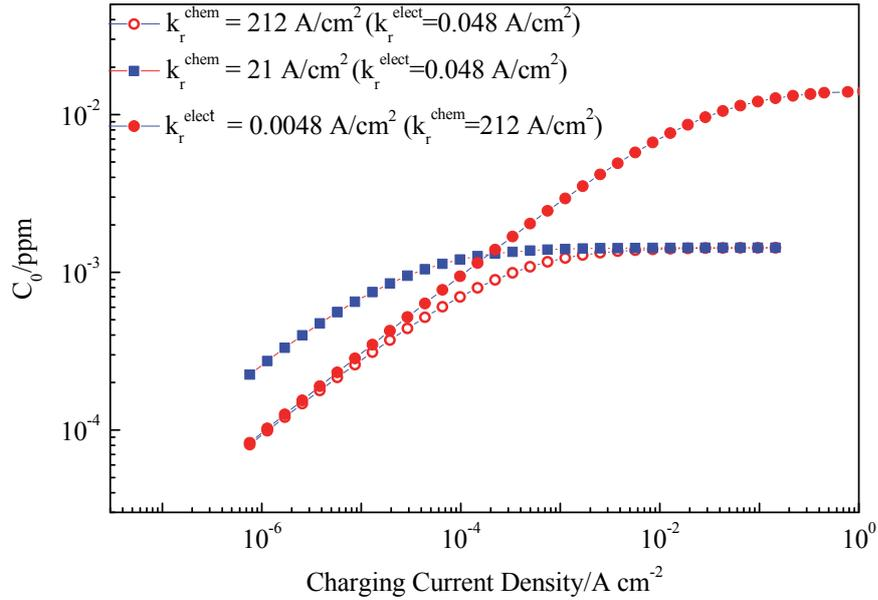
**Figure 7:** The sub-surface lattice concentration of hydrogen as a function of charging current density demonstrating the limiting value as electrochemical recombination becomes dominant and the decrease in magnitude with increase in chemical recombination rate constant.
