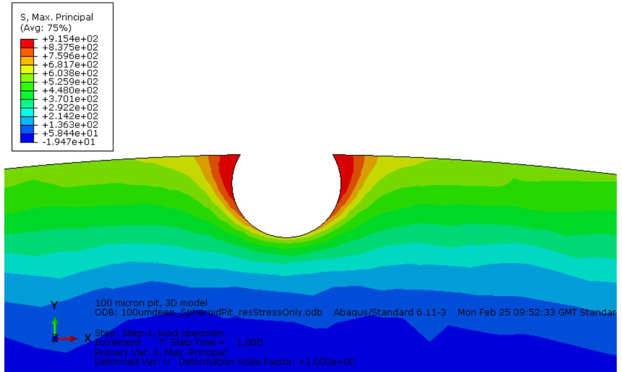
**Figure 6:** Maximum principal stress, cross-section view.
