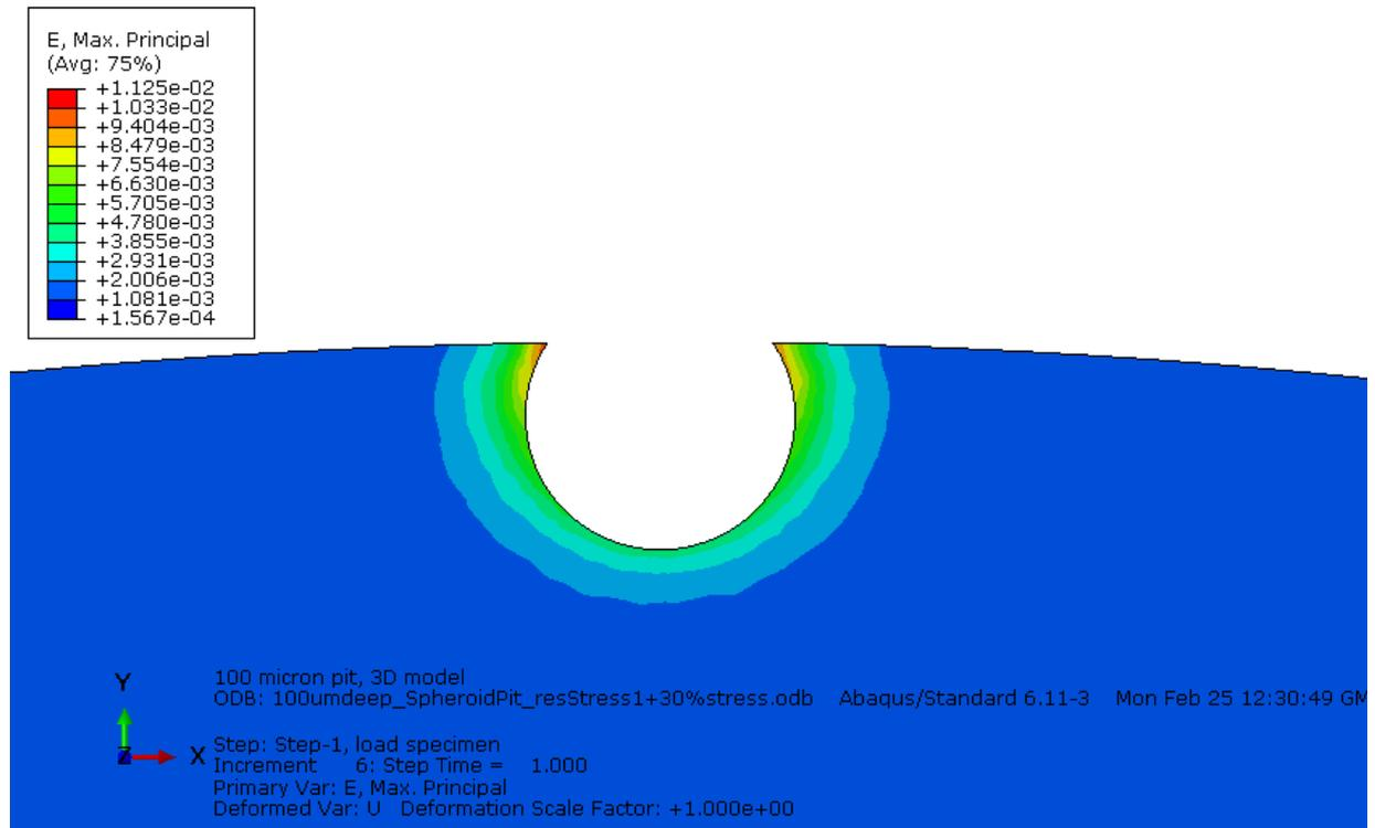
**Figure 10:** Maximum principal strain, cross section view, with applied stress of 30%  $\sigma_{0.2}$  superimposed on residual stress.
