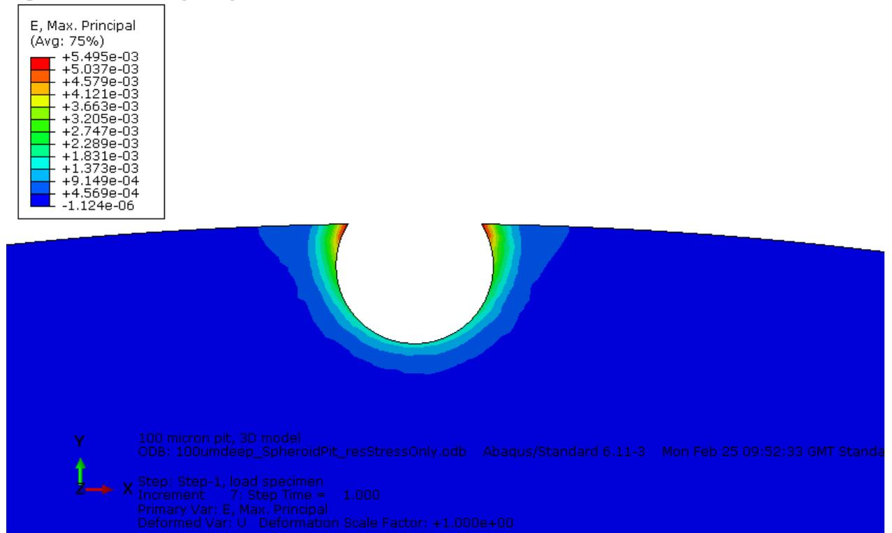
**Figure 7:** Maximum principal strain, cross-section view.
