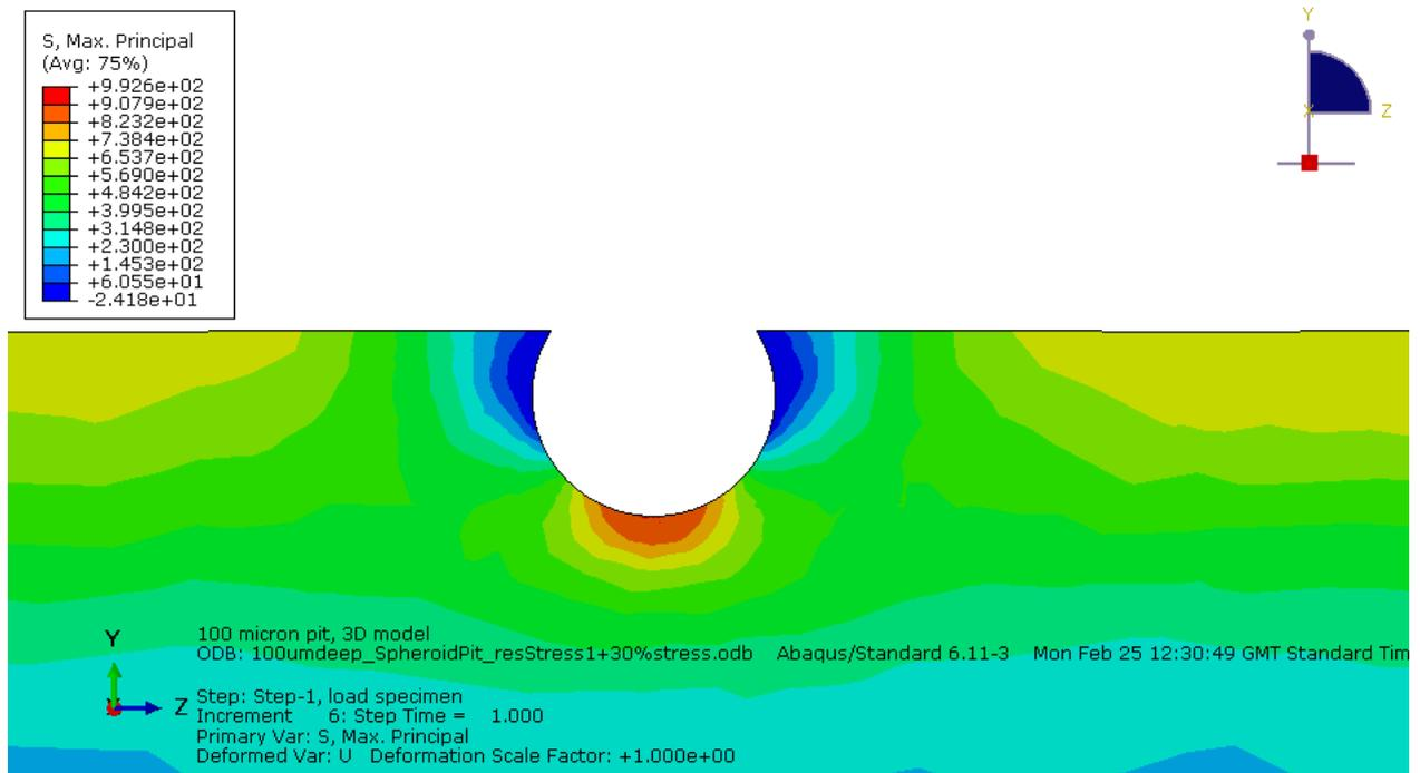
**Figure 9:** Maximum principal stress, longitudinal section, with applied stress of 30%  $\sigma_{0.2}$  superimposed on residual stress.
