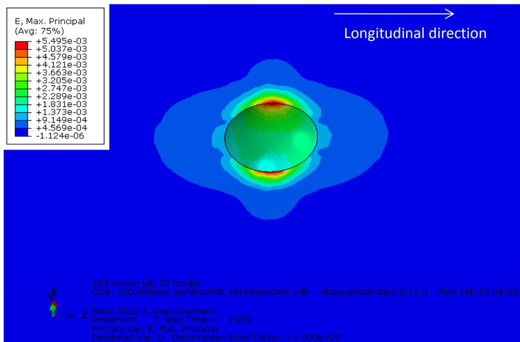
Figure 5: Maximum principal strain in 3D view.
