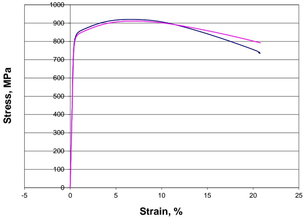
**Figure 1:** Stress-strain behaviour for a FV566 steel in air at 90 °C.
