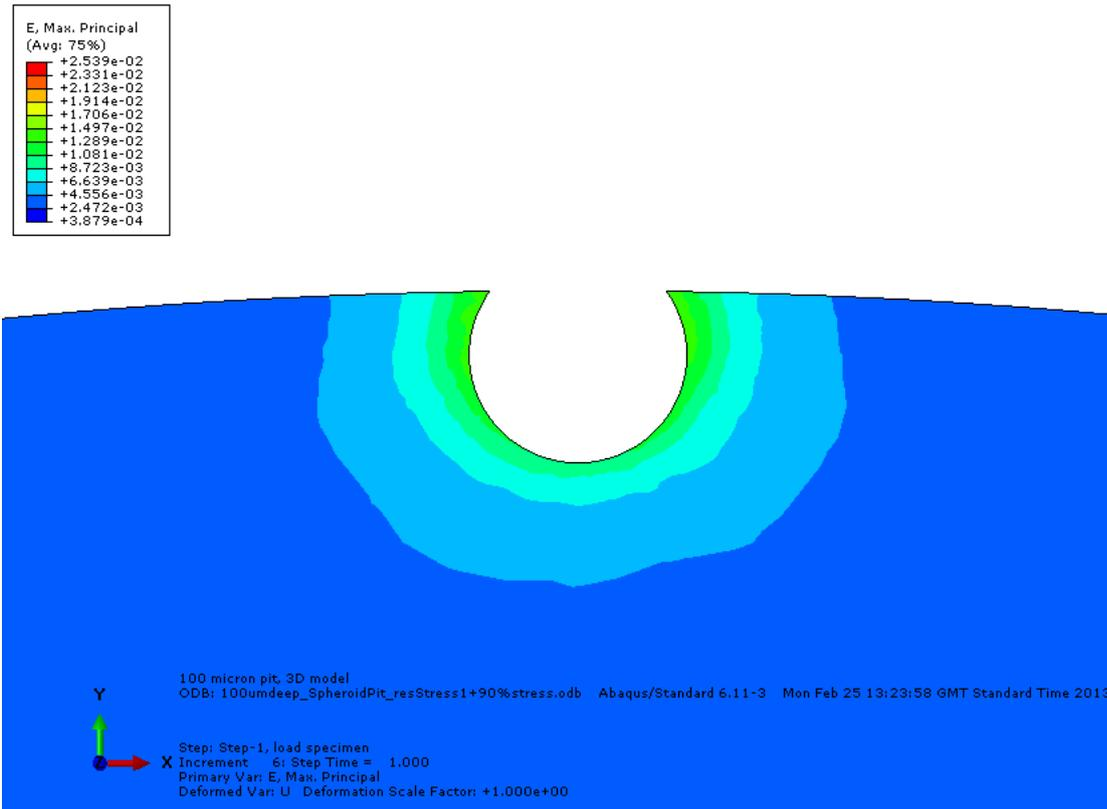
**Figure 12:** Maximum principal strain, cross section view with applied stress of 90%  $\sigma_{0.2}$  superimposed on residual stress.
