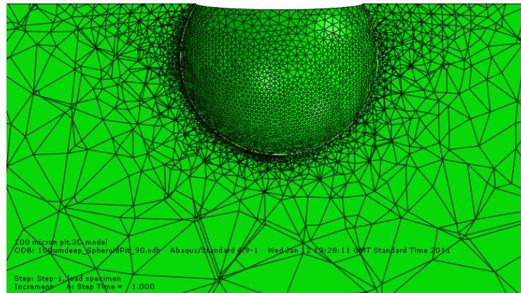
**Figure 2:** Pit geometry showing meshing for 100 µm deep truncated-spherical pit.
