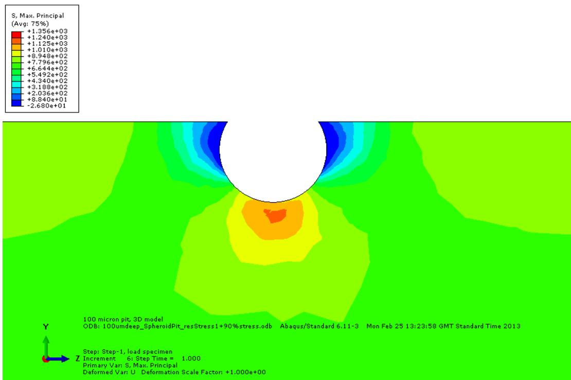
**Figure 13:** Maximum principal stress, longitudinal view, with applied stress of 90%  $\sigma_{0.2}$  superimposed on residual stress.
