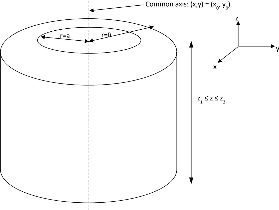
**Figure 3:** Residual stress was assumed tensile in region  $r=R-a$  and compressive in region  $r=a$ .
