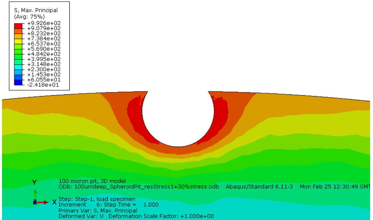
**Figure 8:** Maximum principal stress, cross section view, with applied stress of 30%  $\sigma_{0.2}$  superimposed on residual stress.
