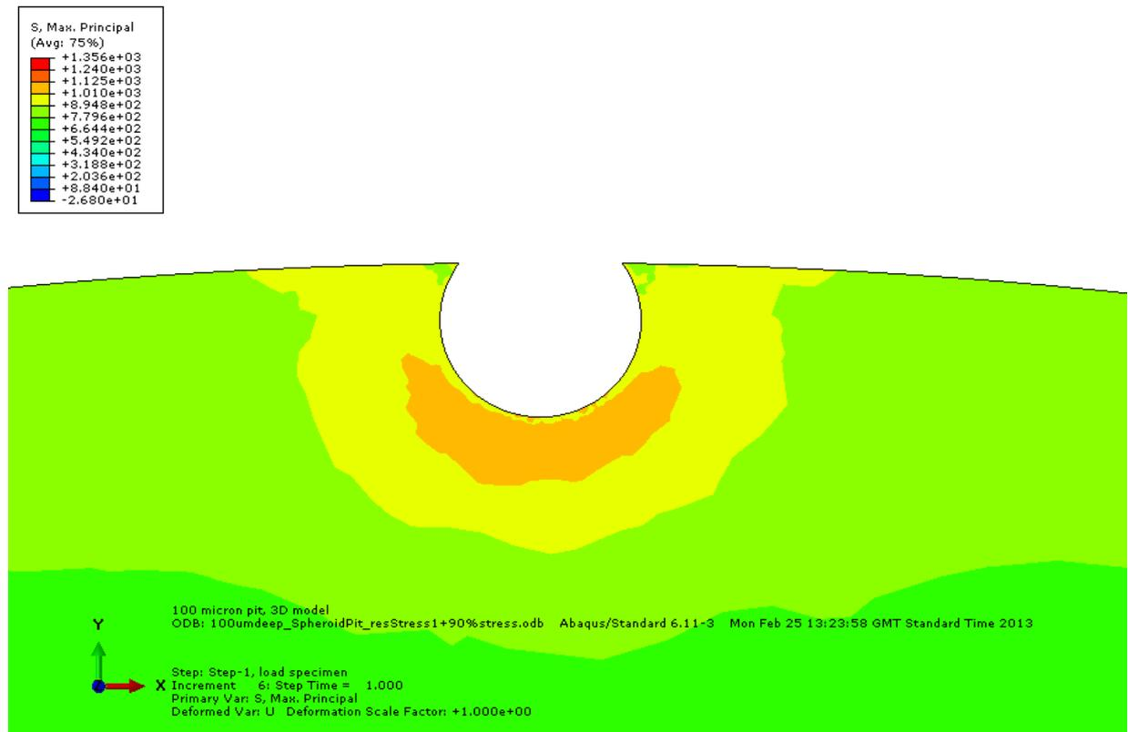
**Figure 11:** Maximum principal stress, cross section view, with applied stress of 90%  $\sigma_{0.2}$  superimposed on residual stress.
