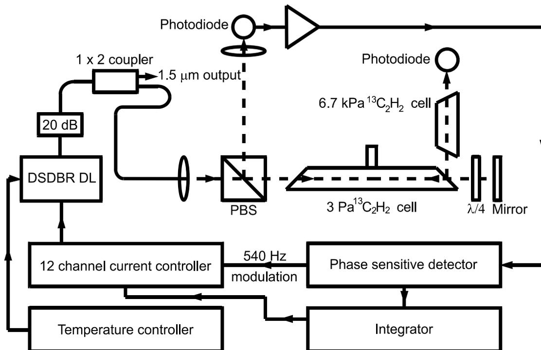
Fig. 1. Experimental arrangement for acetylene spectroscopy
