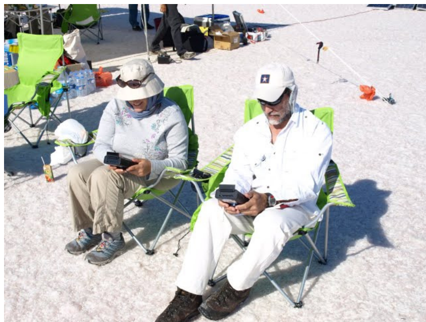
MICROTOPS handheld sunphotometers, Tuz Gölü 2009
