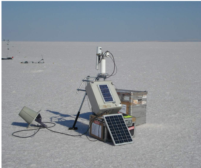
CIMEL sunphotometer used at Tuz Gölü in August 2009
