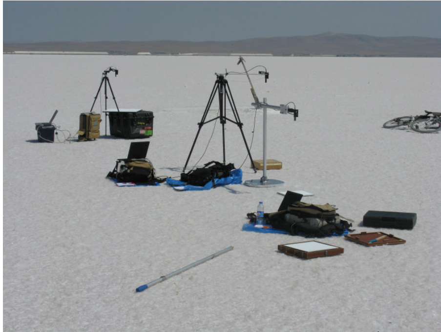
Figure 14: Participants' reference panels were measured in radiance at nadir on 26 th August 2009
