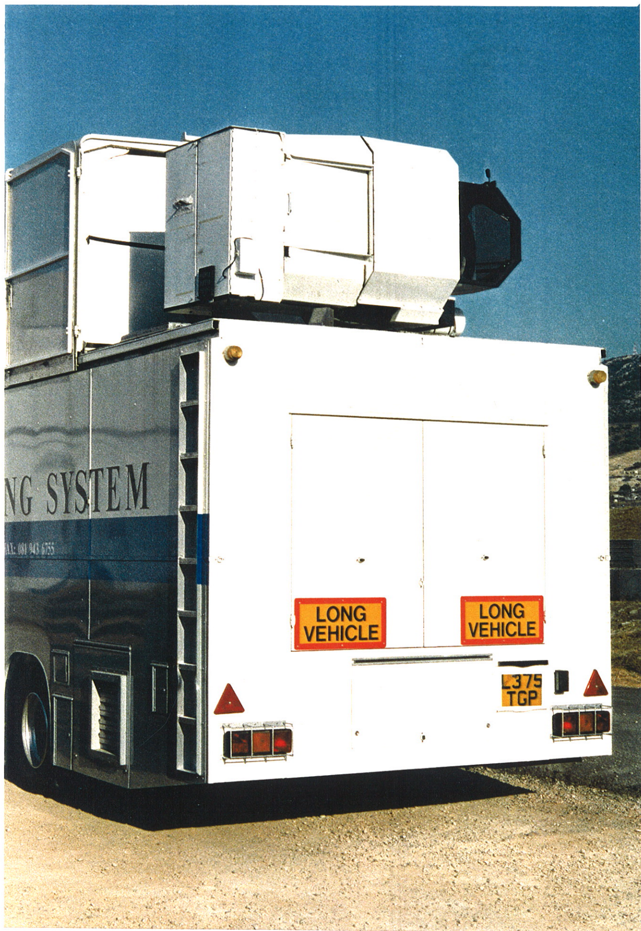
Figure 7: NPL DIAL facility transmitting and receiving telescope, and associated scanning system
