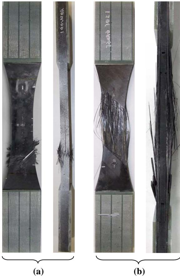
**Figure 15: Failed thick tensile coupons: (a) distributed QI and (b) blocked QI**
