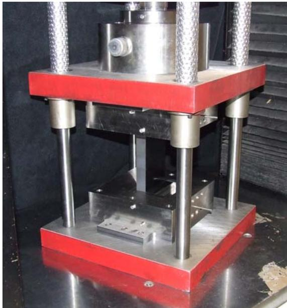
**Figure 12: Large four pillar die set used for end-loaded compression tests**
