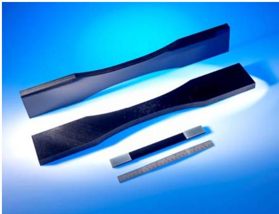
**Figure 2: Comparison between standard multidirectional tensile specimen (~5 mm thick) and thick tensile specimen (~20 mm)**
