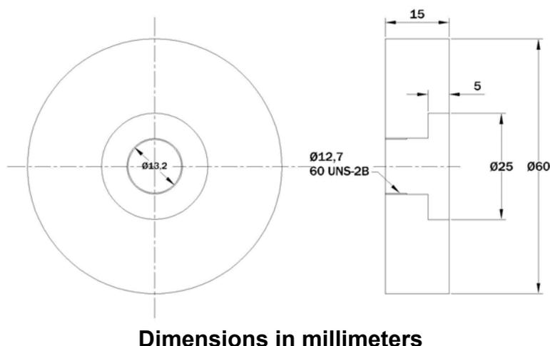
Figure A2 - Adaptor to couple a transmitter microphone to the ear simulator
