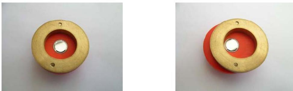
Figure 4. Transmitter microphone mounting for asymmetrical positioning
