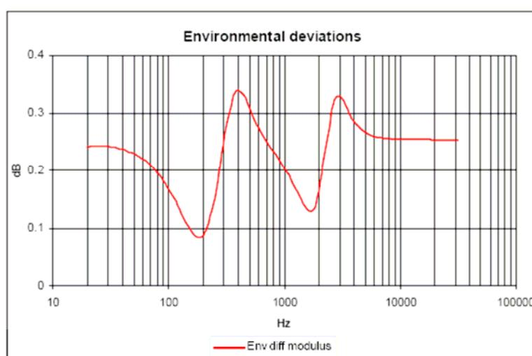
Figure 8. Correction to the lumped parameter model acoustical impedance for a 1°C and 3 kPa variance from the reference environmental conditions.
