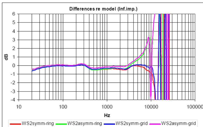
Figure 5. Difference between measured acoustical transfer impedance (magnitude) and lumped parameter model for a WS2 transmitter microphone positioned both symmetrically and asymmetrically. The receiver microphone was fitted either with a protection grid or with a LS2 ring.
