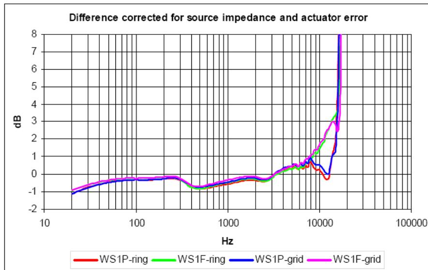
Figure 3. Difference between measured acoustical transfer impedance (magnitude) and lumped parameter model for various combinations of transmitter microphone (type WS1P or WS1F) and receiver configuration (protection grid or ring), corrected for the influence of the finite source impedance and the actuator to pressure response difference.
