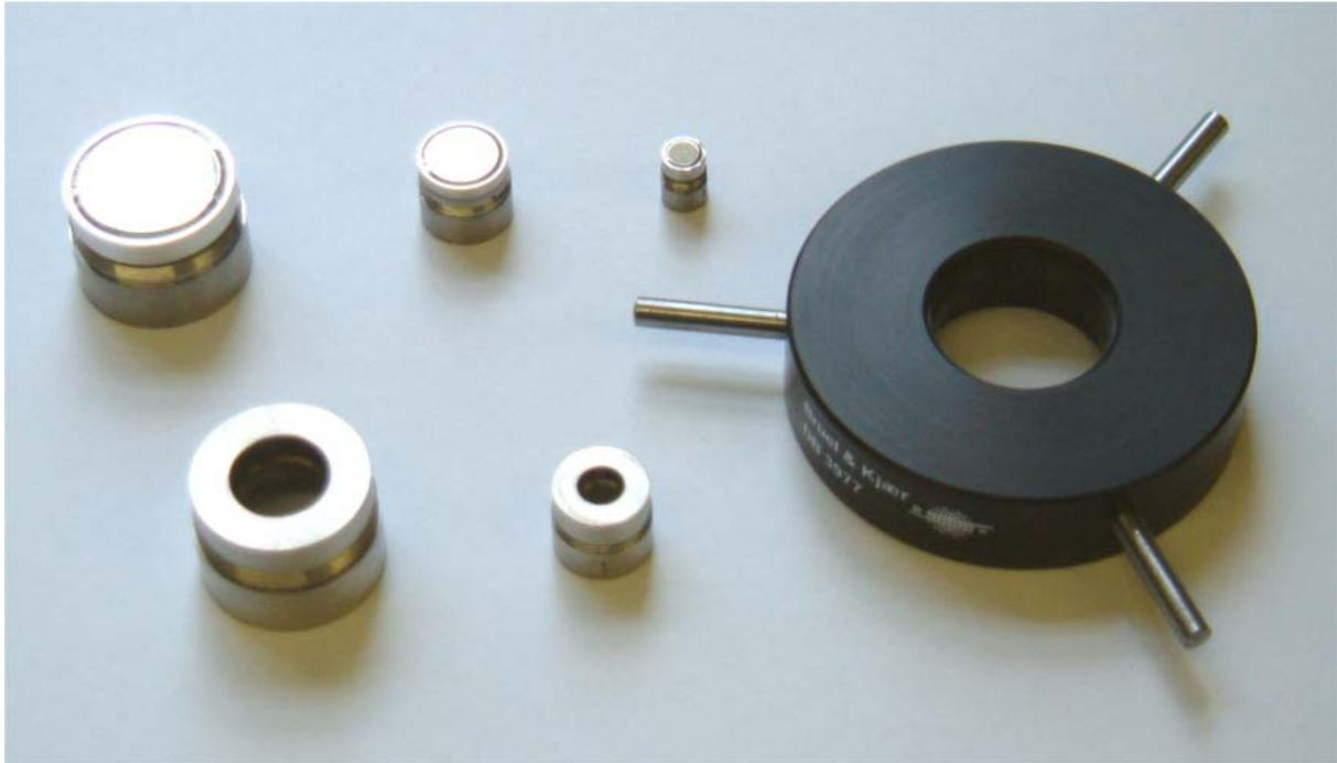
Figure 1. Adaptor for coupling the transmitter microphone to the upper rim of the ear simulator (Brüel & Kjær type DB 3977) together with various microphone & adaptor options.
