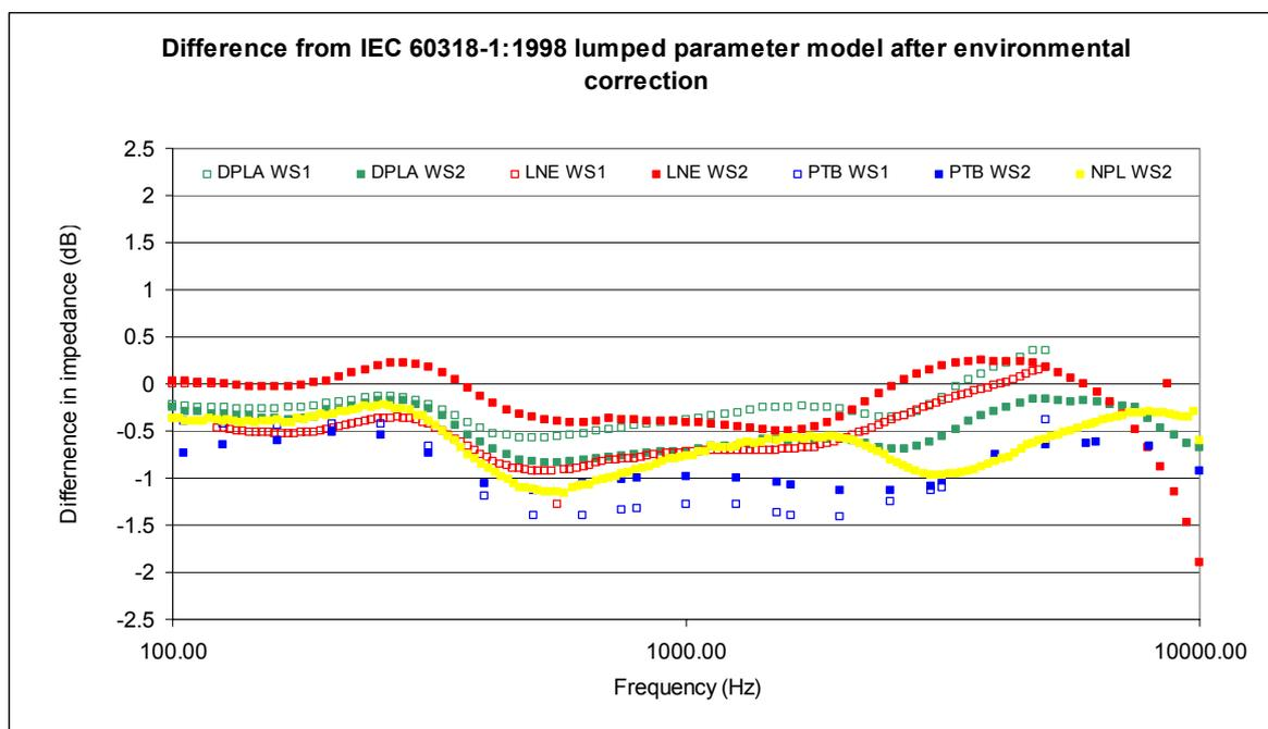
Figure 9. Selected data corrected for variation from reference environmental conditions
