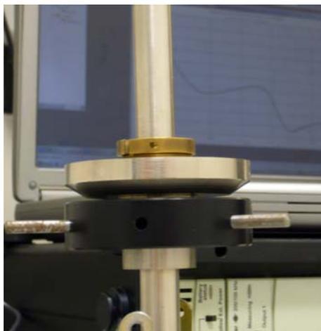
Figure 2. Measurement configuration for coupling the transmitter and receiver microphones to the ear simulator under test.
