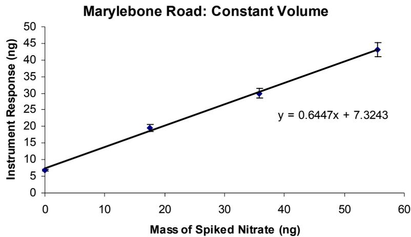
**Figure 3.** *Marylebone Road aqueous calibration with constant volume*
