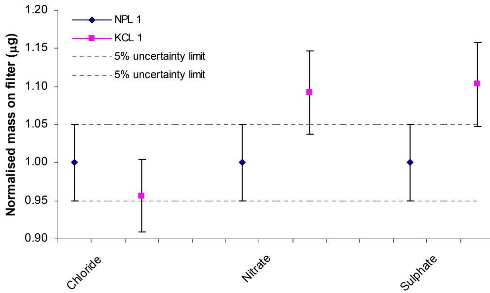
**Figure 1.** *Masses of chloride, nitrate and sulphate measured on a sampled filter, July 2007.*
