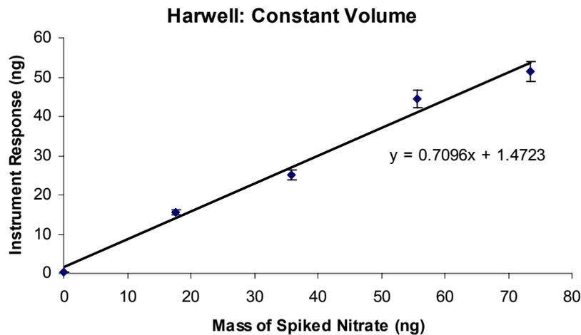
**Figure 4.** *Harwell aqueous calibration with constant volume*
