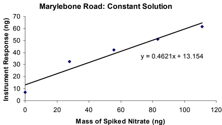
**Figure 2.** *Marylebone Road aqueous calibration with one standard solution*
