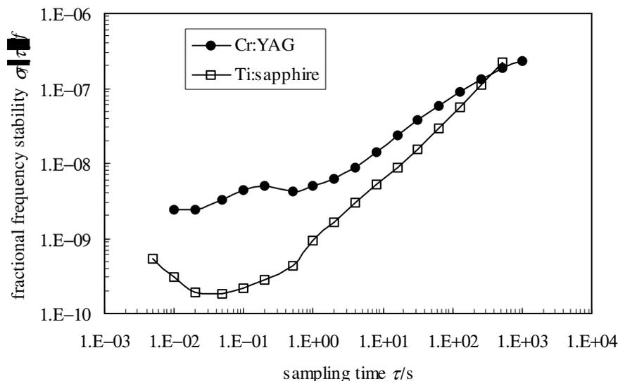
**Figure 2** Fractional frequency stability of the Cr:YAG laser repetition rate, compared to that of a Kerr mode locked Ti:sapphire laser.
