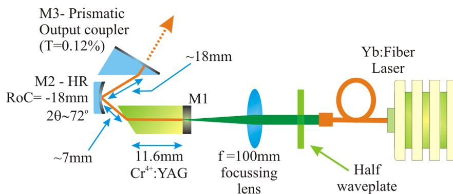
**Figure 1** Schematic of the compact mode-locked Cr:YAG laser.
