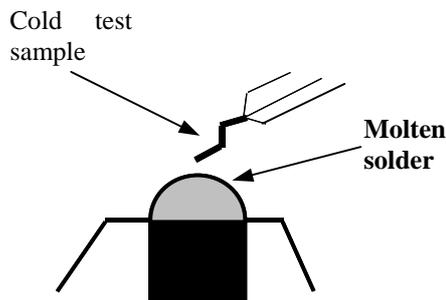
**Figure 1:** Solderability testing
