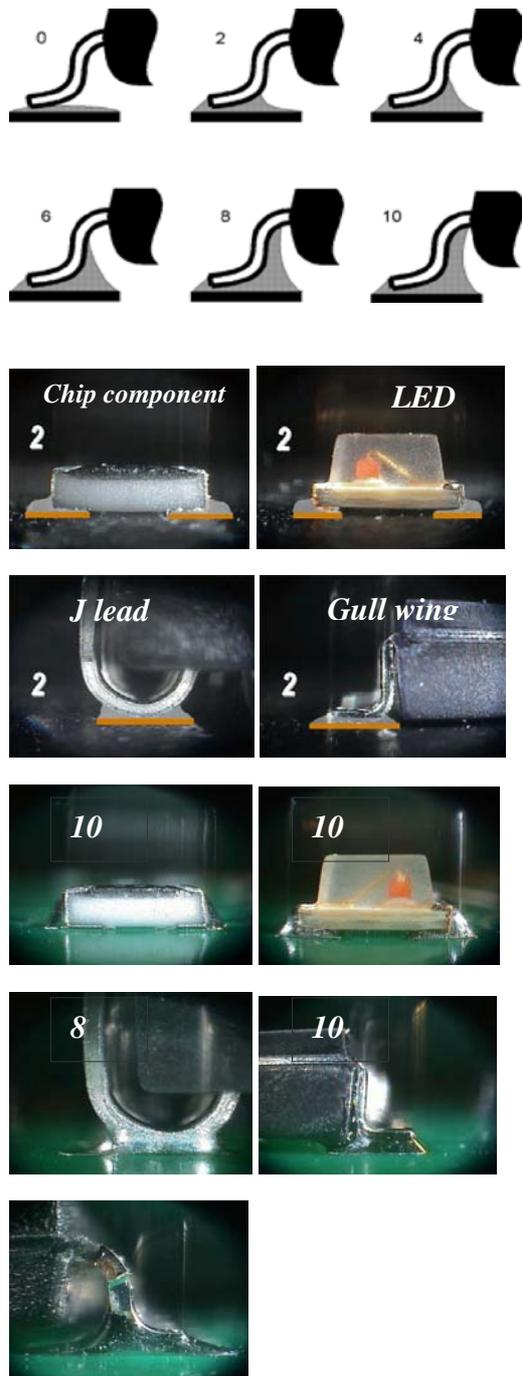
**Figure A8** Solder joint scores used in visual inspection
