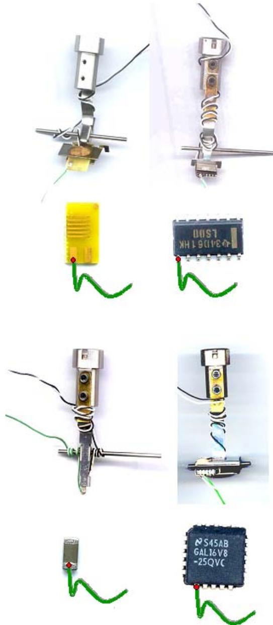
Figure 6 The positions of the thermocouples on clip and component
