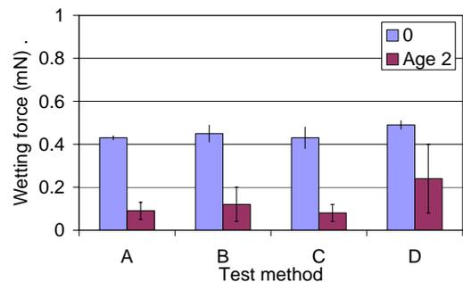
**Figure A1** Wetting force from different methods for SOIC14
