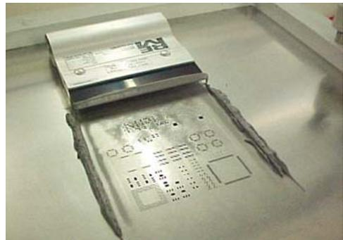
**Figure A7** Board and stencil used for assembly
