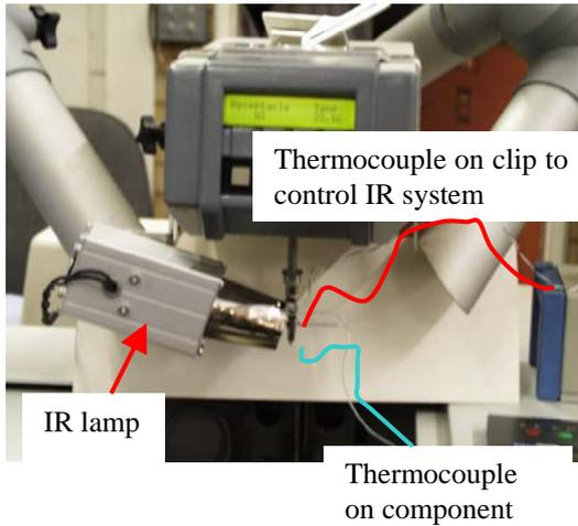
Figure 3 Solderability testing with IR system
