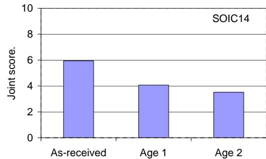
**Figure A10** Joint score with ageing time for SOIC14
