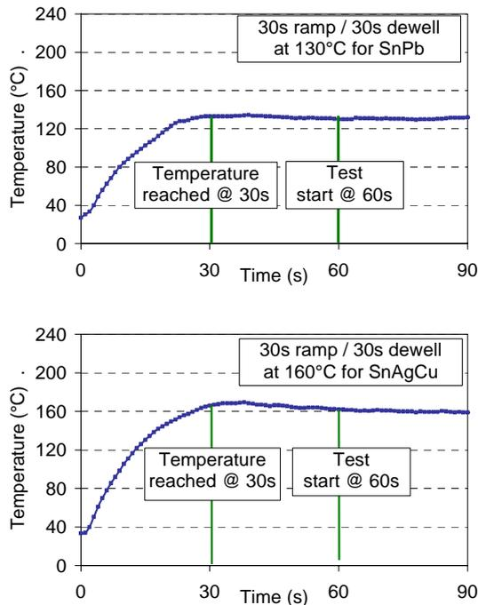
**Figure 8** Preheat temperature profile for SnPb and SnAgCu alloy
