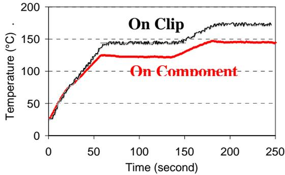
**Figure 7** Temperature difference between two thermocouples for a C1206 component
