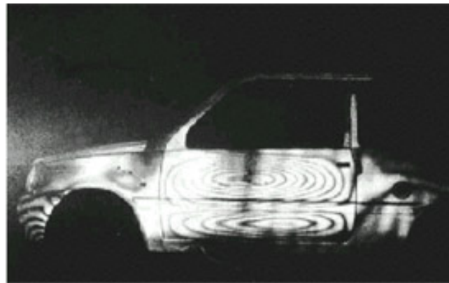
Figure 3.6: Fringes show the deformation of the object compared to when the initial hologram was recorded.
