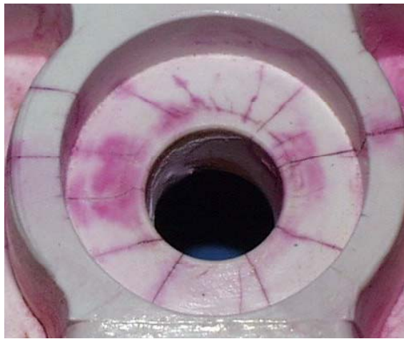
Figure 2.1: Use of dye penetrant to highlight small cracks.
