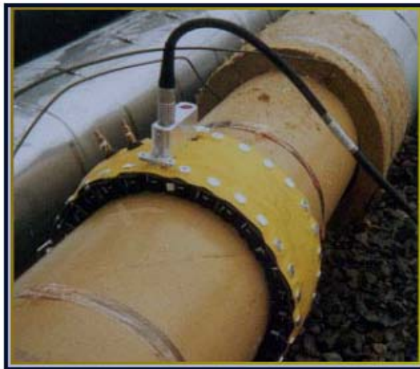
Figure 5.7: Ring actuator and sensor for long range ultrasonic testing on pipelines.
