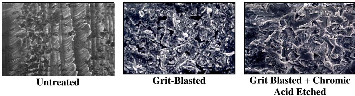
Figure 8.1: SEM images of different surface treatments of 6Al-4V-titanium alloy for adhesive bonding (magnification x 900).
