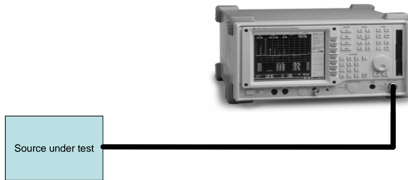
Figure 7: Phase noise measurement with a spectrum analyzer
