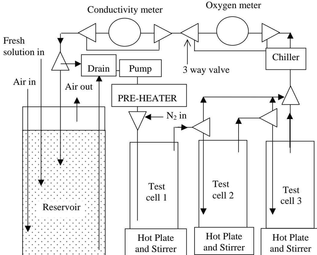
**Figure 1.** Schematic diagram of the test solution circulation loop.
