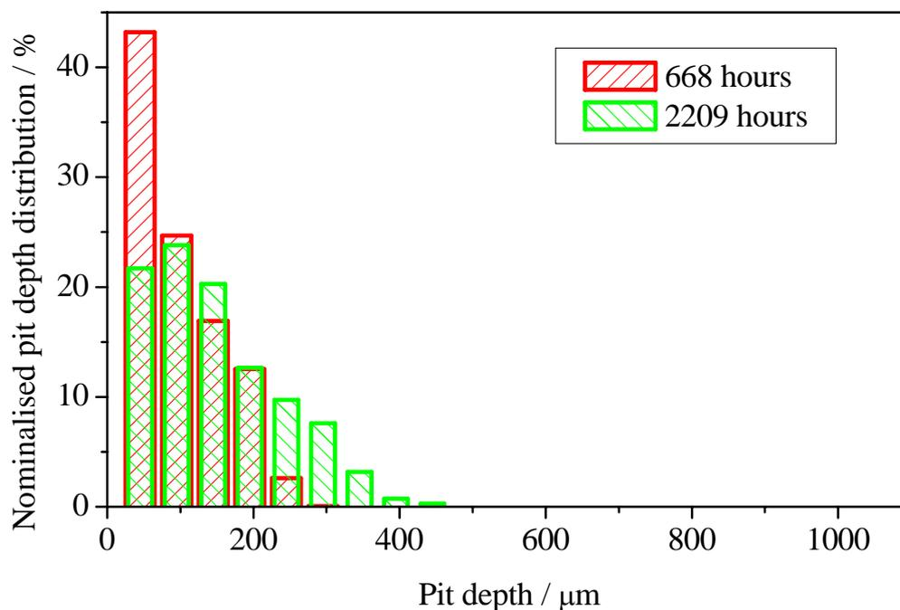
Figure 3. The normalised distribution of pit depths in the specimens tested for 668 hours and 2209 hours
