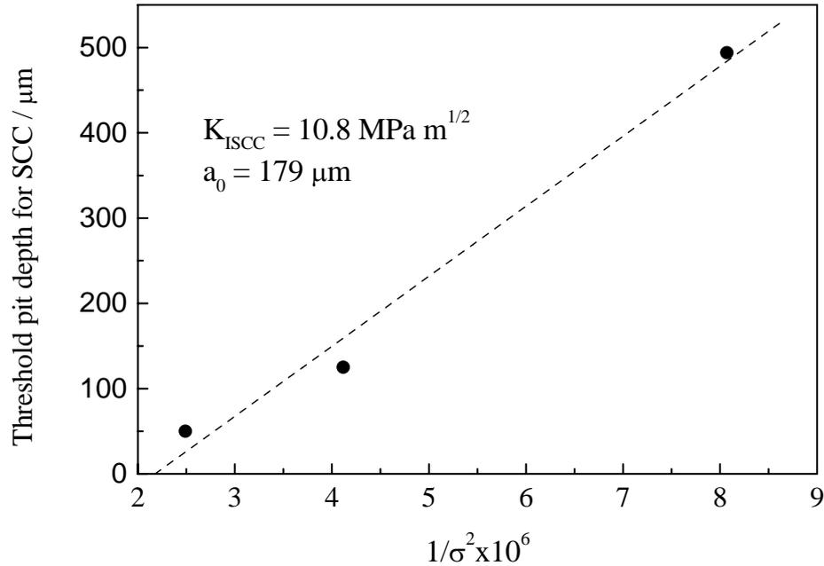
Figure 6 Dependence of threshold pit depth as a function of  $1/\sigma^2$ .
