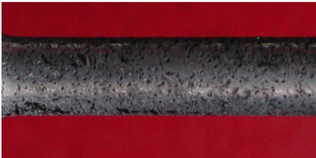
Figure 2. Surface appearance of a self-loaded cylindrical tensile specimen tested in aerated 1.5 ppm  $\text{Cl}^-$  solution at 90 °C for 171 h.
