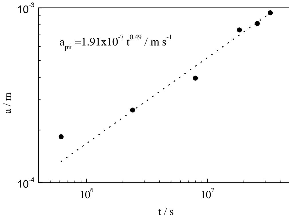
Figure 5 Time dependence of the average depth of 10 deepest pits in the disc steel tested in aerated 1.5 ppm chloride solution at 90 °C.
