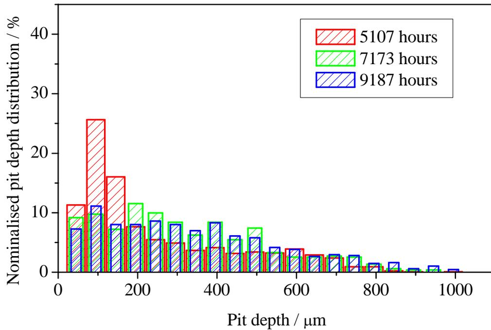
Figure 4. The normalised distribution of pit depth in the specimens tested for 5107 hours, 7173 hours and 9187 hours
