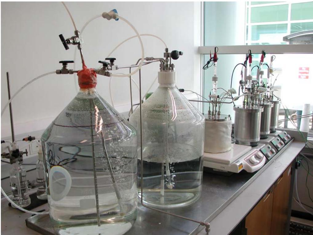
**Figure 1.** Arrangement of four test cells for cyclic water chemistry; the reservoir with deaerated 300 ppb  $Cl^-$  + 300 ppb  $SO_4^{2-}$  is out of shot.
