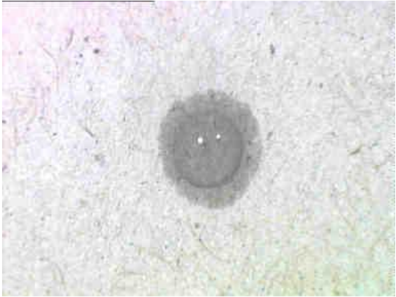
Figure 27: Liquid drop spreading on a rough, porous surface
