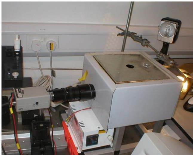
Figure 15: Apparatus for measuring contact angles of molten hot melts
