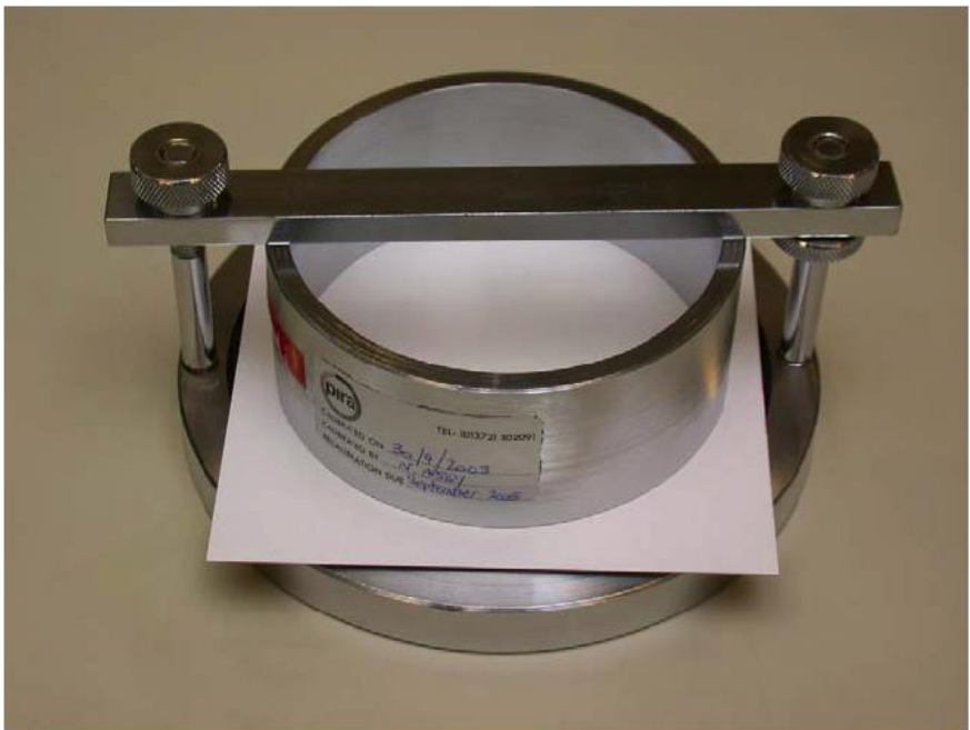
Figure 20: Cobb absorbance test
