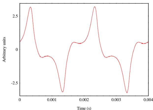
Figure 1. Primary current (magnetic field strength) waveform showing considerable distortions due to the non-linear material behaviour.
