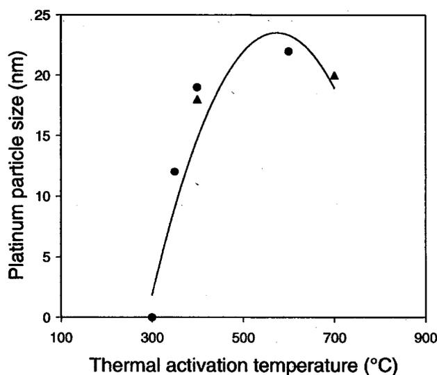
**Figure 2.6** Effect of thermal activation temperature on mean Pt particle size from XRD (●) and TEM (▲) measurements on Pt/C catalysts<sup>48</sup>.
