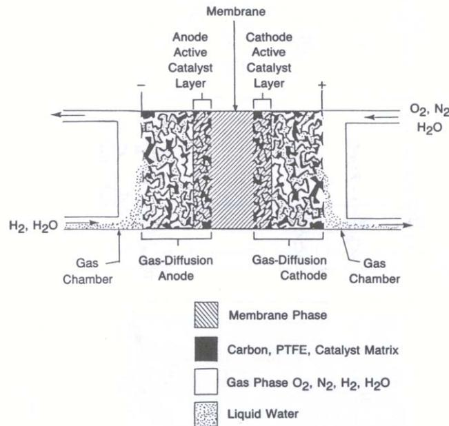
**Figure 1.1** Components of a PEMFC<sup>1</sup>.
