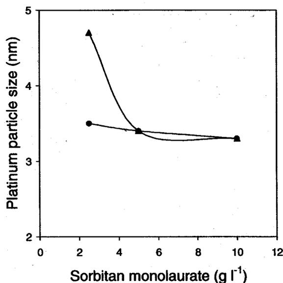
**Figure 2.4** Effect of sorbitan monolaurate concentration on mean Pt particle size before (●) and after (▲) heat treatment<sup>35</sup>.
