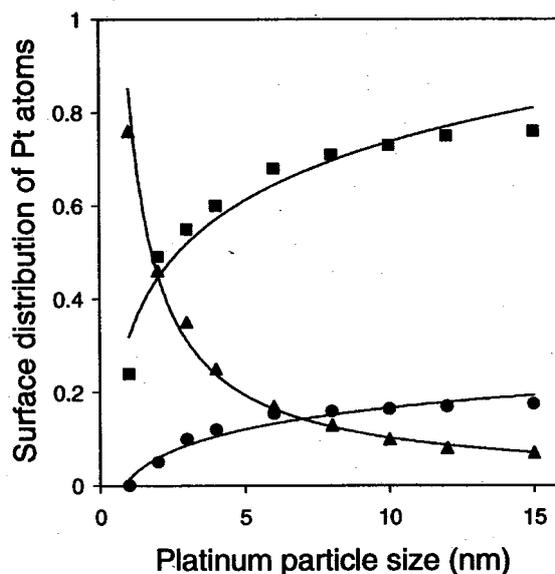
**Figure 2.7** Surface distribution of Pt atoms as a function of particle size:  $\langle 100 \rangle$  atoms (●),  $\langle 111 \rangle$  atoms (■) and edge/corner atoms (▲)<sup>54</sup>.
