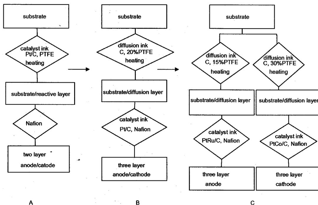
**Figure 3.1** Evolution of typical preparation methods for PEMFC electrodes<sup>55</sup>.
