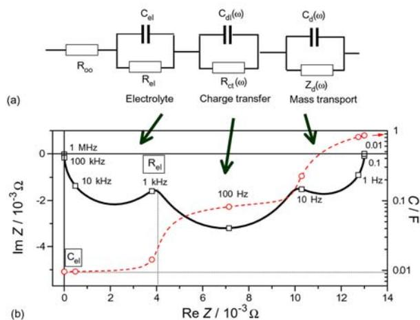
**Figure 3.7** (a) General equivalent circuit for a PEMFC (b) Schematic frequency response of impedance and capacitance<sup>124</sup>.
