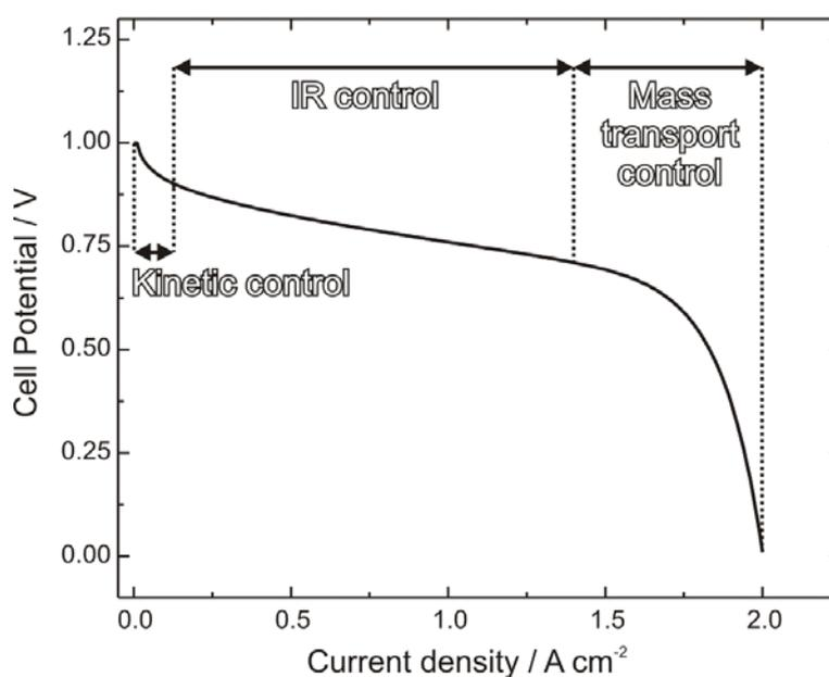
**Figure 3.4** Typical polarisation curve for a PEMFC.
