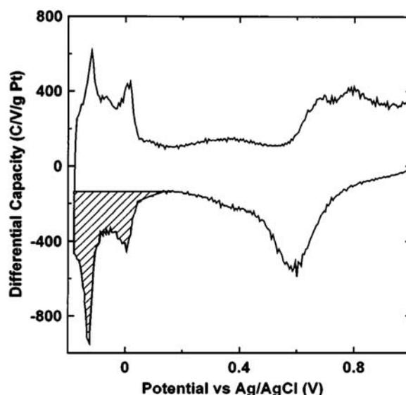
**Figure 3.5** Illustration of the method used to calculate active surface area using hydrogen adsorption voltammetry<sup>111</sup>. The shaded area represents the charge due to hydrogen adsorption.
