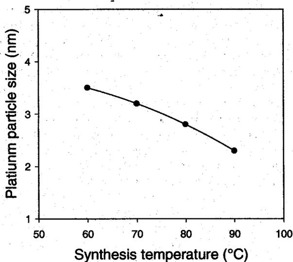
**Figure 2.5** Effect of synthesis temperature on mean Pt particle size<sup>36</sup>.
