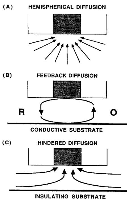
Figure 4.2 Principle of SECM operation in feedback mode far from substrate (A) and close to conducting (B) and insulating (C) substrates<sup>130</sup>.
