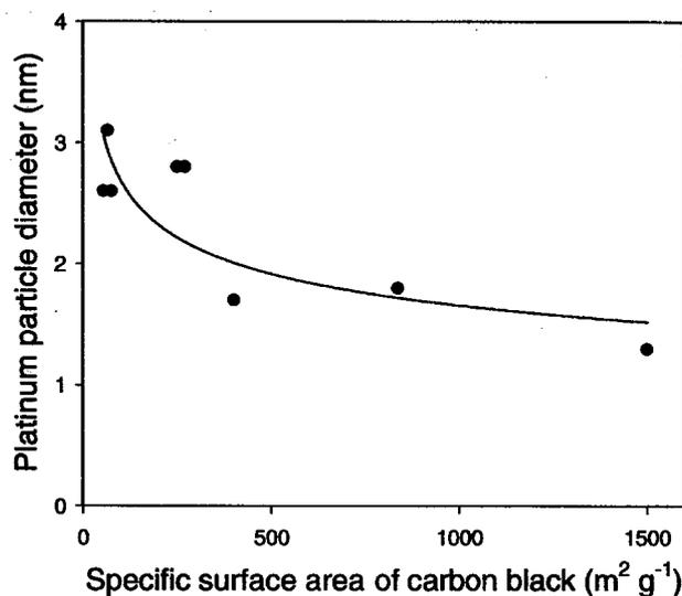
**Figure 2.3** Effect of specific surface area of carbon support on mean Pt particle size<sup>32</sup>.
