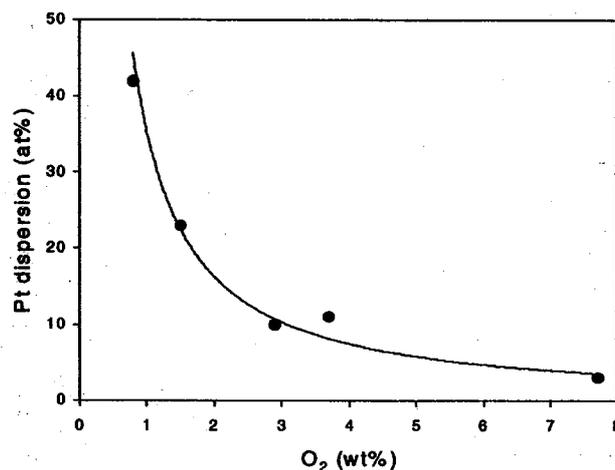
**Figure 2.2** Effect of surface oxygen concentration of carbon support on Pt dispersion in Pt/C catalysts<sup>17</sup>.
