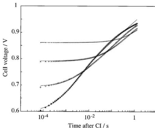
**Figure 3.6** Relaxation curves of PEMFC voltage after current interruption for current densities of (.) 1, (x) 10, (+) 100 and (\*) 400 mA/cm<sup>2</sup> before interruption<sup>121</sup>.
