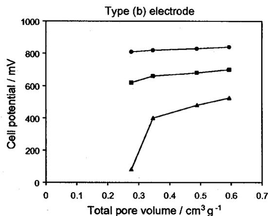
**Figure 3.3** Cell potential as a function of total pore volume in the diffusion layer at 100 mA/cm<sup>2</sup> (●), 400 mA/cm<sup>2</sup> (■) and 700 mA/cm<sup>2</sup> (▲)<sup>83</sup>.
