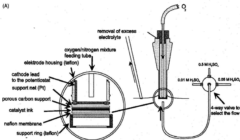
**Figure 4.1** Measuring device for half cell characterisation of cathode catalyst layers<sup>127</sup>.
