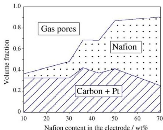
**Figure 3.2:** Volume fraction of gas pores, Nafion and Pt/C in an electrode as a function of Nafion content<sup>79</sup>.
