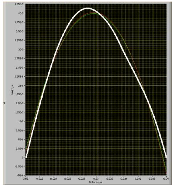
**Figure 7** Front panel of Labview™ routine used to fit circles and parabolae to coupon bending data
