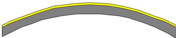
**Figure 1** Schematic diagram showing a coated sample (coating is yellow) with thermal mismatch compressive stress in the coating
