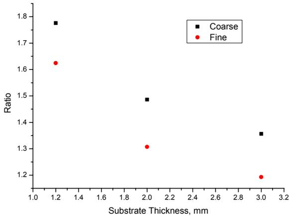
**Figure 10** Ratio of value of residual stress calculated from Freund analysis to value calculated from Stoney formula.
