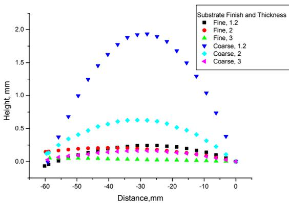
**Figure 2 Results of measurements on thermally sprayed WC/Co samples. The figure in the legend denote substrate thickness.**
