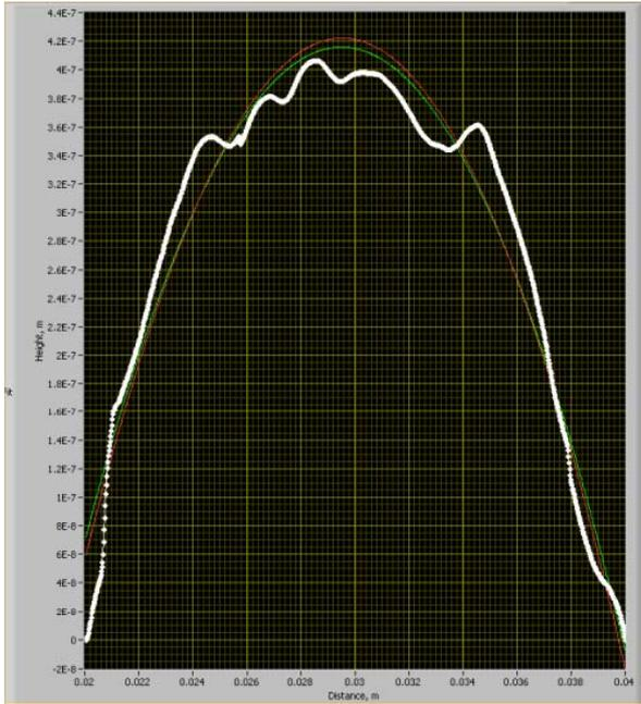
**Figure 8** Plot of change in bending for two profiles measured with Flexus instrument at two temperatures of 21°C and 78°C.
