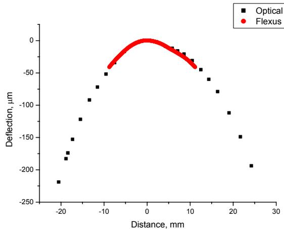
**Figure 6** Comparison of measurements of bend of FeCrAlY sample with optical and flexus instruments.
