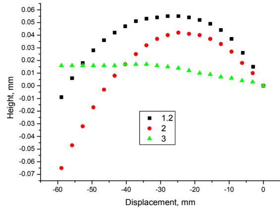
**Figure 4 Profiles of coarse grit blasted substrates. Numbers in legend refer to thickness of substrate. The radius of curvature results are plotted in Figure 5. The different points for the same conditions are measurements on different samples. The radius of curvature for the coarse grit blast samples are larger than those for the fine grit blast samples. There is also a large scatter in the results.**
