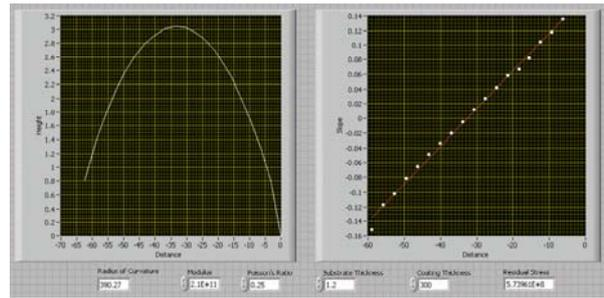
**Figure 3 Front panel of Labview™ routine to evaluate curvature and residual stress in coatings. Left hand panel shows fit though data, right hand panel shows regression fit of slopes to derive curvature.**
