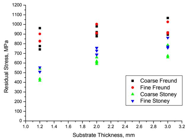
**Figure 9** Residual stress in coating calculated by Freund analysis and Stoney formula.
