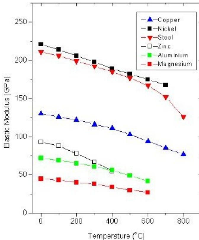
Figure 1: Variation of modulus with temperature for a variety of metals [1].
