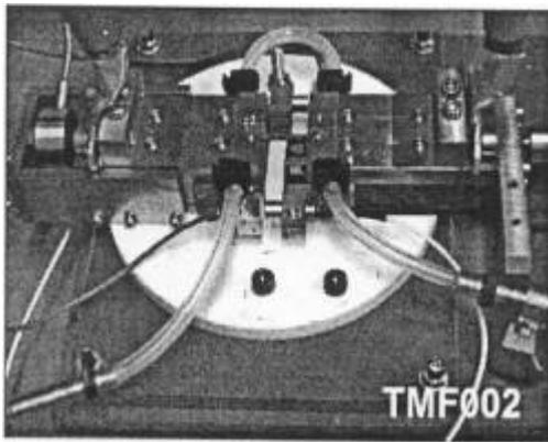
Figure 2: Photograph of the modified ETMTrig
