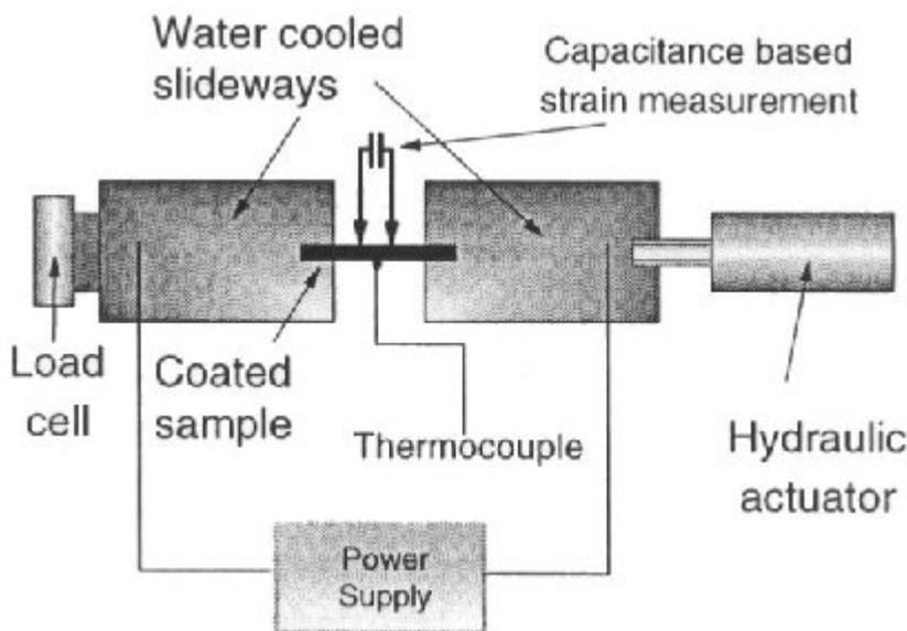
**Figure 5: Schematic diagram of the re-designed ETMT-TMF rig**
