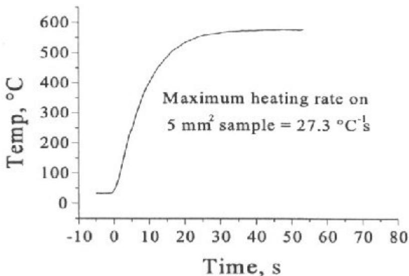
Figure 3: Maximum heating rate for a 5 mm<sup>2</sup> cross-section testpiece
