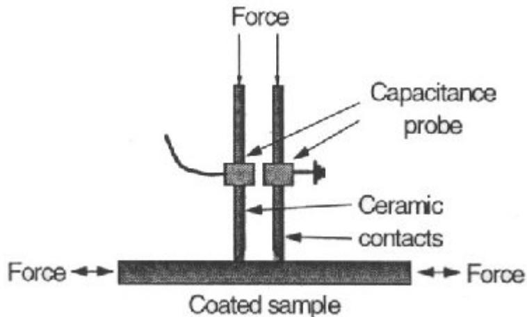
**Figure 4: A schematic diagram of the capacitance probes directly attached to the testpiece for the measurements of strain**
