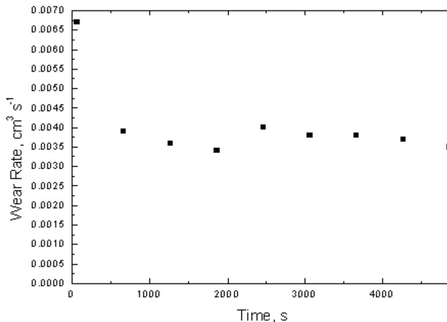
**Figure 9, Variation in wear rate with time for interrupted test carried out using rubber wheel test under dry conditions and test load of 75 N.**
