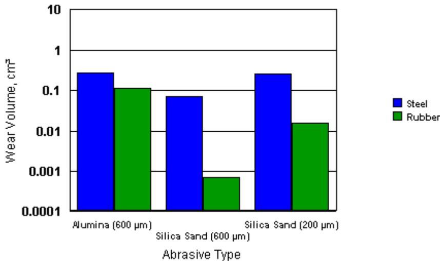
**Figure 8, Variation in wear volume with type of abrasive**
