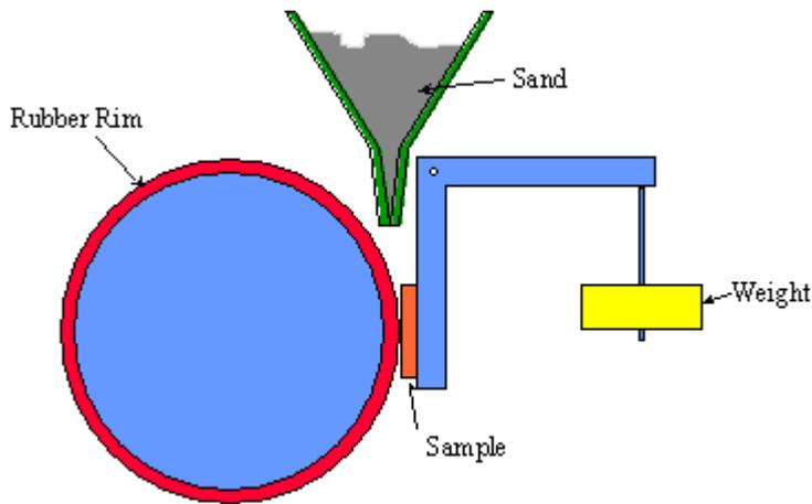
**Figure 1, Schematic diagram of original ASTM G65 test system**
