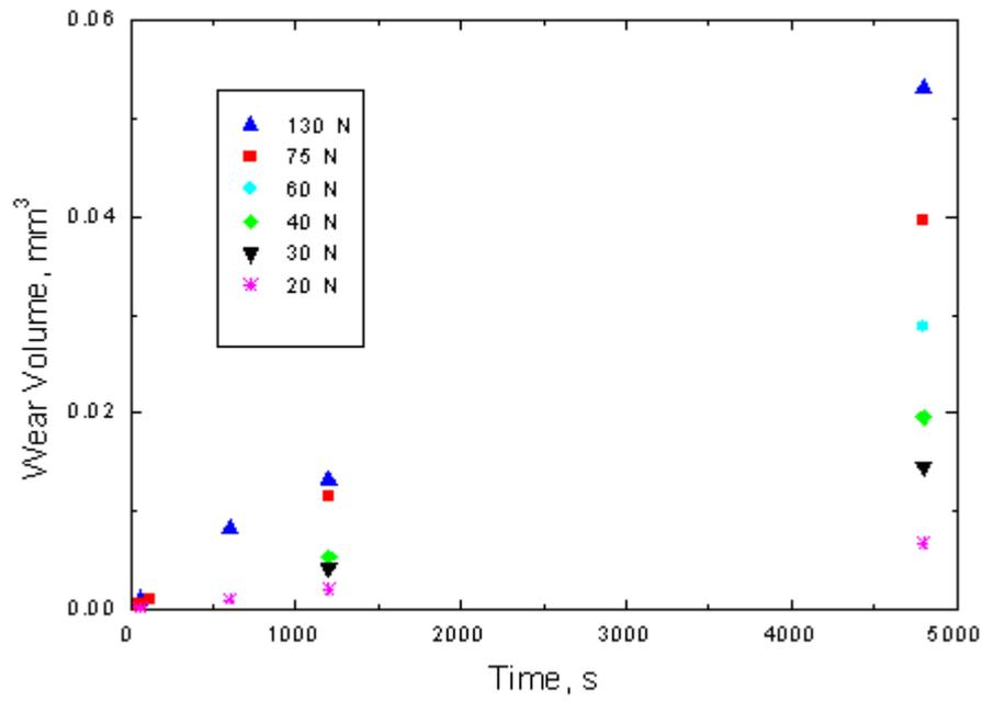
Figure 4, Variation in wear volume with test load and duration for tests carried out using rubber wheel and dry conditions
