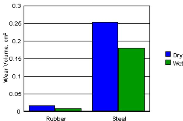
**Figure 7, Variation in wear volume for wheel material in tests**
