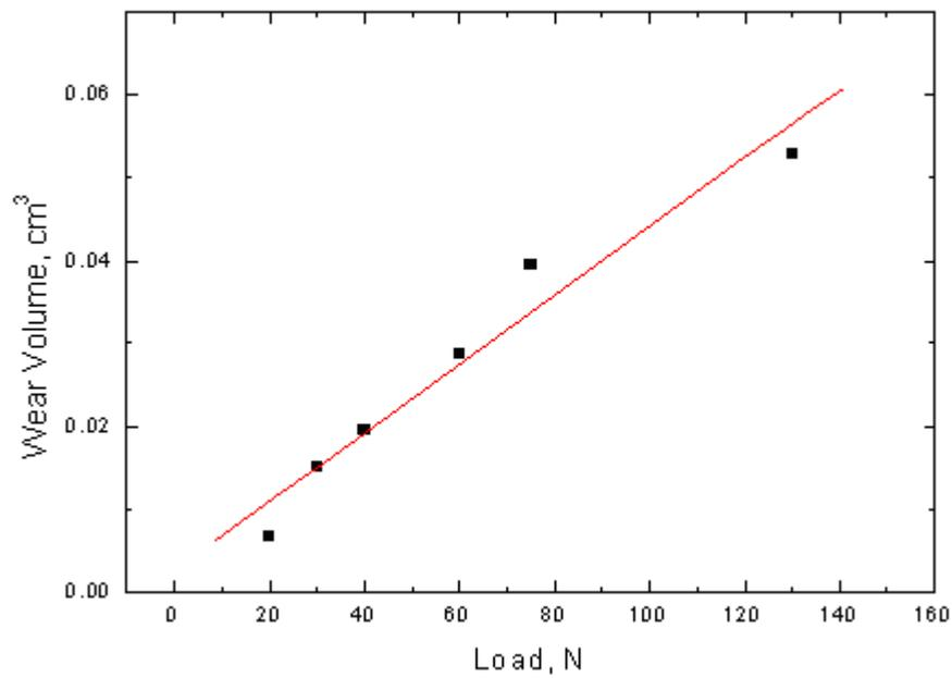
Figure 5, Variation in wear volume with test load for tests carried out using rubber wheel and dry conditions for a duration of 4800 s
