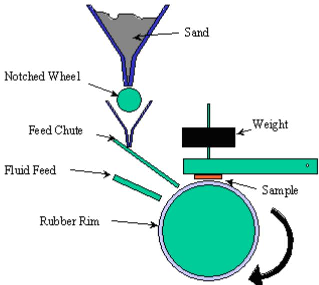
Figure 2, Schematic diagram of modified test system
