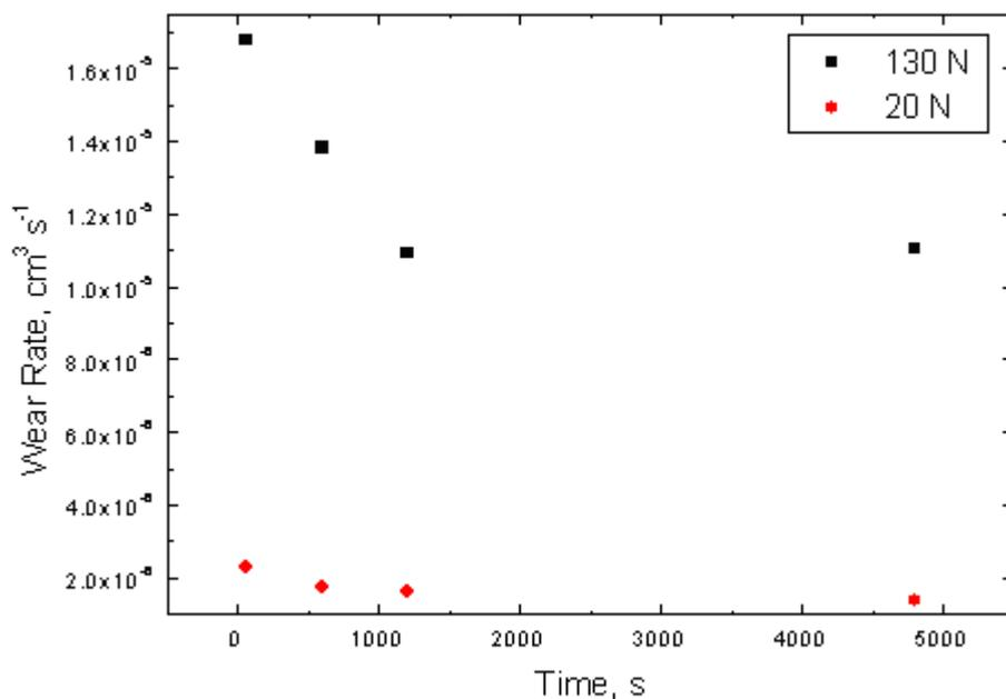
**Figure 6, Variation in wear rate with time for two loads carried out using rubber wheel and dry conditions.**
