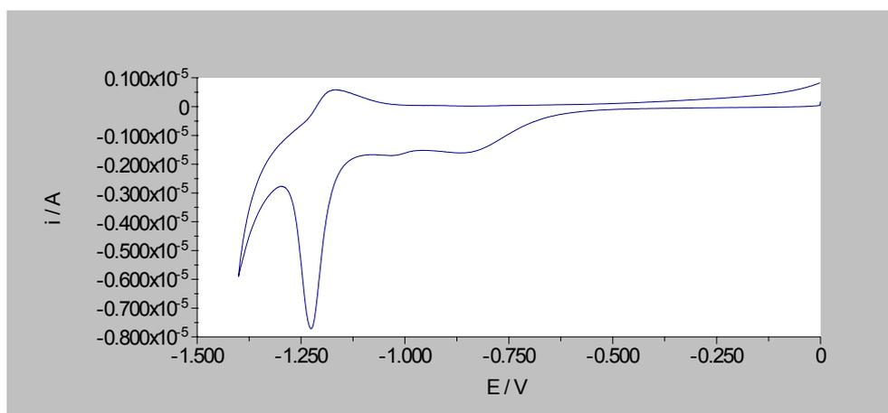
**Figure 7(a).** Reductive desorption of biotin-HPDP in 0.1M NaOH at a scan rate of  $20 \text{ mVs}^{-1}$ . Assembly time of 60mins.
