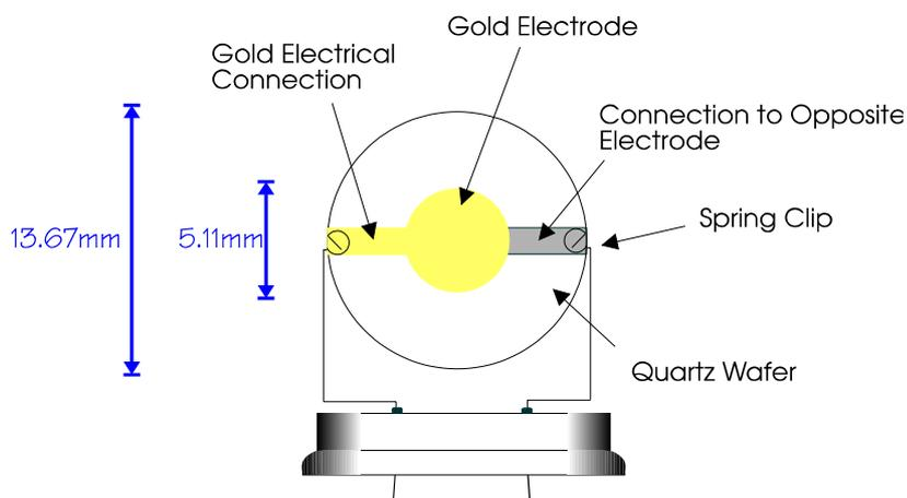
**Figure 3.** Dimensions of the EQCM crystal
