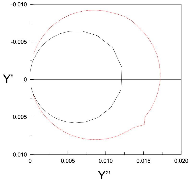
**Figure 4(a).** Complex plane admittance plot of  $C_{18}$  (dashed red line) and bare gold (solid black line) at low resolution between  $9.975 \times 10^6$  and  $1.0025 \times 10^7$  Hz
