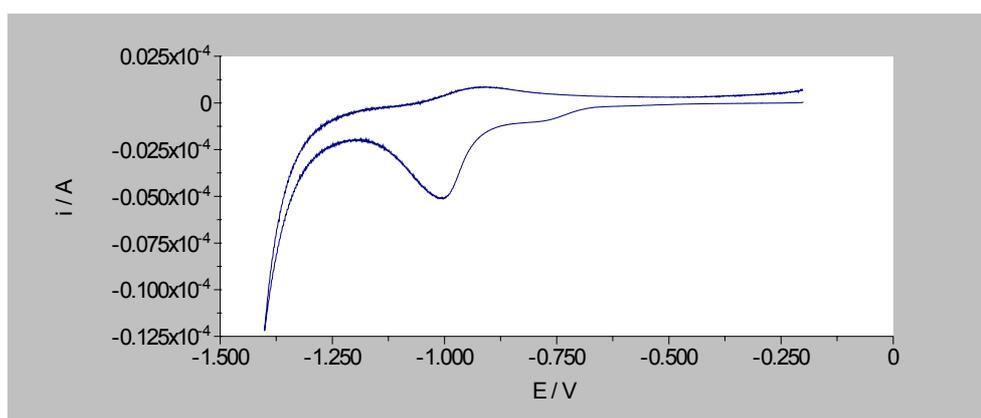
**Figure 6.** Reductive desorption of benzene thiol in 0.1M NaOH at a scan rate of  $20 \text{ mVs}^{-1}$ .
