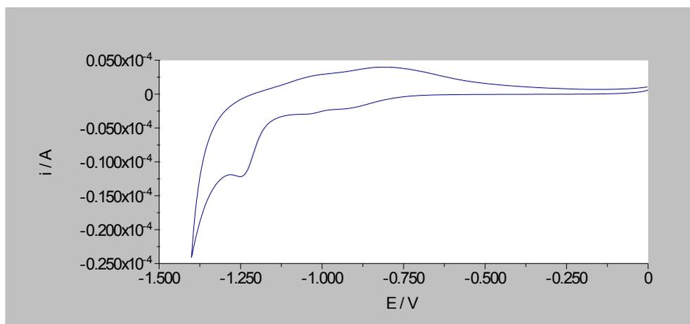
**Figure 7(b).** Reductive desorption of biotin-HPDP in 0.1M NaOH at a scan rate of  $20 \text{ mVs}^{-1}$ . Assembly time of 1440 mins.
