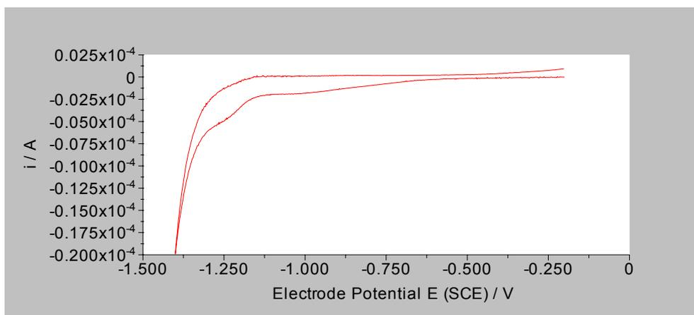
**Figure 8.** Reductive desorption of biotin-HPDP, formed by direct assembly without chemical reduction, in 0.1M NaOH at a scan rate of 20  $\text{mVs}^{-1}$ . Assembly time of 60 mins.
