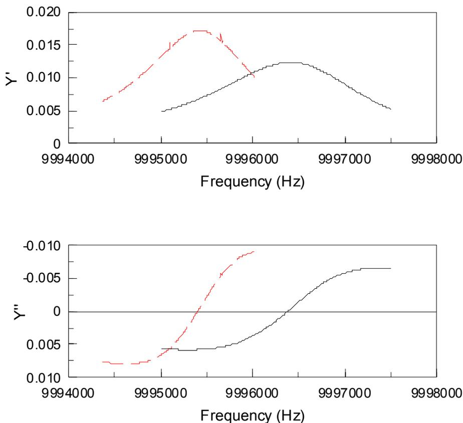
**Figure 4(c).** Bode plots of  $C_{18}$  (dashed red line) and bare gold (solid black line) close to the fundamental oscillation.
