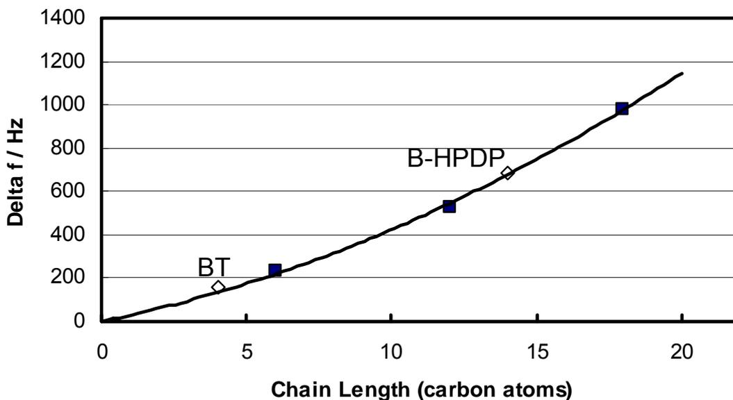
**Figure 5.** Frequency shift in the maximum conductance of the admittance against carbon chain length for ‘calibration’ alkanethiols (■) of C<sub>6</sub>, C<sub>12</sub> and C<sub>18</sub>. Equivalent Alkane Thiol Chain Lengths (EATCLs) for benzene thiol (◇ BT) and biotin-HPDP (◇ B-HPDP) derived SAMs have then been interpolated from experimentally observed frequency shifts.
