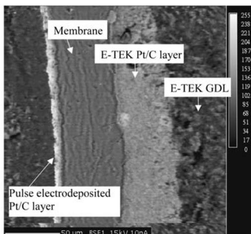
**Fig. 9:** Backscattered electron image of a typical MEA cross-section<sup>61</sup>.
