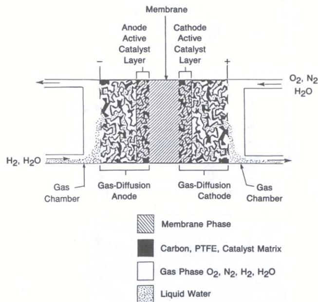
**Fig. 1:** Components of a PEMFC<sup>1</sup>.
