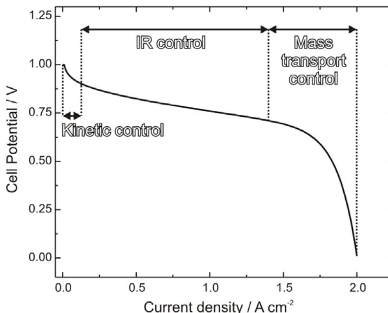
**Fig. 2:** Typical polarisation curve for a PEMFC.
