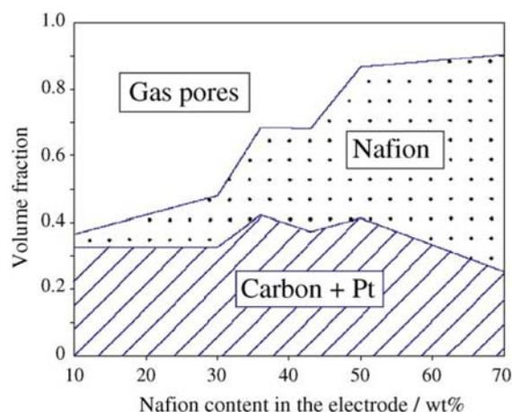
**Fig. 11:** Volume fraction of gas pores, Nafion and Pt/C in an electrode as a function of Nafion content<sup>70</sup>.
