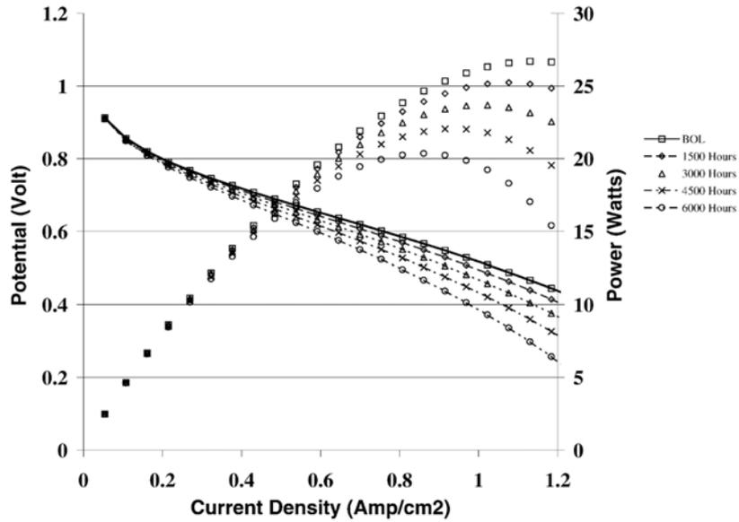
**Fig. 13:** Simulation of cell ageing using the model of Fowler et al<sup>140</sup>.
