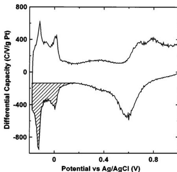
**Fig. 4:** Illustration of the method used to calculate active surface area using hydrogen adsorption voltammetry<sup>27</sup>. The shaded area represents the charge due to hydrogen adsorption.
