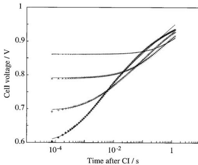
**Fig. 7:** Relaxation curves of PEMFC voltage after current interruption for current densities of (.) 1, (x) 10, (+) 100 and (\*) 400 mA/cm<sup>2</sup> before interruption<sup>48</sup>.
