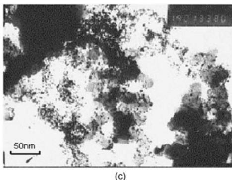
**Fig. 10:** TEM micrograph of Pt/C electrocatalyst<sup>62</sup>.
