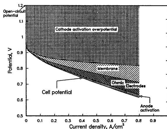
**Fig. 12:** Model calculations of the contributions to PEMFC losses as a function of current density with no mass transport limitation<sup>82</sup>.
