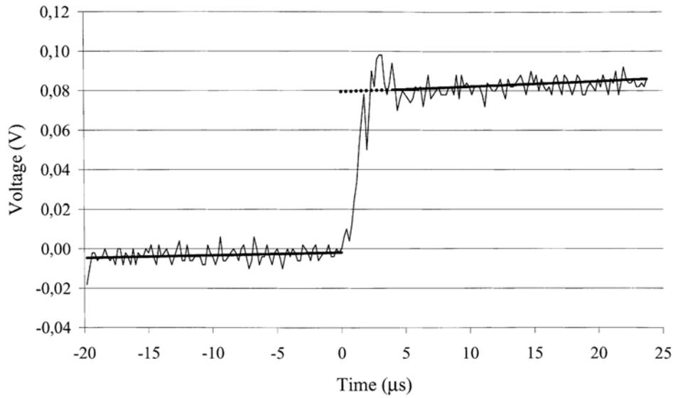
**Fig. 6:** Voltage transient for an individual cell in a PEMFC stack during current interruption<sup>46</sup>. Extrapolation is indicated by the dotted line. Current density before interruption is 400 mA/cm<sup>2</sup>.
