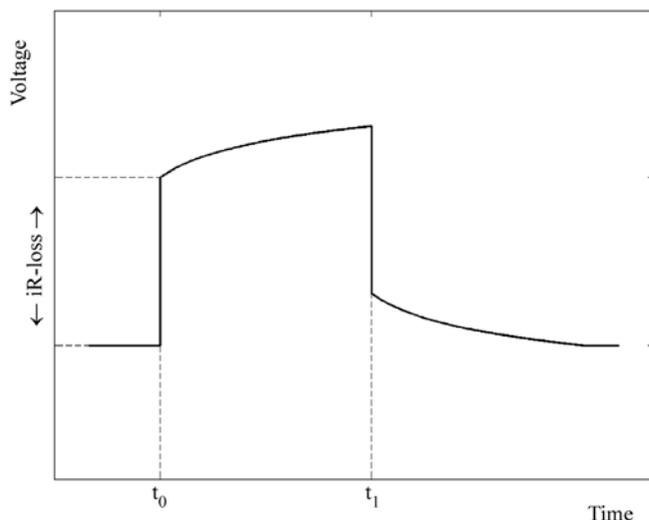
**Fig. 5:** Ideal voltage transient in a PEMFC after current interruption<sup>41</sup>.
