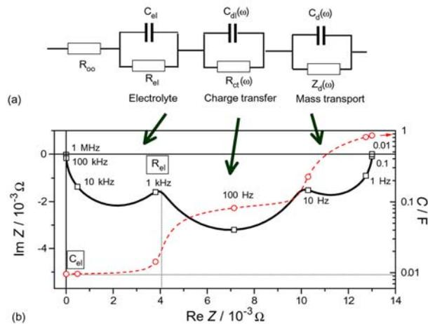
**Fig. 8:** (a) General equivalent circuit for a PEMFC (b) Schematic frequency response of impedance and capacitance<sup>49</sup>.
