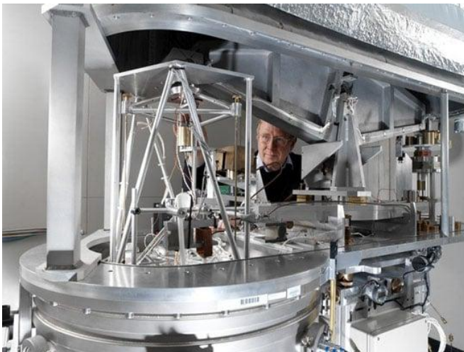
Figure 1: The NPL Mk. II Kibble Balance (now at NRC in Canada)
