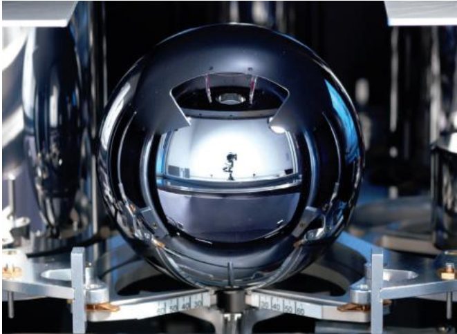
Figure 2: An XRCD (Avogadro) sphere on a mass comparator
