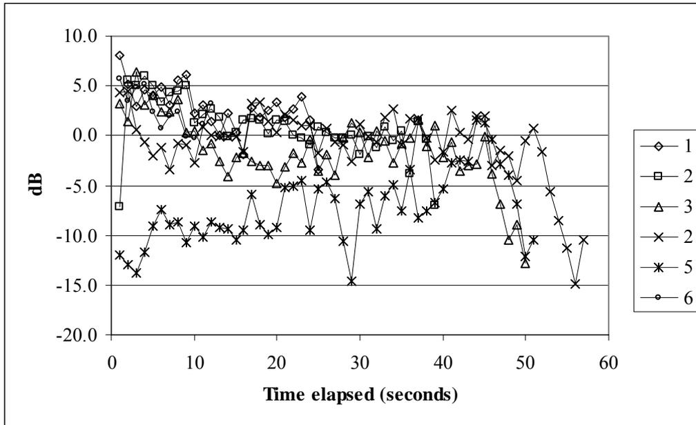
**Figure B.6b Sound Power Levels determined over 1-second periods for Shredder/chipper (Long timber samples)**
