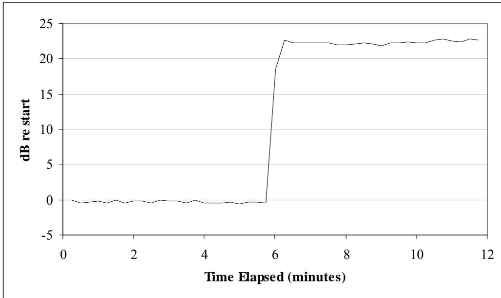
**Figure B.7b Sound Power Levels determined over 1-second periods for Chainsaw under load**
