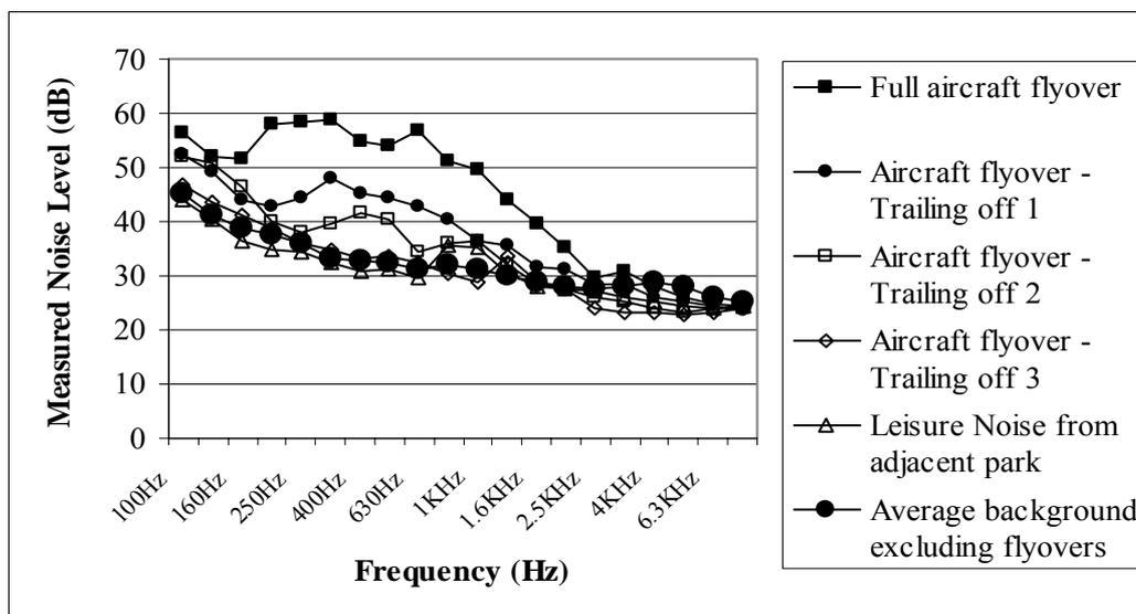
The corresponding A-weighted average background noise level excluding flyovers was determined to be around  $L_{Aeq}$  61 dB(A) at the test site during the daytime. It was considered likely that the machines selected for the study would generate significantly higher levels than prevailing background noise levels at the site, especially where aircraft flyovers and local traffic passby's could be avoided.
