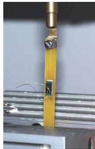
Figure 5. Specimen for pull testing.
