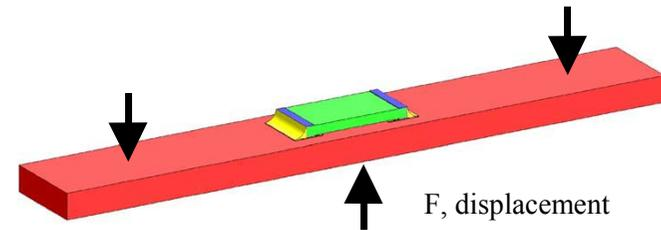
Figure 6. Schematic of the 3-point bend test.
