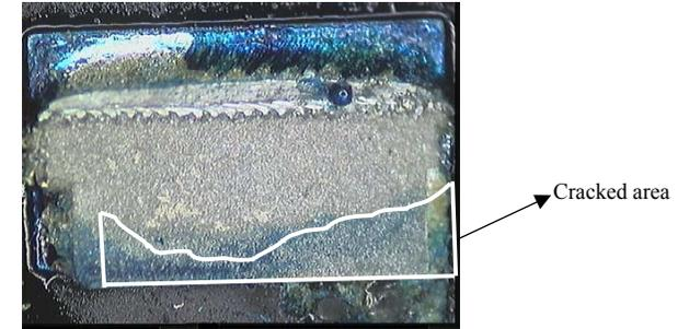
**Figure 3. Crack in a SnAgCu solder joint after thermal cycling**
