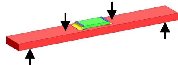
Figure 7. Test specimen with forces (arrows) acting in 4-point bend test.
