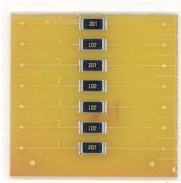
Figure 1. FR4 laminate with 2512-type resistors used in the crack assessment study.
