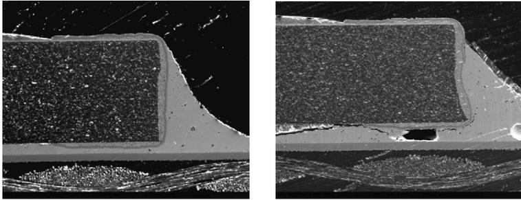
**Figure 2. Microsections of 2512-type resistor solder joints without a crack (300 cycles - left) and cracked (after 900 cycles - right). The images were taken in the SEM secondary electron mode**
