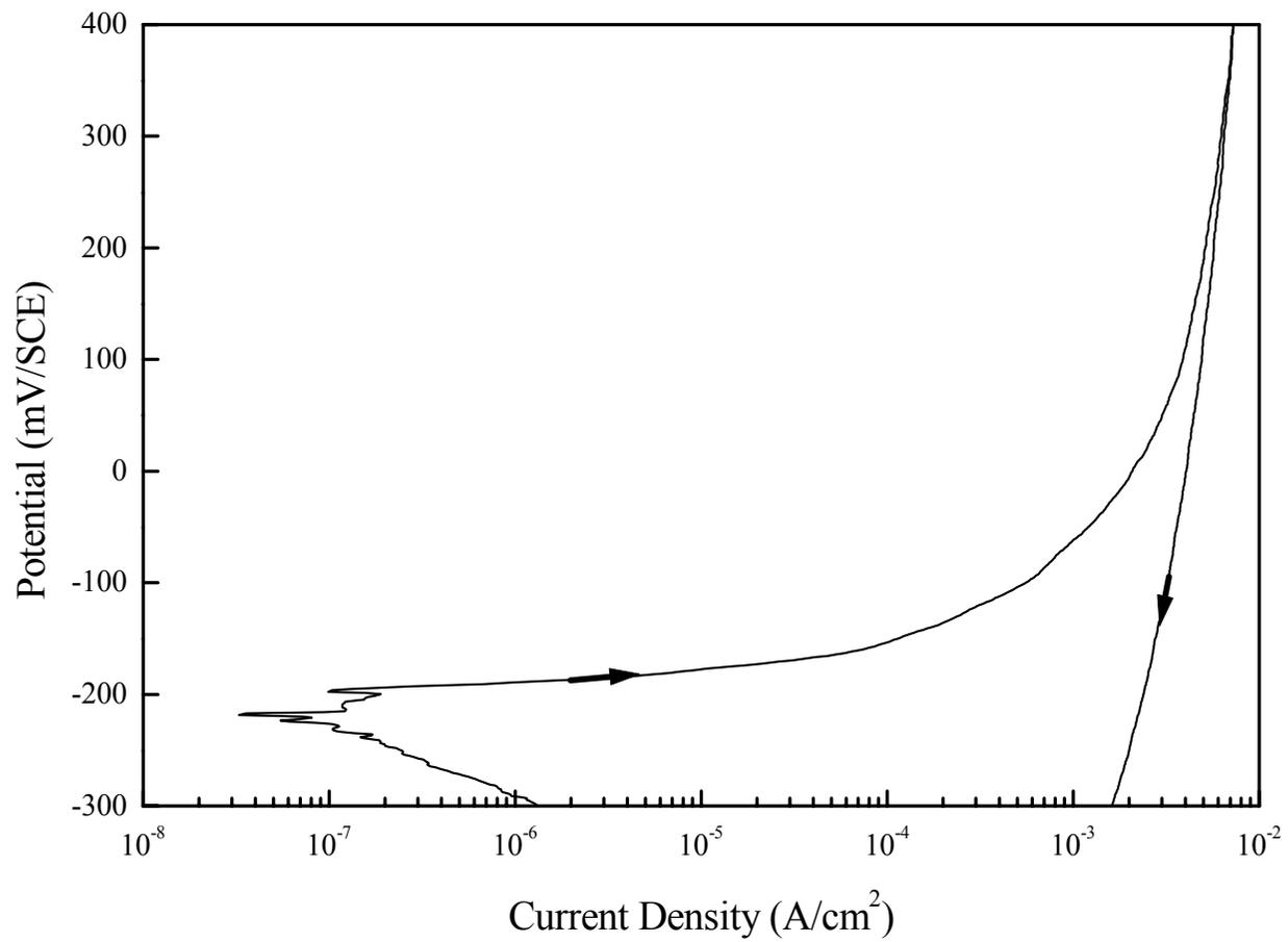
(b) 0.01 M Na<sub>2</sub>B<sub>4</sub>O<sub>7</sub> + 0.05 M NaCl solution
