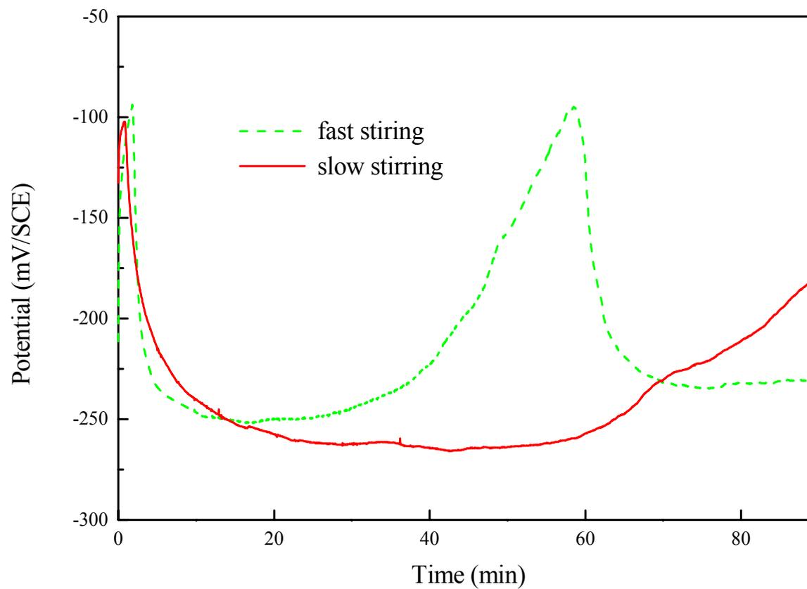
Fig. 4 Effect of the flow rate on the potential response of 3% NiCrMoV steel under galvanostatic polarisation ( $I = 10 \mu\text{A}$ ).
