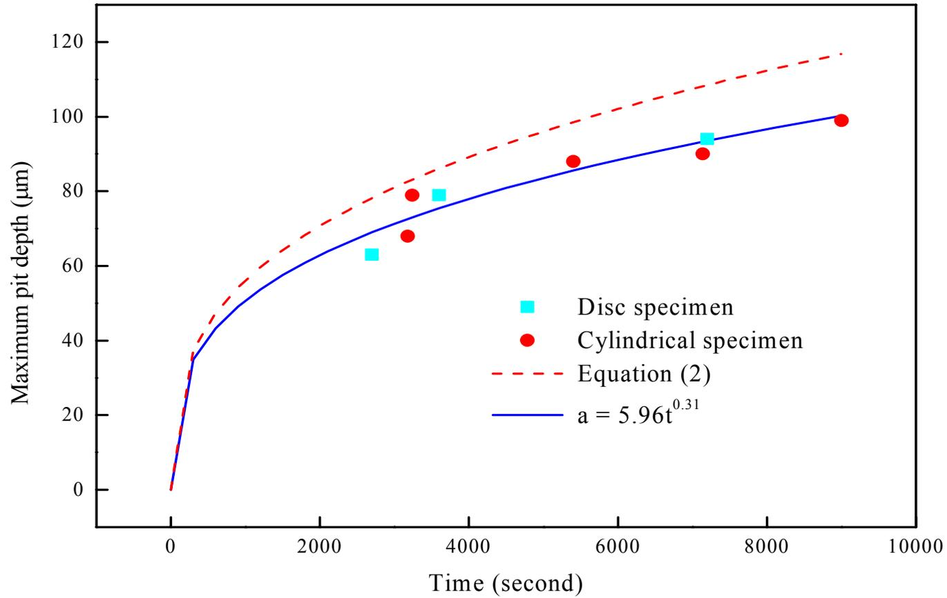
Fig. 5 Time dependence of maximum pit depth of 3% NiCrMnV steel in 0.02M  $\text{Na}_2\text{B}_4\text{O}_7$  + 0.01 M NaCl solution
