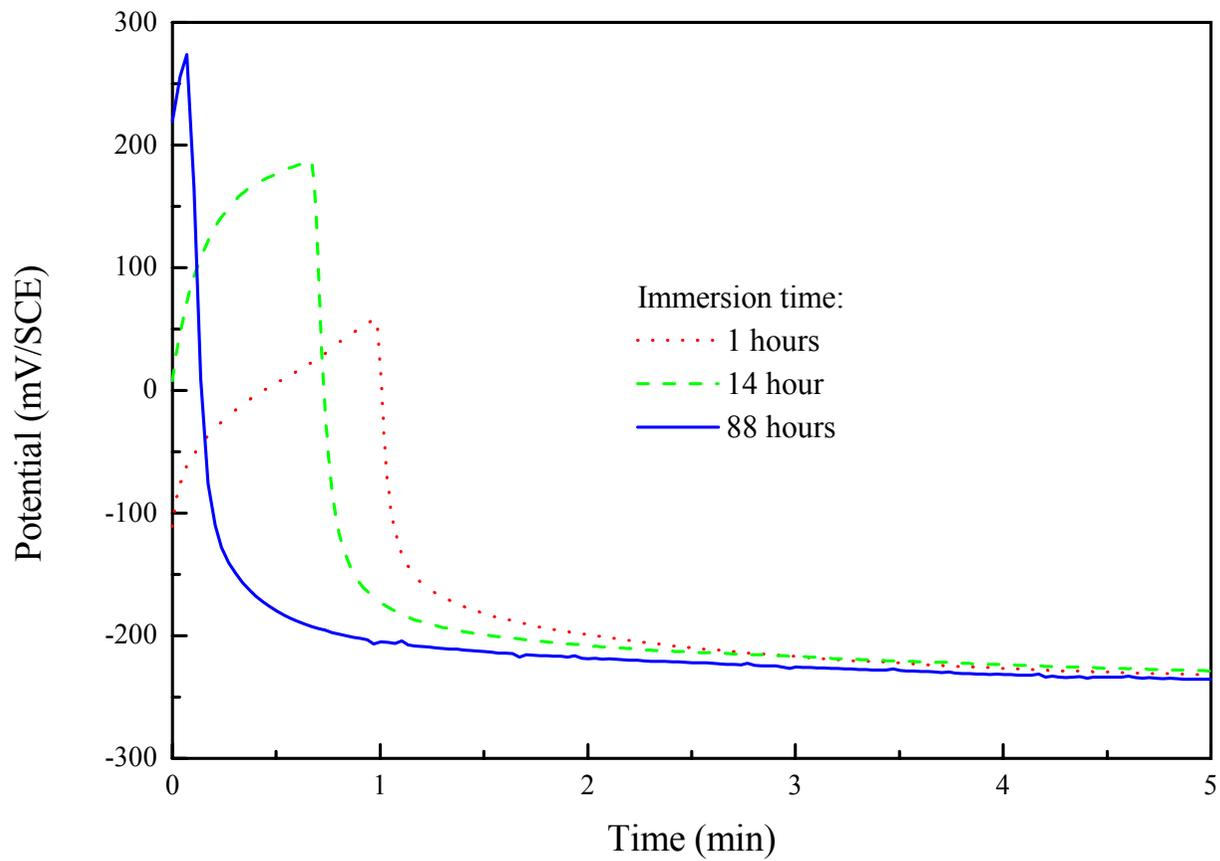
Fig. 3 Effect of immersion time on the pitting potential and the time to pit initiation under galvanostatic polarisation ( $I = 10 \mu\text{A}$ ).
