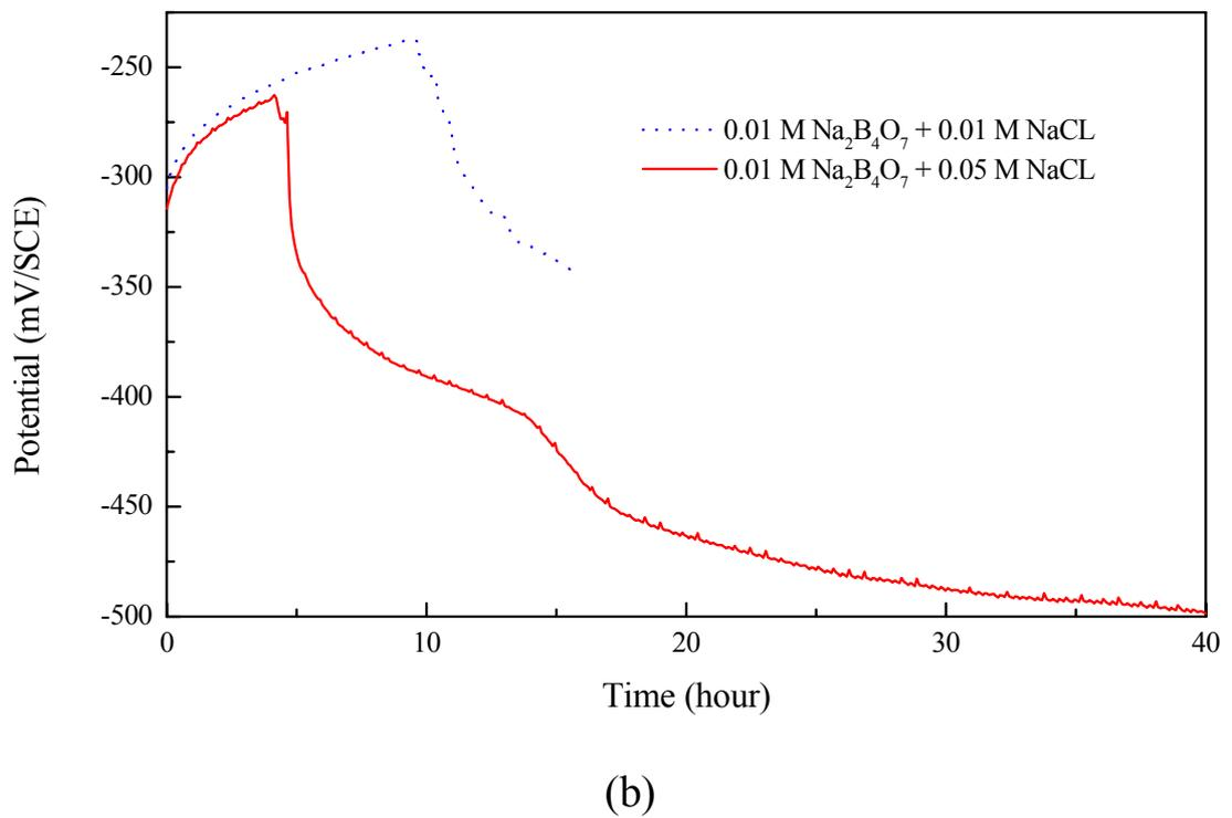
Fig.1 Effect of the ratio of  $\text{B}_4\text{O}_7^{2-}/\text{Cl}^-$  on the open circuit potential of 3% NiCrMoV steel as a function of time.
