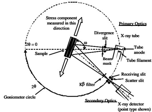
**Figure 2: Schematic of XRD system.**
