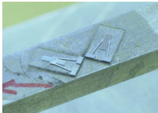
**Figure 5: Surface acoustic wave (SAW) devices mounted on torque beam.**
