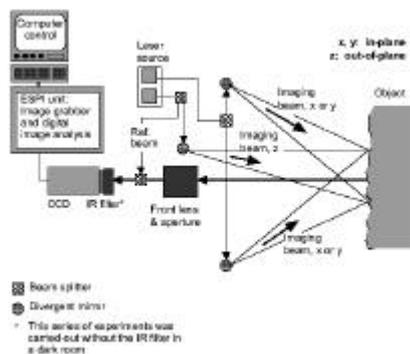
Figure 13: ESPI system layout [2].
