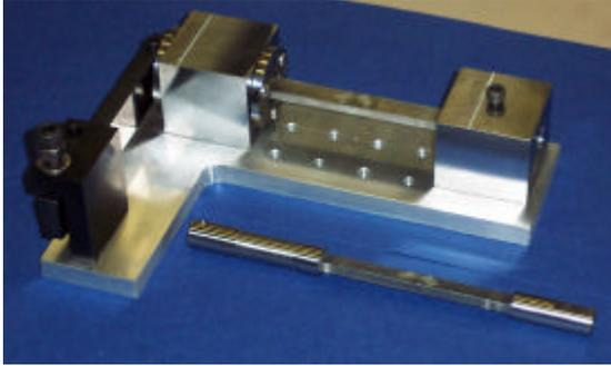
**Figure 6: Torque loading rig and specimen.**
