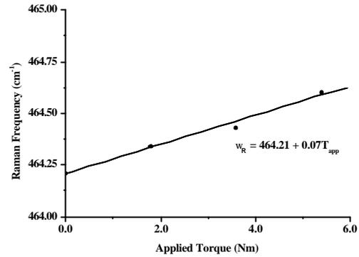
**Figure 12: Raman frequency shift (464 cm<sup>-1</sup>) at Position 6 on line C.**
