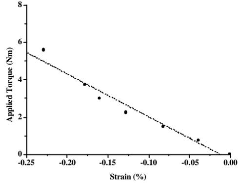
**Figure 7: XRD strain measurement versus applied torque.**
