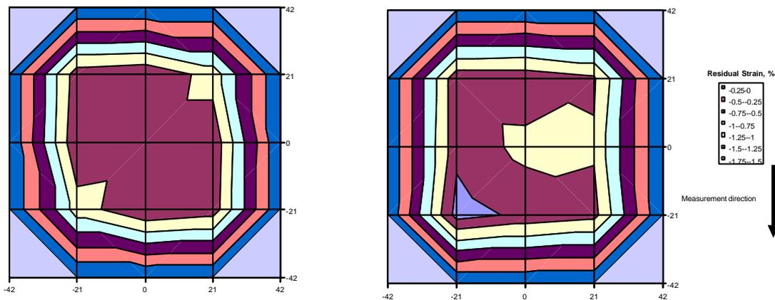
**Figure 4: Residual strain maps for “as-received” quartz wafers AA AE and AA AF.**
