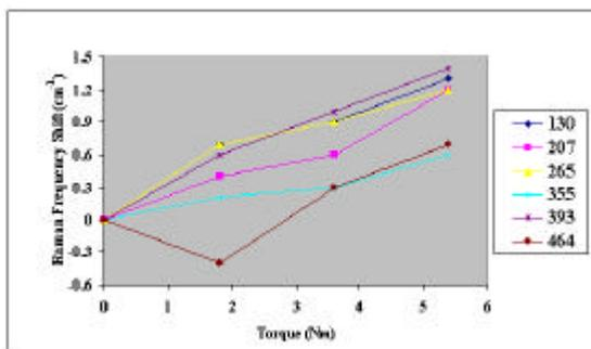
**Figure 11: Raman frequency shift as a function of applied torque.**
