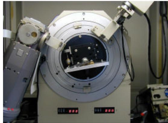
**Figure 1: Siemens D500 Diffractometer.**
