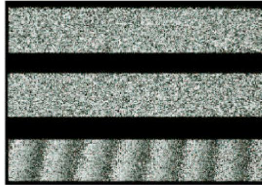
Figure 14: A typical speckle pattern resulting from out-of-plane deformation: undeformed (top); deformed (middle); and difference (bottom) [2].
