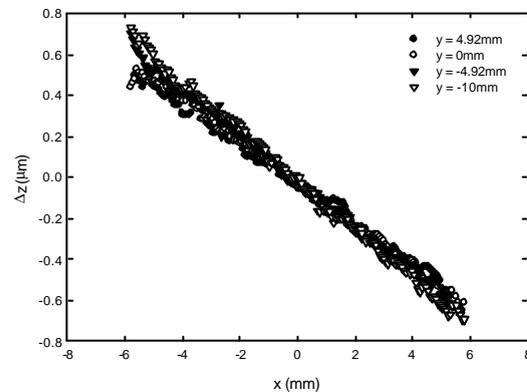
Figure 15: Out-of-plane deformation measurements on torque bar using ESPI.
