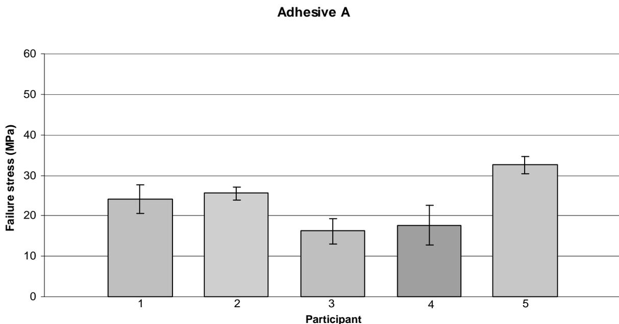
**Figure 4 Comparison of average failure stresses (with error bars) of specimens manufactured with Adhesive A from each participant**
