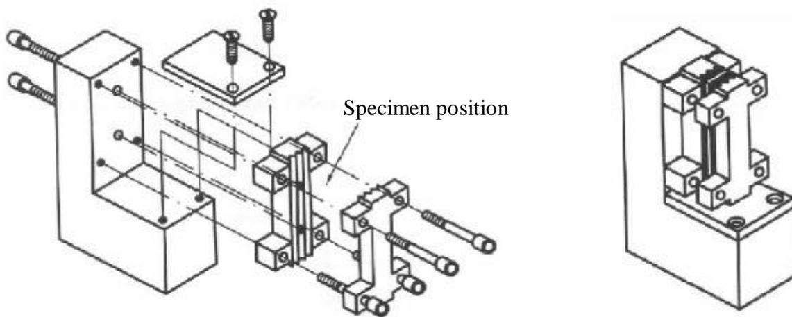
**Figure 2 Schematic of anti-buckling fixture**
