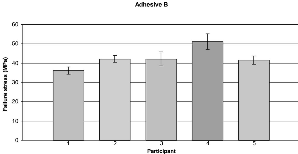
**Figure 5 Comparison of average failure stresses (with error bars) of specimens manufactured with Adhesive B from each participant**
