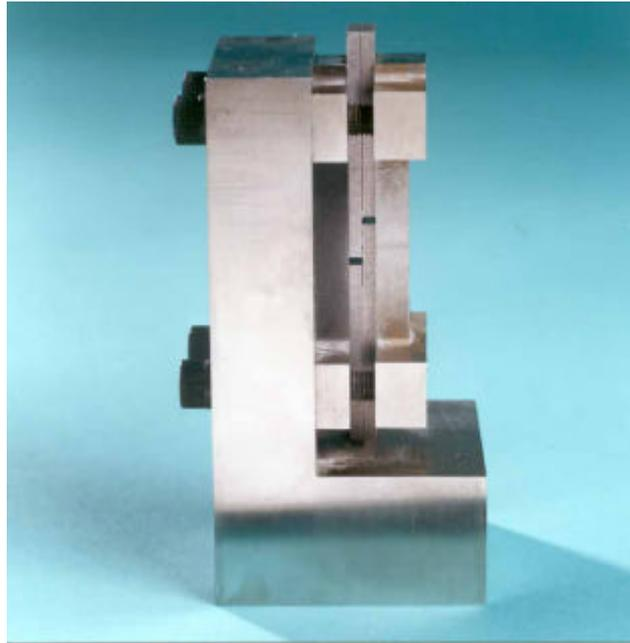
**Figure 3 Specimen in anti-buckling fixture**
