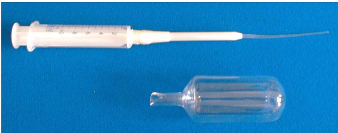
**Figure 3** The proboscis device (top) used to transferring acid from a quartz ampoule (below) during a reverse Tris titration.
