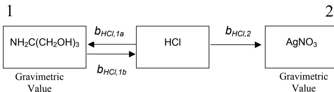
**Figure 1** The proposed titration regimes to determine the HCl molality.
