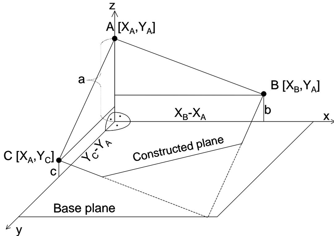
**Figure 4 Schematic for matrix levelling**
