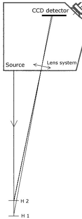
Figure 2: Schematic of laser triangulation sensor
