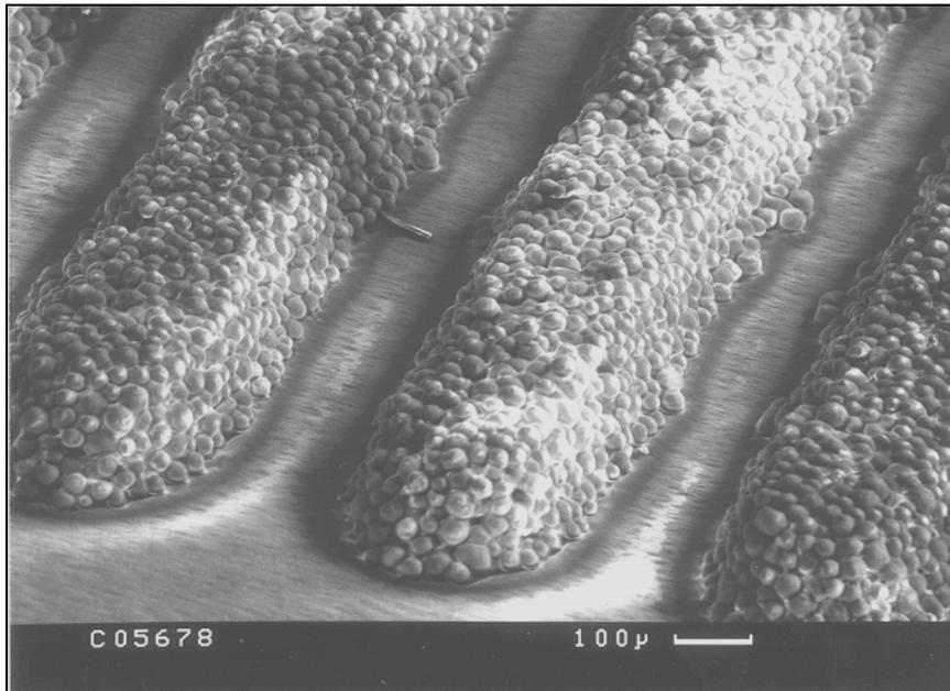
**Figure 1: Solder paste deposits stencil-printed on Cu substrate**
