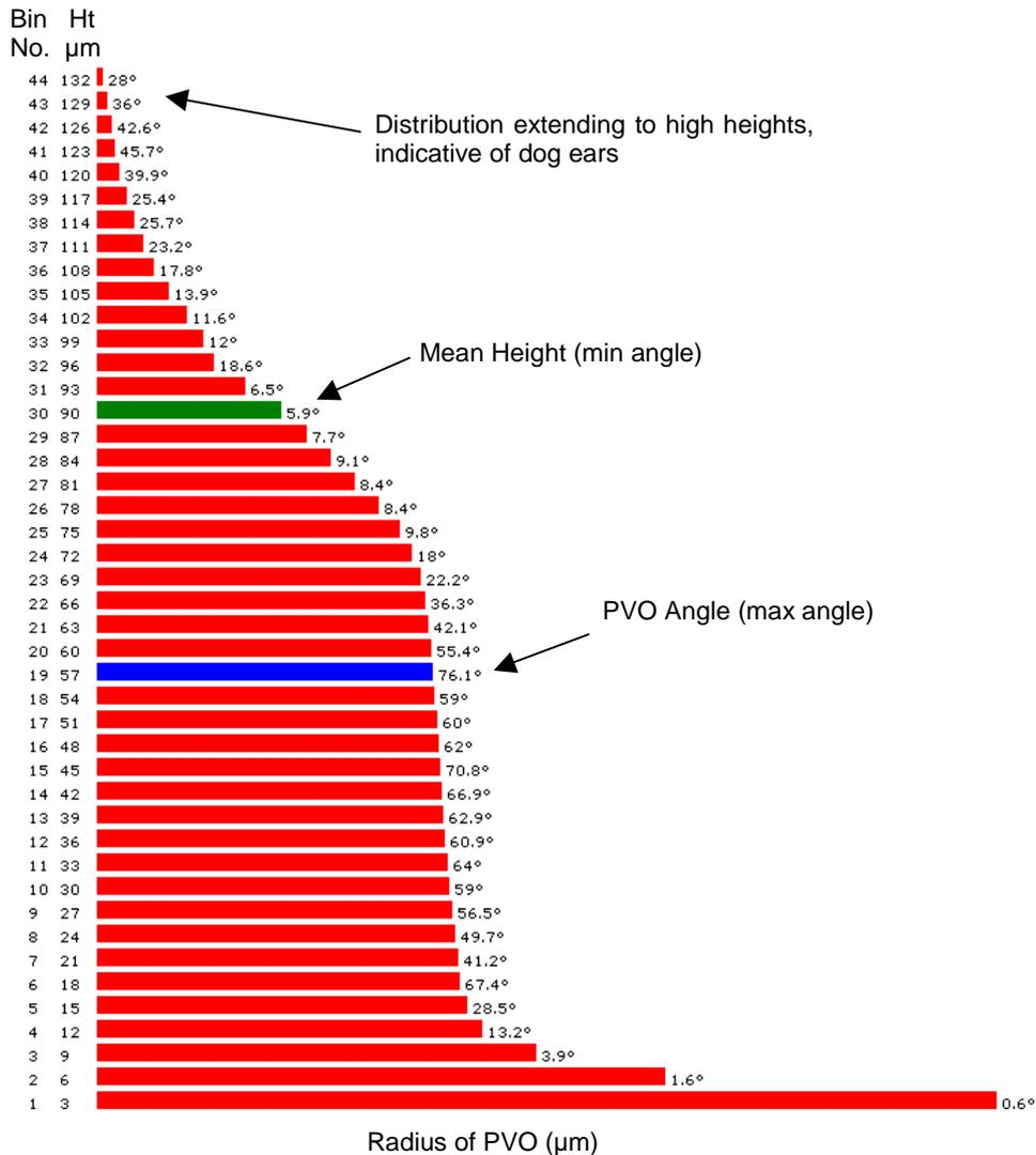
Figure 7: PVO profile derived from Figure 5 indication mean height =  $90\ \mu\text{m}$  and PVO corrected angle =  $76.1^\circ$  at  $57\ \mu\text{m}$
