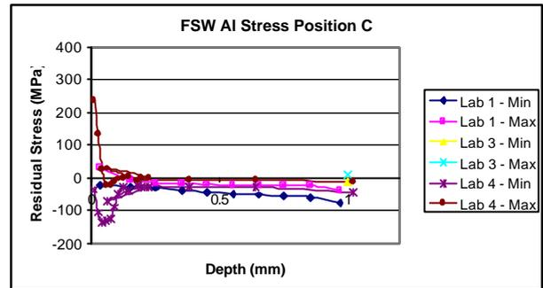
**Fig 12: Profile of residual stress vs depth for the Al friction stir weld (2<sup>nd</sup> iteration)**
