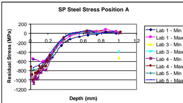
**Fig 11: Profile of residual stress vs depth for the shot-peened steel (2<sup>nd</sup> iteration)**
