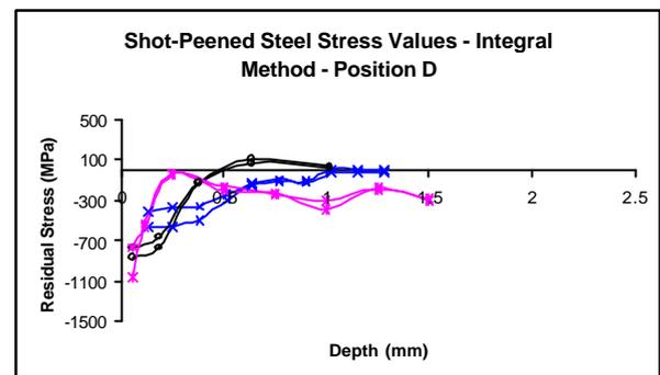
Fig 9: Profile of residual stress vs depth for the shot-peened steel for laboratories that used the integral method.
