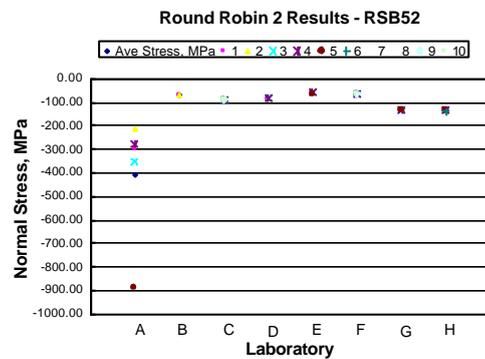
Fig 5: XRD Residual Stress measurements conducted on the 6082 alloy, showing the scatter from repeat measurements and the average value for each laboratory
