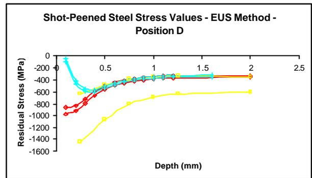
Fig 8: Profile of residual stress vs depth for the shot-peened steel for laboratories that used the EUS method.
