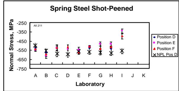
**Fig 2: XRD results on the spring steel in the SHOT PEENED condition (1<sup>st</sup> iteration)**
