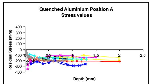
Fig 10: Profile of residual stress vs depth for the heat-treated aluminium
