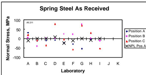
**Fig 1: XRD results on the spring steel in the AS RECEIVED condition (1<sup>st</sup> iteration)**
