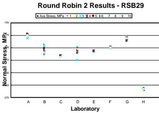
Fig 4: XRD Residual Stress measurements conducted on the same 7010 Al specimen, showing the scatter from repeat measurements and the average value for each Lab
