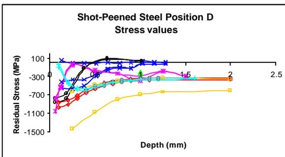
Fig 7: Profile of residual stress vs depth for the shot-peened steel
