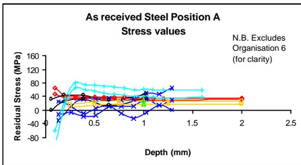
Fig 6: Profile of residual stress vs depth for the as-received steel.
