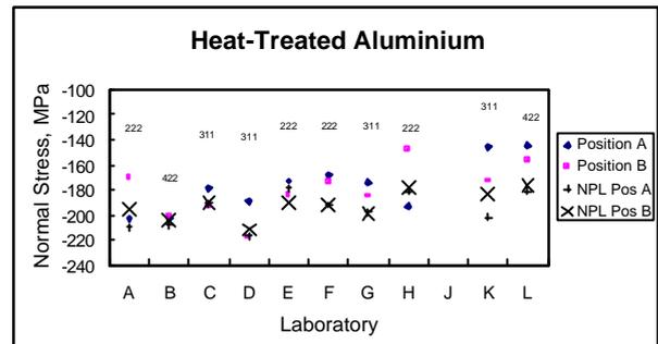
**Fig 3: XRD results on the Quenched Aluminium specimen (1<sup>st</sup> iteration)**
