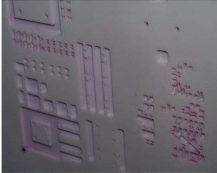
Figure 4: Underside of relief stencil, showing cut outs
