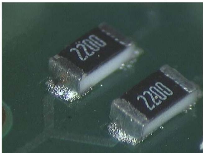
Figure 33: Reflowed solder joint on R0603s on side A
