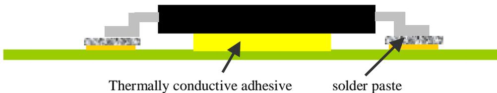
Figure 6: Schematic of relief printing process for thermally conductive adhesive
