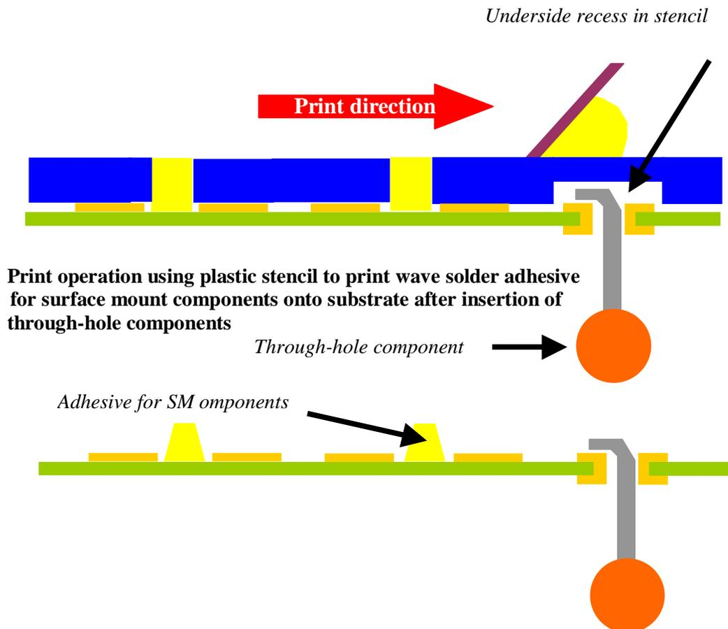
Figure 7: Schematic of printing of wave solder adhesive for SM
