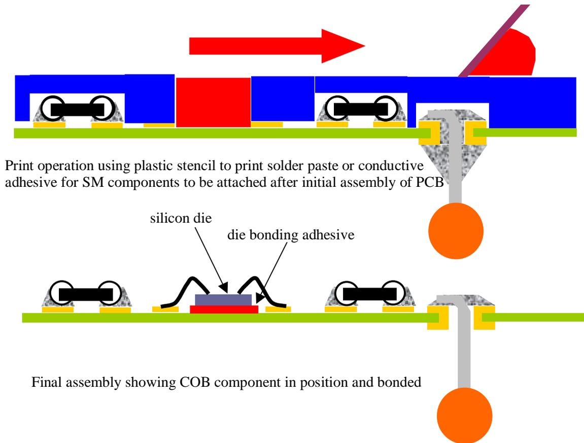
Figure 11: Schematic of printing of die-bonding adhesive for assembly of COB
