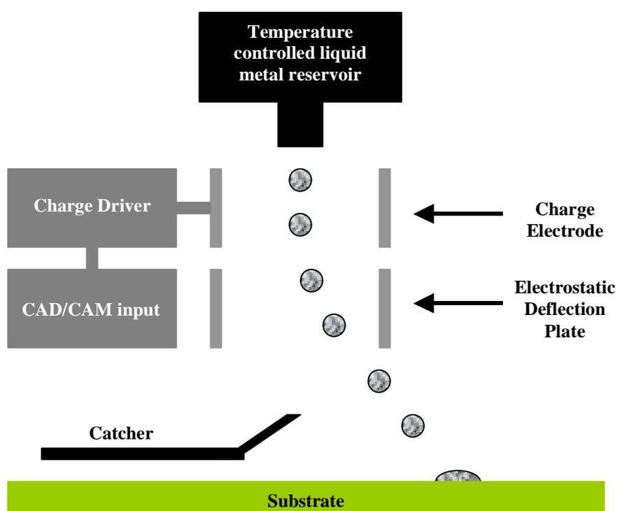
Figure 1: Schematic of continuous deposition solder jetting
