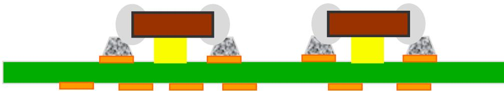
Stage 4: Optional curing of adhesive (heat and/or UV), inversion of assembly and printing of solder paste with metal stencil
