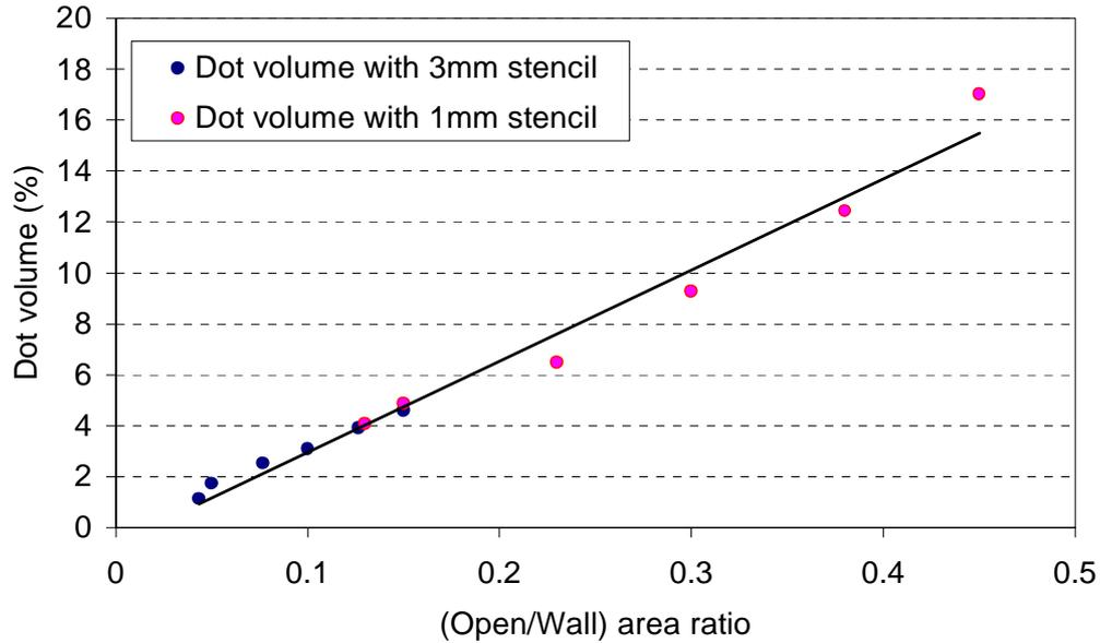
Figure 17: Dot volume with (open/wall) area ratio for 1.0 and 3.0mm stencils
