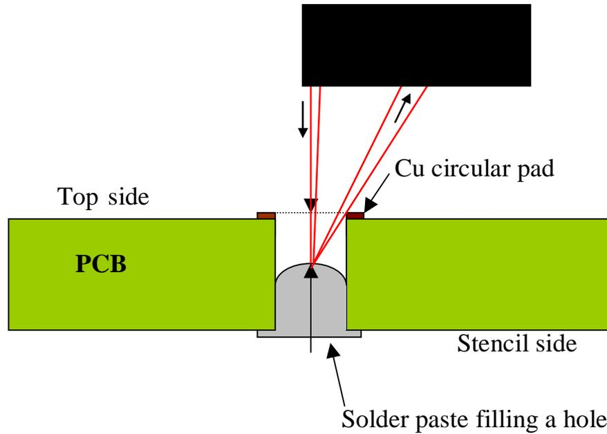
**Figure 20 : Schematic of height measurement of solder paste filling a PCB hole**
