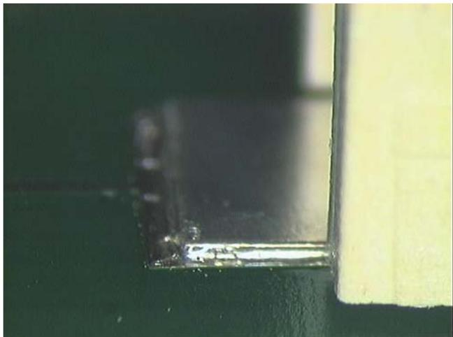
Figure 31: Reflowed solder joint on battery connector on side A
