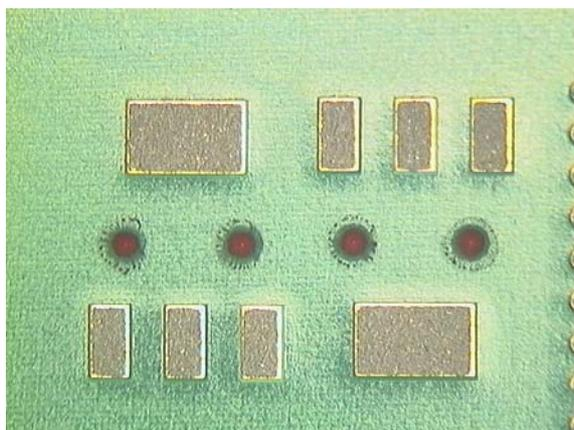
Figure 25: Paste and adhesive for SOT223 component
