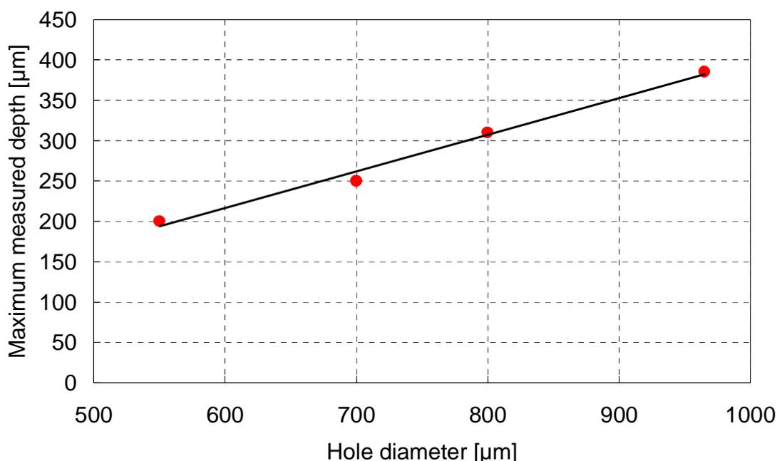
Figure 22 : Maximum available height measured from top of PCB to solder paste surface
