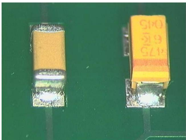
Figure 34: Reflowed solder joints on C1206 and tantalum on side A
