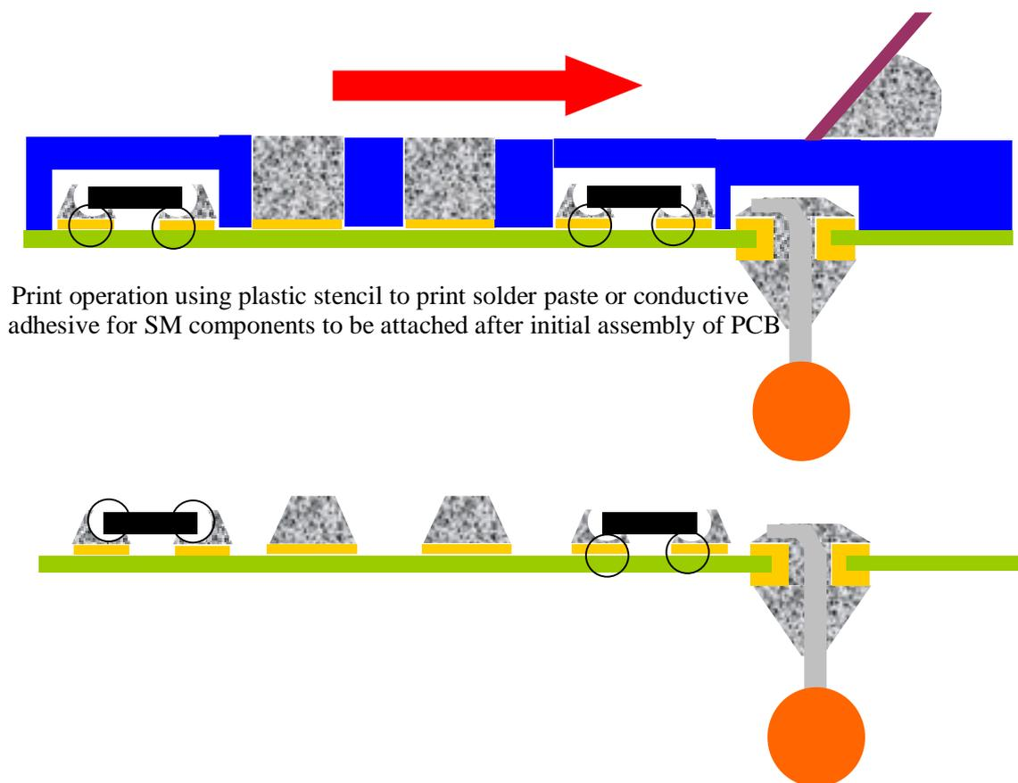
Print operation using plastic stencil to print solder paste or conductive adhesive for SM components to be attached after initial assembly of PCB
