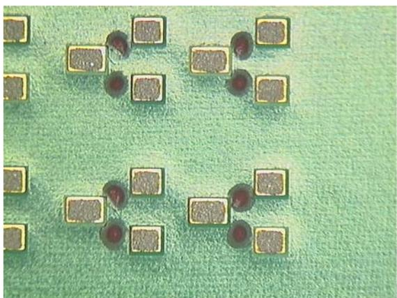
Figure 29: Paste and adhesive for SOT323 component
