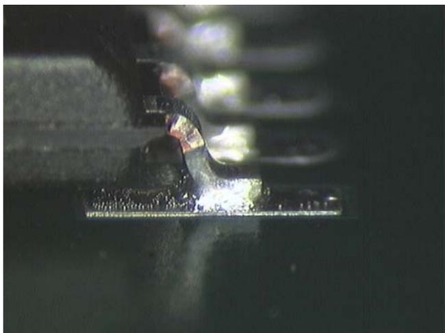
Figure 32: Reflowed solder joint on SOIC on side A
