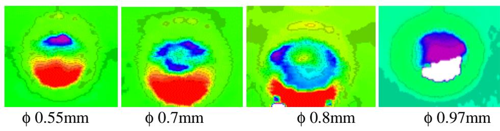
Figure 21 : Example of contour maps of scanned holes in a PCB filled with solder paste (as a function of hole diameter)
