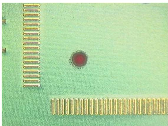
Figure 28: Paste and adhesive for QFP component
