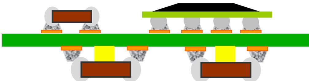
Figure 24: Schematic of SDSRS assembly using relief printing
