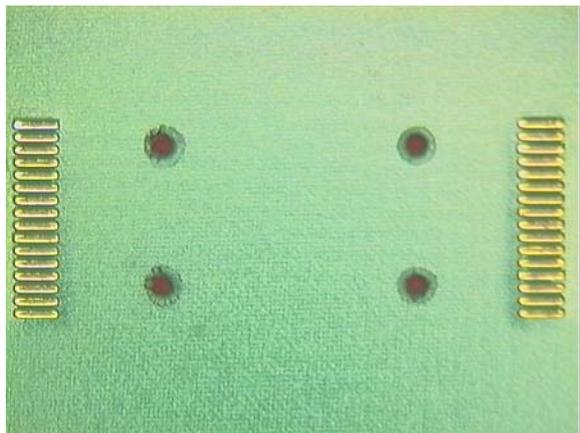
Figure 27 : Paste and adhesive for TSOP component
