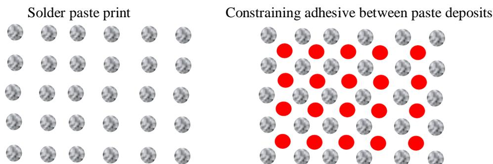
Figure 12: Plan view of relief printed underfill constraining columns
