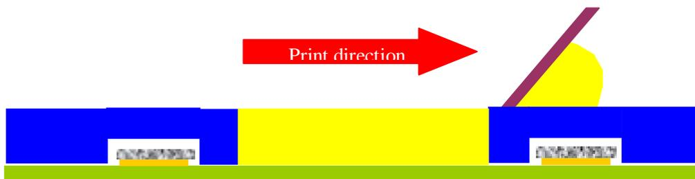
Print operation using plastic stencil and thermally conductive adhesive with underside recesses fitting over previously printed deposits of solder paste
