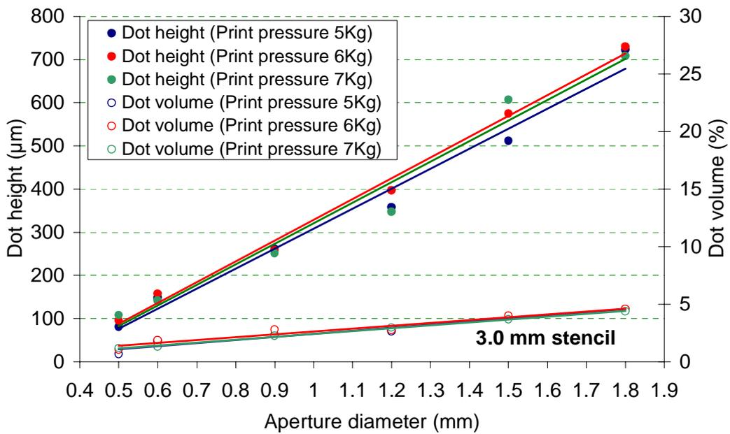
Figure 16: Dot height and volume with squeegee pressure for 1.0 and 3.0mm stencils
