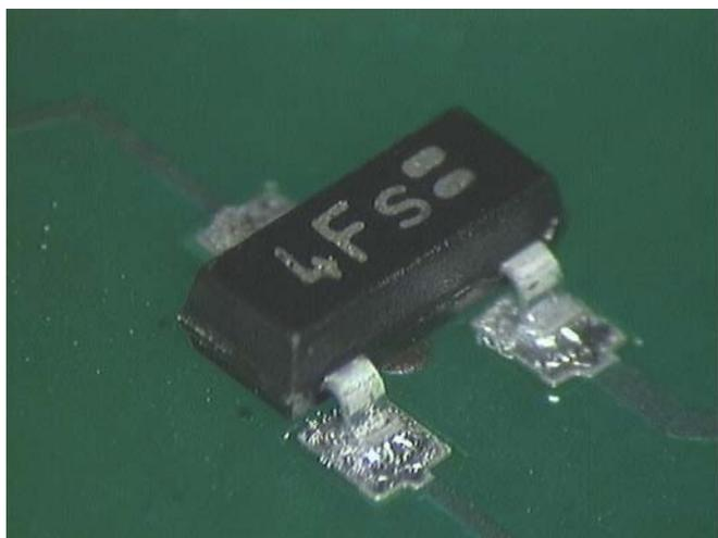
Figure 35: Reflowed solder joint on SOT23 on side A
