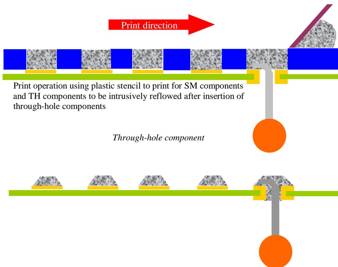
Figure 8: Schematic of printing for extrusive reflow
