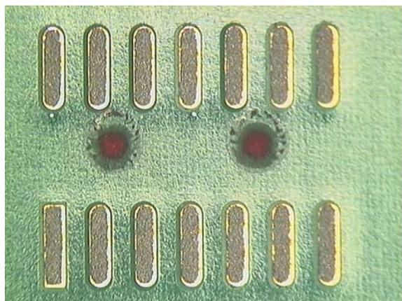
Figure 26: Paste and adhesive for SOIC14 component
