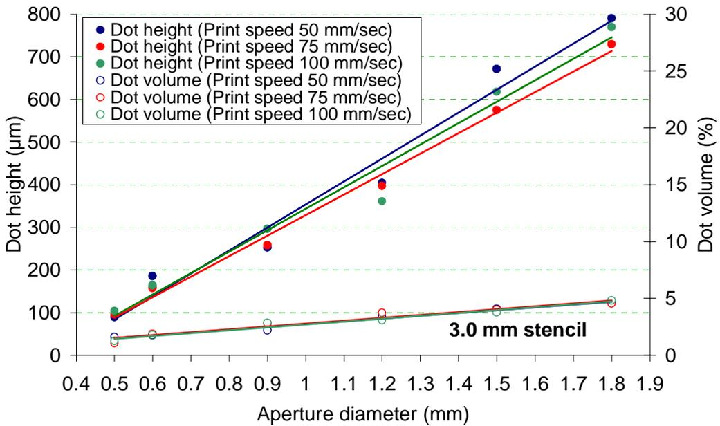
Figure 15: Dot height and volume with print speed for 1.0 and 3.0mm stencils
