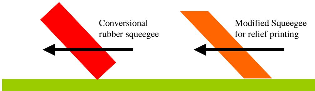
Figure 13: Comparison of conventional squeegee and modified Squeegee for relief printing
