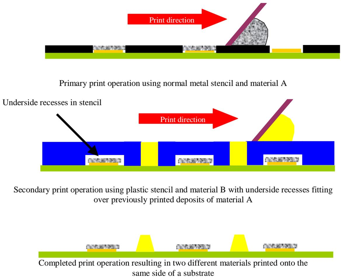
Figure 5: Schematic of relief printing process
