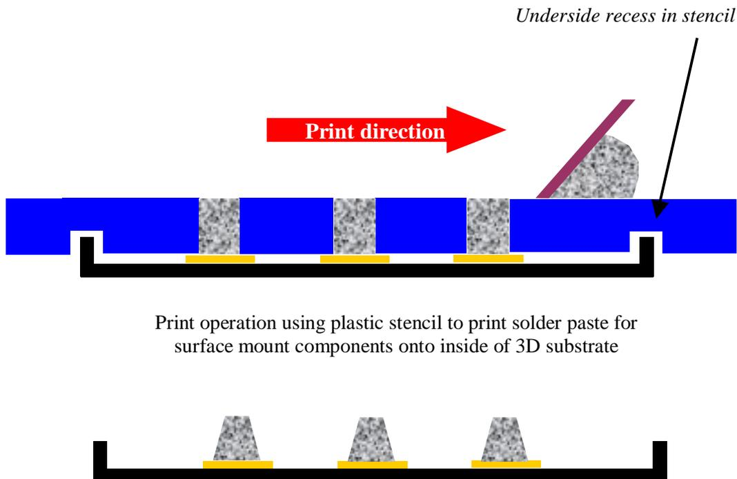
Figure 9: Schematic of printing on 3D substrates
