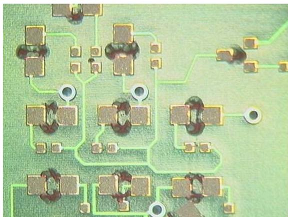
Figure 30: Paste and adhesive for chip LED, SOT23 and R0603 components
