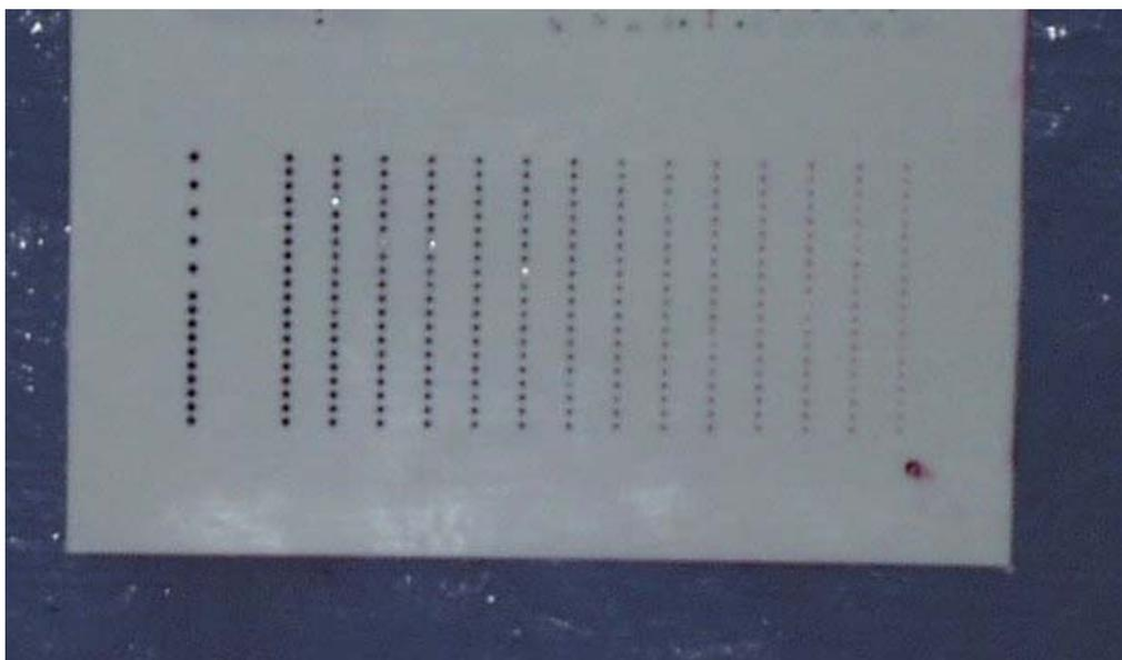
Figure 2: Photo of typical pump print stencil
