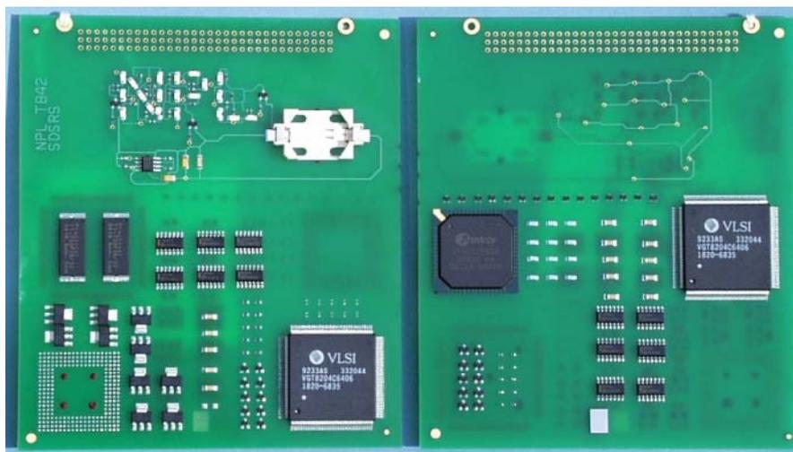
Figure 23: SDSRS Test Assembly (NPL Test Board TB42)
