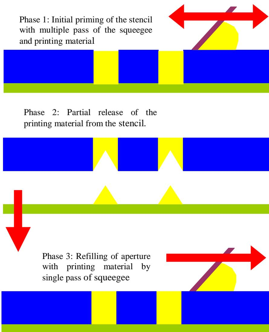
Figure 3: Schematic of Pump Printing Operation
