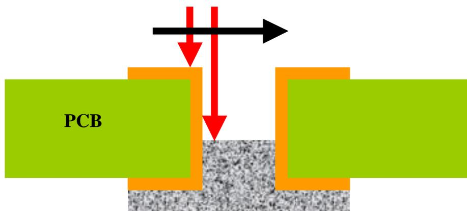
**Figure 19 : Schematic showing rapid height changes experienced with intrusive reflow measurement**
