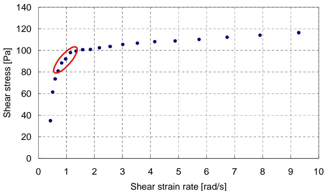
**Figure 2: Flow curve, red ellipse indicates working region of shear strain rate and related stress for a solder paste extract**
