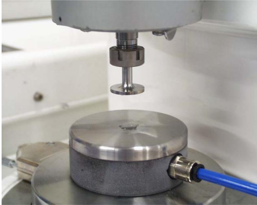
**Figure 3: Parallel plate geometry with a liquid solder paste extract as a measurement sample**
