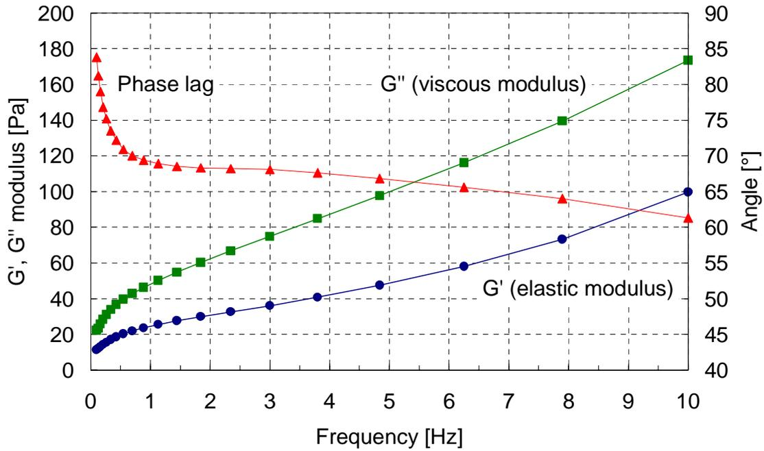
**Figure 5: Oscillation test run at 90 Pa shear stress of harmonic amplitude for determination of frequency response of solder paste extract**
