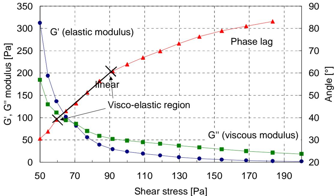
**Figure 4 Oscillation test run at 1 Hz for determination of visco-elastic region**
