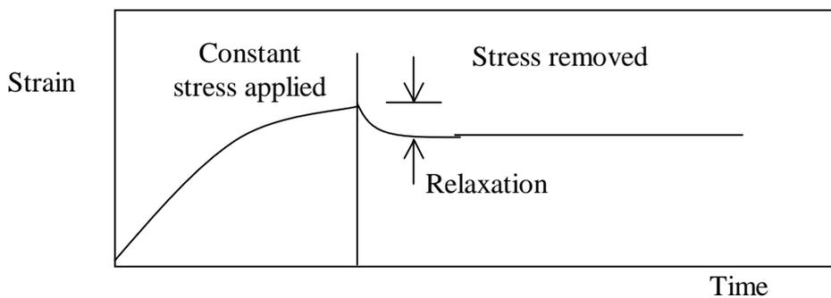
**Figure 6: Schematic of creep response of print media**
