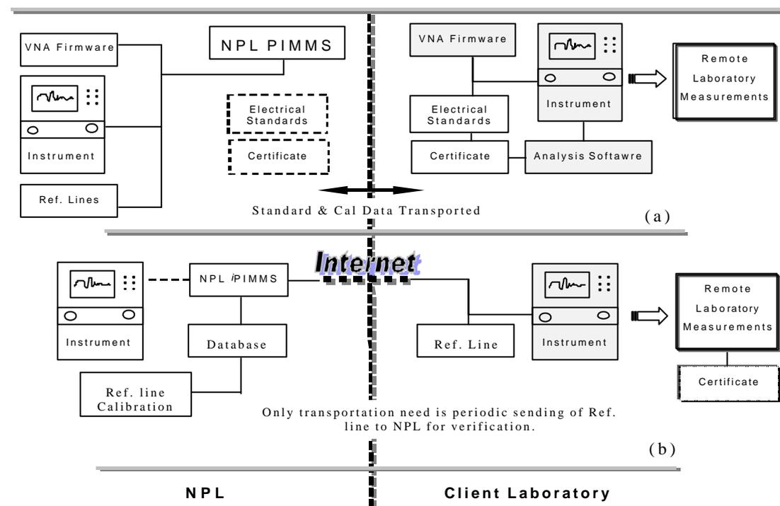
Figure 1: (a) basic components of NPL VNA calibration system: artefacts, instrument and control firmware, producing a certificate for the remote laboratory's artefacts; (b) the Internet system removes the need for travelling verification artefacts by allowing direct access to PIMMS.
