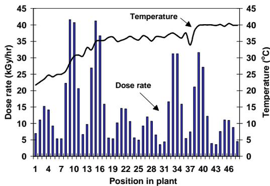
**Fig. 3** Dose rate and temperature profiles measured at a MDS Nordion JS 7500 irradiator. Sensors approximately in centre of tote.
