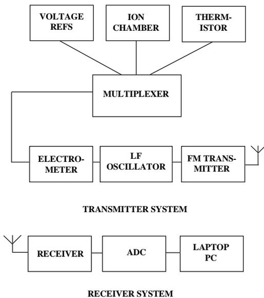
**Fig. 1** Block diagram of Real Time Dosimeter System.
