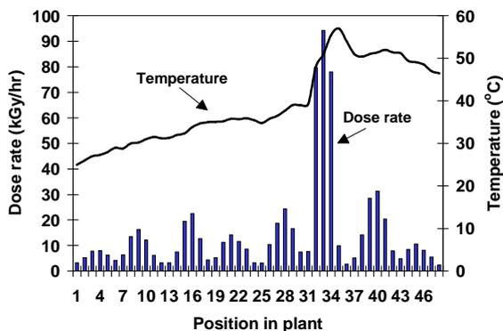
**Fig. 4** Dose rate and temperature profiles measured at a MDS Nordion JS 7500 irradiator. Sensors in bottom corner of tote.
