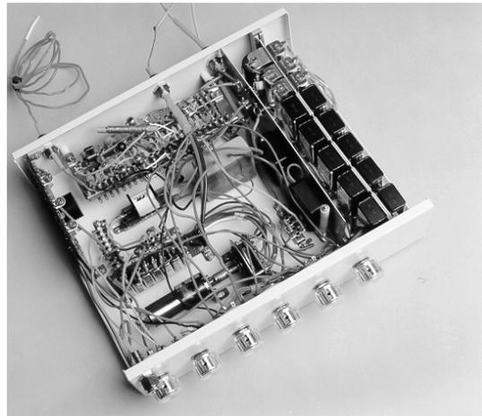
**Fig. 2** Photograph of transmitter unit with cover removed.
