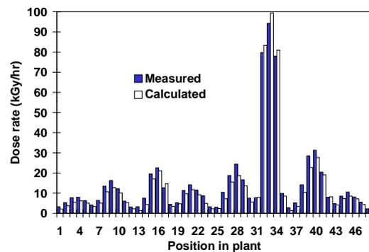
**Fig. 5** Comparison of measured and calculated dose rate profiles in a MDS Nordion JS 7500 irradiator. Sensor in bottom corner of tote.
