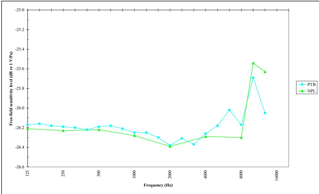
Figure 5. Uncorrected  $L_{MF}$  of 4145 2071917 measured using an LS2P reference microphone
