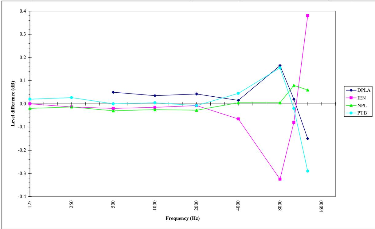
Figure 9. Deviation of corrected  $L_{Mf}$  from grand mean (LS2P reference microphone)
