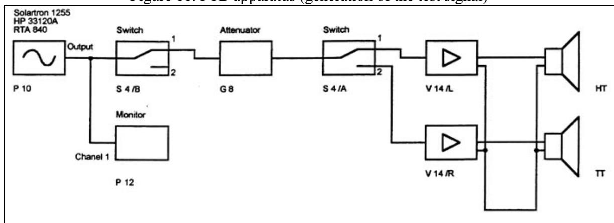
Figure 12. PTB apparatus (measurement of microphone output by insert voltage technique)
