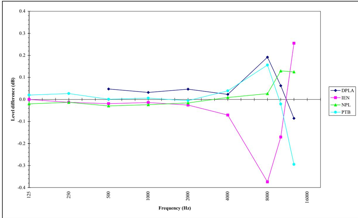
Figure 7. Deviation of uncorrected  $L_{Mf}$  from grand mean (LS2P reference microphone)
