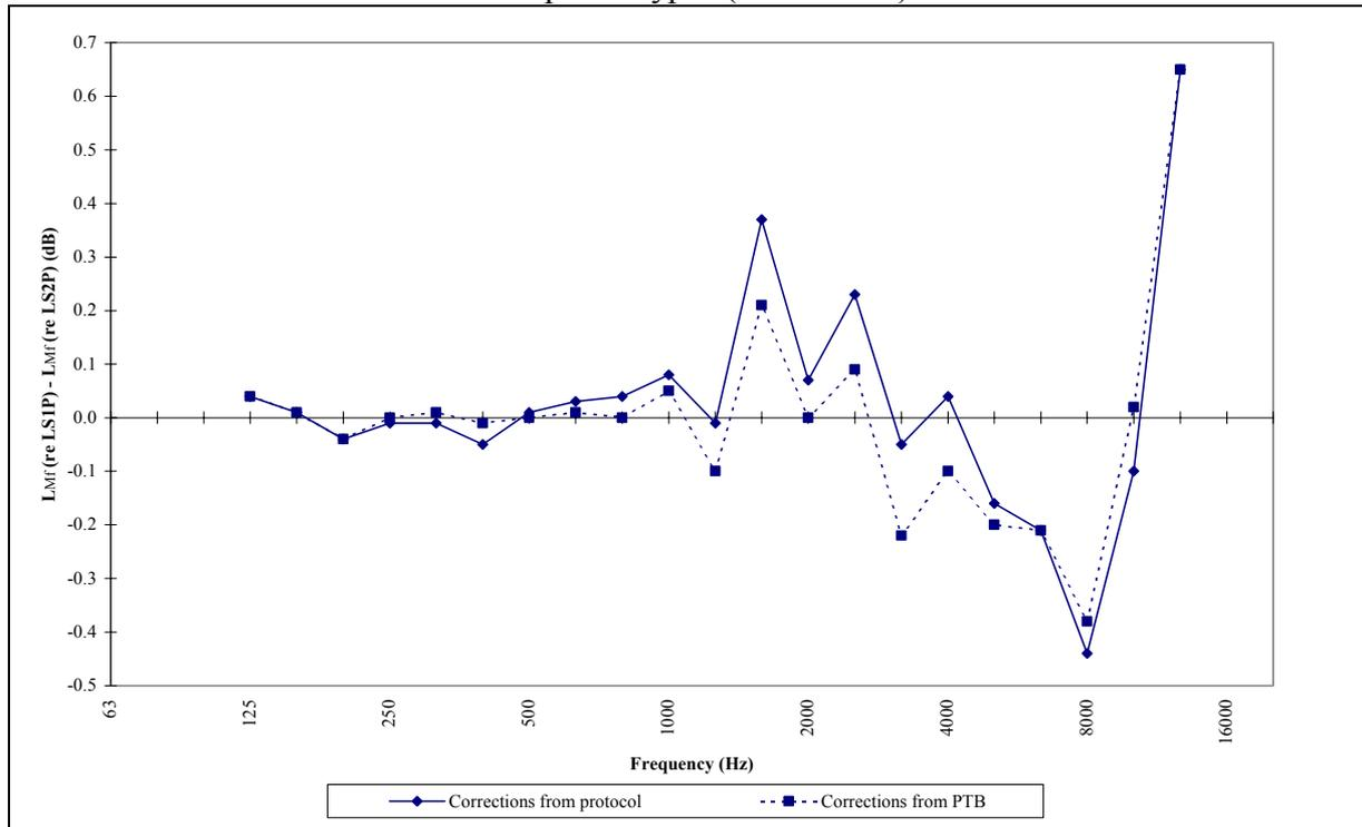
Figure 16. Difference between  $L_{MF}$  of 4145 2071918 measured with different reference microphone types (NPL results)
