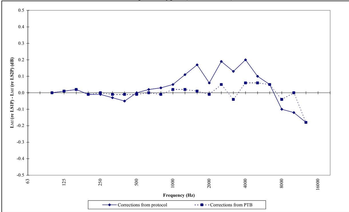
Figure 14. Difference between  $L_{Mf}$  of 4145 2071917 measured with different reference microphone types (NPL results)
