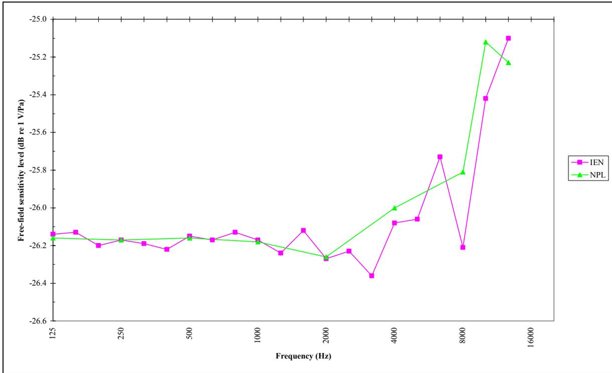
Figure 3. Uncorrected  $L_{MF}$  of 4145 2071918 measured using an LS2P reference microphone
