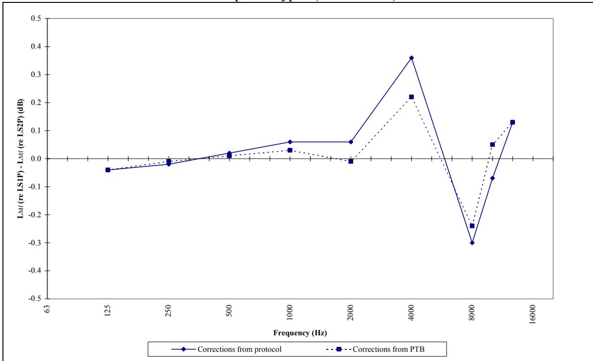
Figure 15. Difference between  $L_{MF}$  of 4145 2071918 measured with different reference microphone types (IEN results)
