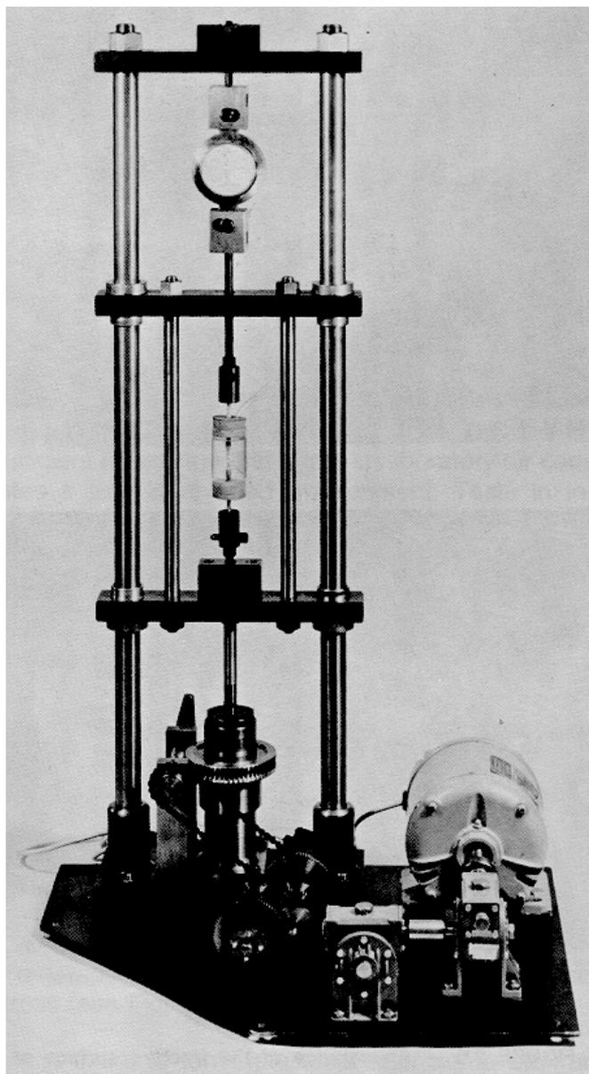
**Figure 7 Typical apparatus used for slow strain rate testing of plastics (courtesy of University of Newcastle upon Tyne, Newcastle upon Tyne, UK).**
