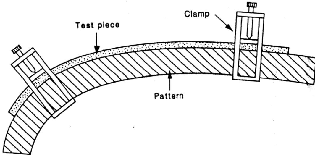
Figure 5 Elliptical jig with a former of variable radius used to develop variable strains along the length of the specimen
