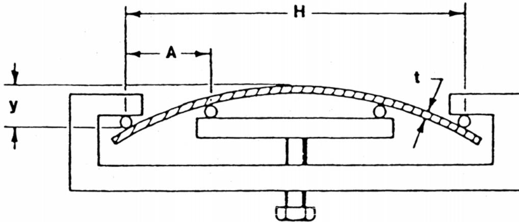
**Figure 3** Schematic illustration of 4 point bend constant strain apparatus, where  $H$  distances between the outer supports,  $A$  distance between inner and outer supports,  $t$  thickness of specimen,  $y$  deflection of specimen.
