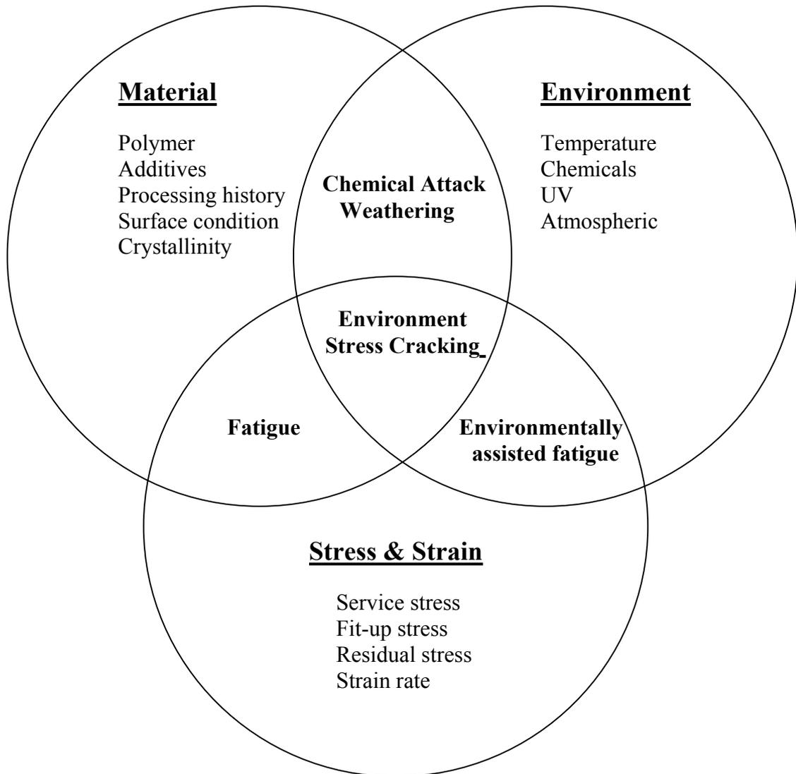
**Figure 1 Interaction of material properties, environment and stress/strain on environment stress cracking.**
