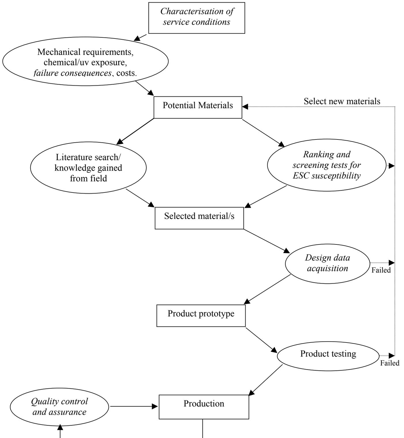
**Figure 2** Flow chart illustrating a typical test strategy employed in materials selection.
