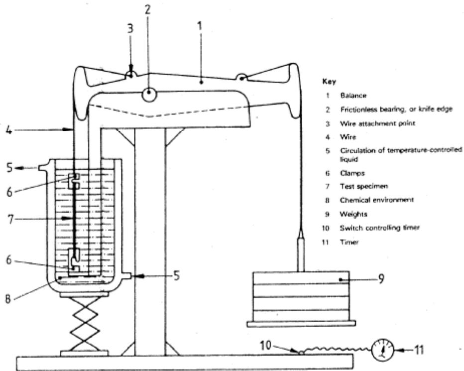
Figure 6 Illustration of typical apparatus used for a constant load test.
